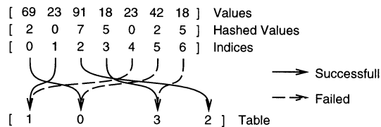
FIGURE 47.6 Each key attempts to write its index into a hash table entry.
