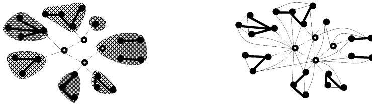
FIGURE 34.2 The figure on the left shows the r trees T_1, \dots, T_r obtained from T by deleting the nodes of S . Each tree is indicated by a shaded region. The figure on the right shows that no edges of the input graph G connect different trees T_i .
