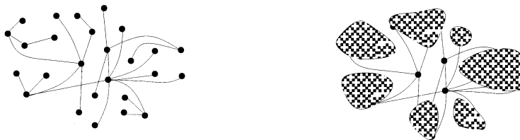
FIGURE 34.3 The figure on the left shows an arbitrary spanning tree T^* for the same input graph G . The figure on the right has r shaded regions, one for each subset V_i of nodes corresponding to a tree T_i in Fig.34.2. The proof of the algorithm's performance guarantee is based on the observation that at least r + |S| - 1 edges are needed to connect up the V_i 's and the nodes in S .
