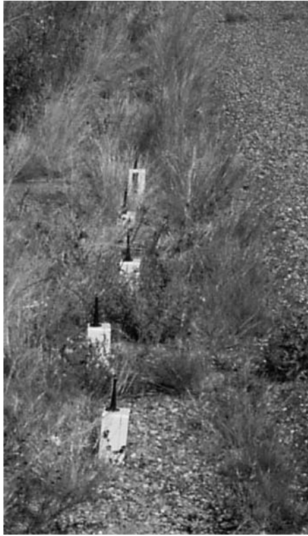
Figure 2.5. Stage one Mica2 vehicle detection network.
