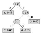
With this tree, the codes would be A=0, C=111, G=110, T=10. They would still be prefix-free, and the number of bits in each code would be the same as before. That's because the number of bits in the code for a character is the same as the *depth* of the character's leaf: the number of edges in the path from the root down to the leaf. Life is simpler, however, if we always label edges to left children by 0 and edges to right children by 1.
