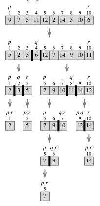
The bottommost value in each array position gives the final element stored there. When you read the array from left to right, looking at the bottommost value in each position, you see that the array is indeed sorted.
