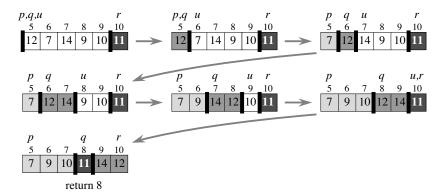
As when we partitioned books, we compare each element with the pivot once and perform at most one swap for each element that we compare with the pivot. Since each comparison takes constant time and each swap takes constant time, the total time for PARTITION on an n-element subarray is  $\Theta(n)$ .
