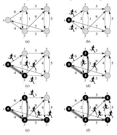
It shows a directed graph with source vertex s and weights next to the edges. Think of the weight of an edge as the number of minutes it would take a runner to traverse the edge.
