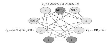
It's easy enough to see that this reduction can be performed in polynomial time. If the 3-CNF formula has k clauses, then it has 3k literals, and so the graph has 3k vertices. At most, each vertex has an edge to all the other 3k-1 vertices, and so the number of edges is at most 3k(3k-1), which equals  $9k^2-3k$ . The size of the graph constructed is polynomial in the size of the 3-CNF input, and it's easy to determine which edges go into the graph.
