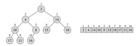
A *binary heap* is a binary tree with three additional properties. First, the tree is completely filled on all levels, except possibly the lowest, which is filled from the left up to a point. Second, each node contains a key, shown inside each node in the figure. Third, the keys obey the *heap property*: the key of each node is less than or equal to the keys of its children. The binary tree in the figure is also a binary heap.
