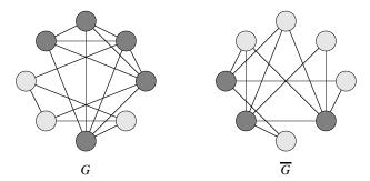
Note that every edge in  $\overline{G}$  is incident on at least one heavily shaded vertex.
