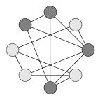
Verifying a certificate is easy. The certificate is the k vertices claimed to form a clique, and we just have to check that each of the k vertices has an edge to the other k-1. This check is easily performed in time polynomial in the size of the graph. Now we know that the clique problem is in NP.
