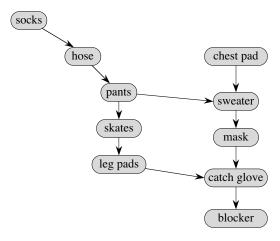
I kept going in this way—choosing an item with no incoming arrows, adding it to the end of the order, and removing the item from the diagram—until no items remained. The three orders shown on page 72 result from making various choices for the item with no incoming arrows, starting from the diagram on page 72.
