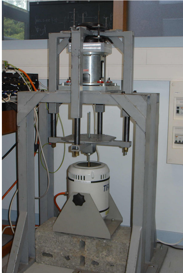
Fig. 1.21 Active vibration control system using an inertial actuator (photo)
