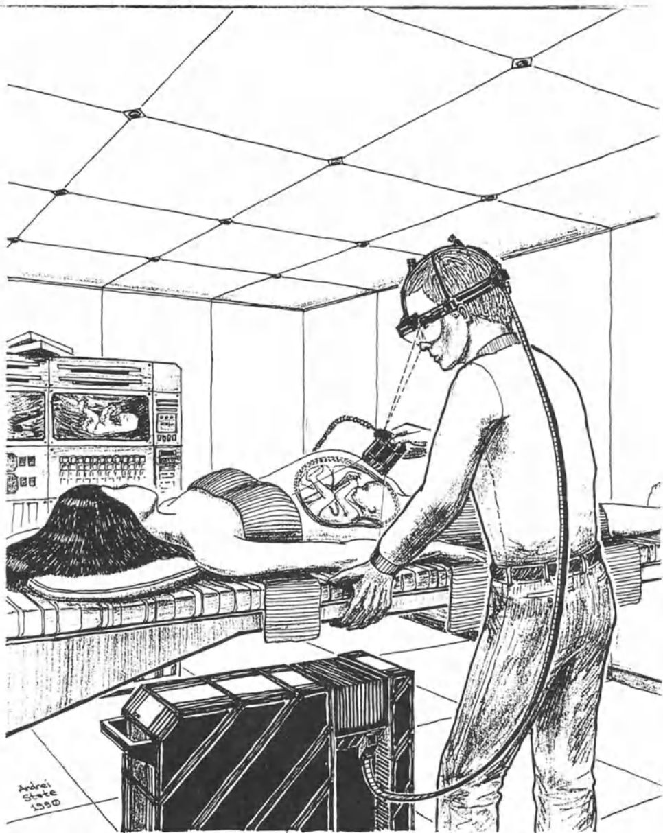
Fig. 7: Conceptual sketch of a future real-time 3D ultrasound display system with a head-mounted display. Physician observes the ultrasound data registered within the patient.
