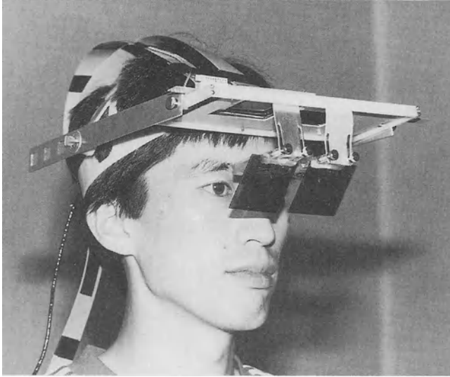
Fig. 4a: Head-mounted display at UNC (1986 vintage). The left and right eye displays are mounted in the visor, pointed down, so that the user observes the computer-generated scene superimposed on his surroundings.
