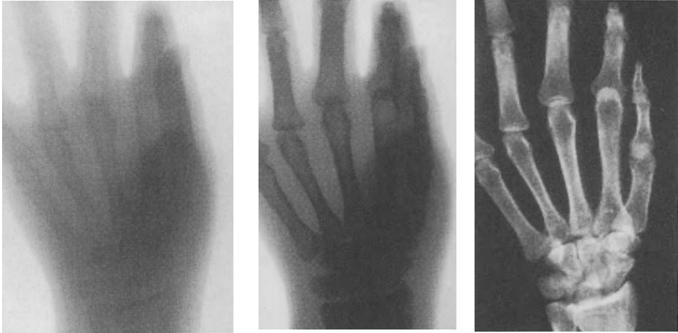
Fig.1 - Dual energy subtraction result for the hand phantom: raw low energy (a) and high energy (b) radiography and “bone only” computed projection (c)
