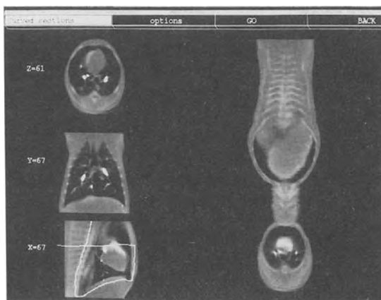
Fig. 7 An example of interactive curved sections showing a trace along an arbitrary path on one section (bottom left) with corresponding section displayed (right).
