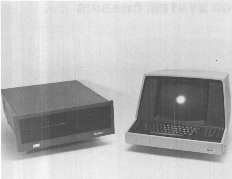
Model 235 Development System. Includes ZX-85 CPU, ZX-200A Disk Controller, and dual 8" floppy disks. Includes ZX-904 for parallel printer and MDS-UPP input/output.
