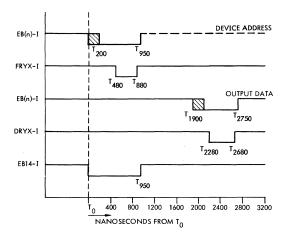
$T_0$  is the start of the execute phase of the data transfer out instruction. Logic levels: true = 0V dc, false = +3V dc.
