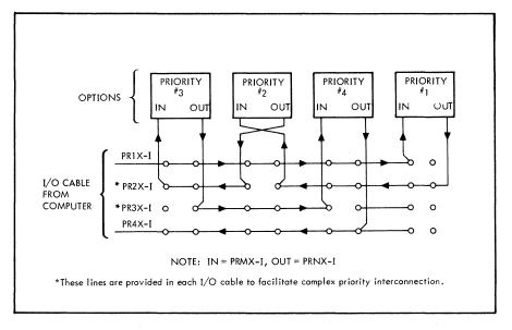
Figure 11-23. Device Interconnection: Device Position Does Not Correspond to Priority Assignment
