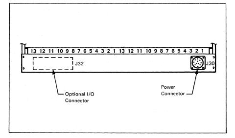
Figure 16-2. Expansion Chassis Connector Panel
