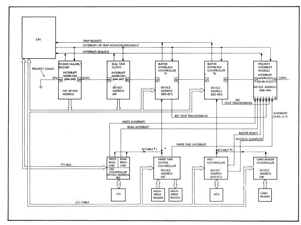
Figure II-1. Typical I/O System Configuration
