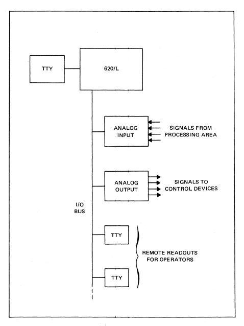
Figure 5-6. Real-Time Process Control
