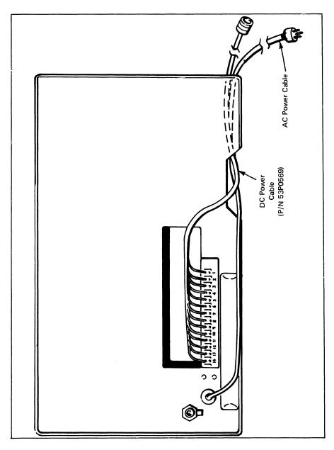
Figure 16-3. Power Supply Connector Panel
