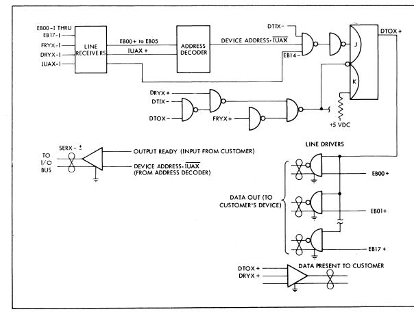
Figure 11-16. **Typical Peripheral Controller Logic: Output Data Transfer**
