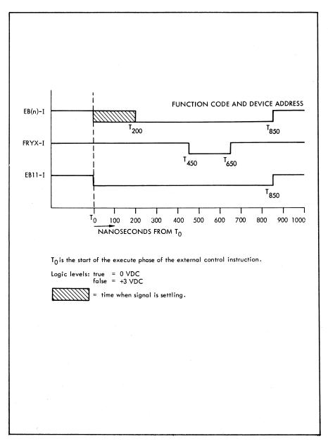
Figure 11-9. External Control Timing
