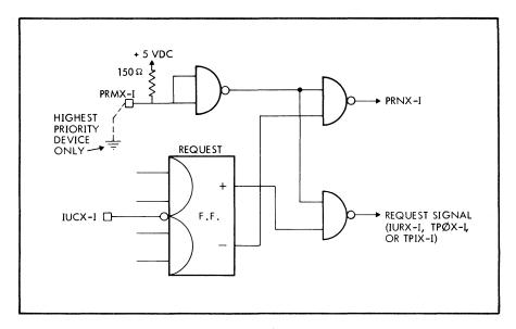
Figure 11-21. Priority Logic Within Controller
