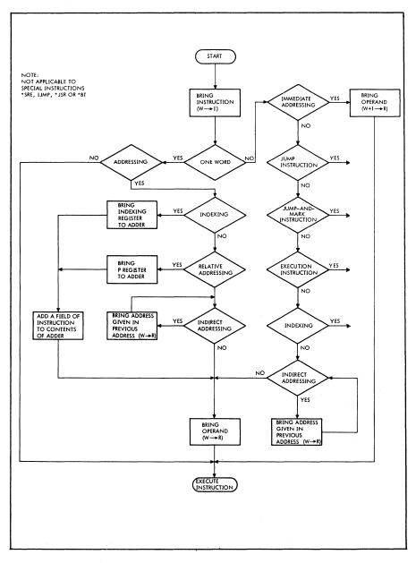
Figure 20-2. Instruction Processing, Simplified Flow
