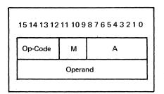
Figure 18-6. Double-Word Non-Addressing (Immediate) Instruction Format
