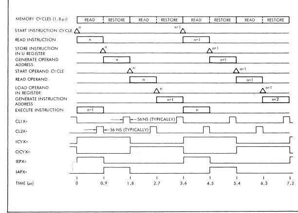
Figure 8-5. Sequence for Operand Access from Memory
