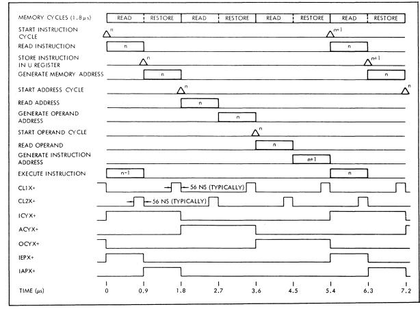
Figure 8-7. Sequence for Indirect Operand Access
