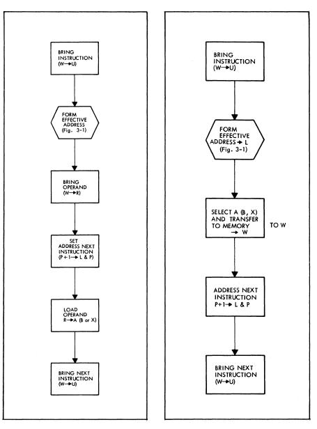
Figure 20-6. Load Type Instruction, General Flow
