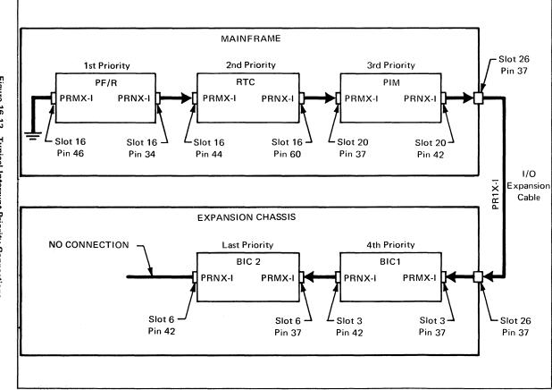
Interconnection of options located in the same chassis is accomplished by connecting the priority-out signal (PRNX-I) of the first priority option to the priority-in signal (PRMX-1) of the next lower priority option. This process continues until all subsequent priorities within the chassis are assigned. The priority-in signal of the first-priority option is connected to ground.
