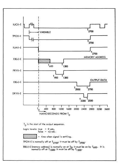
Figure 11-20. Trap-Out Timing
