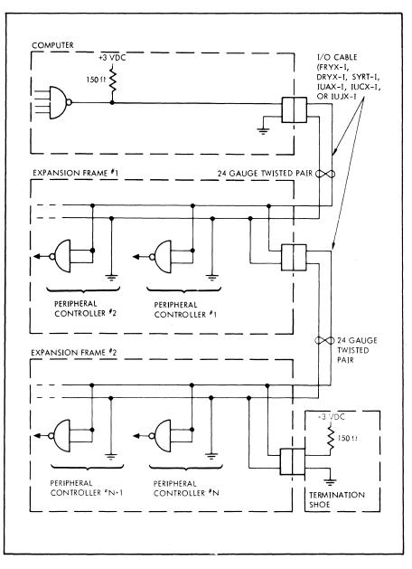
Figure 11-7. Typical Control From The Computer
