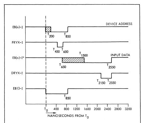
$T_0$  is the start of the execute phase of the data transfer in instruction. Logic levels: true = 0 vdc, false = +3 vdc.
