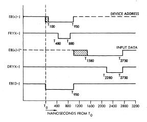
T<sub>0</sub> is the start of the execute phase of the data transfer in instruction. Logic levels: true = 0V dc, folse = +3V dc. = time when signal is settling.
