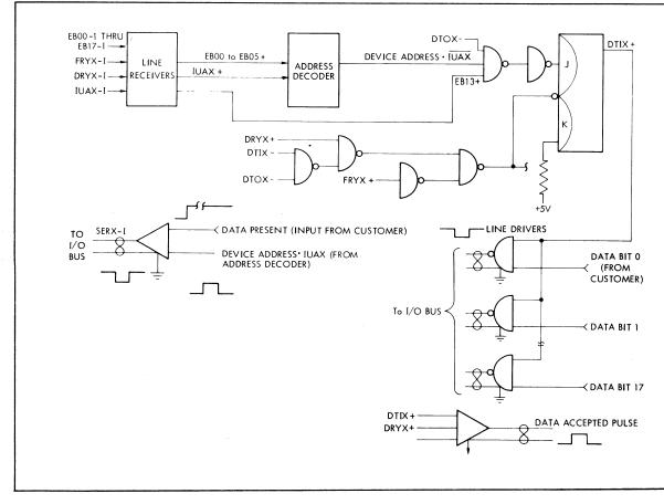
Figure 11-14. **Typical Peripheral Controller Logic: Input Data Transfer**
