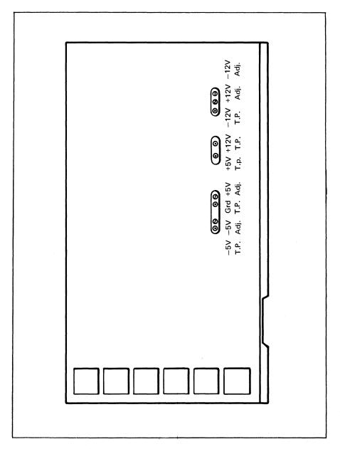
Figure 15-12. Power Supply Top Panel
