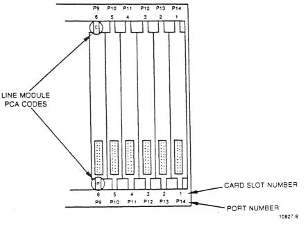
Figure 1-4. Line Module Code
