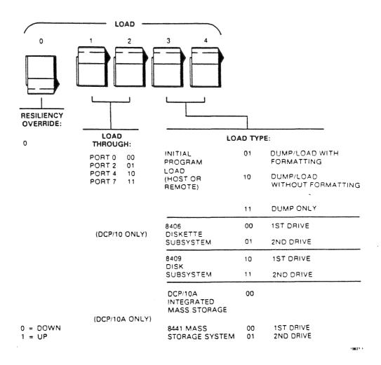
Figure 2-1. Telcon Load Switch Settings
