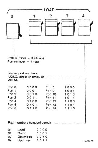
Figure 2-2. Path and Port Number Switch Settings for DCP!OS
