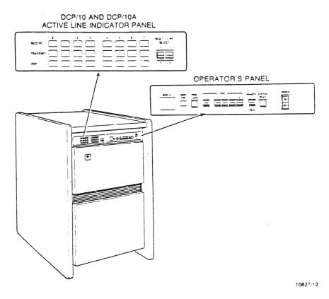
Figure 1-1. Operator Control and Active Line Indicator Panels
