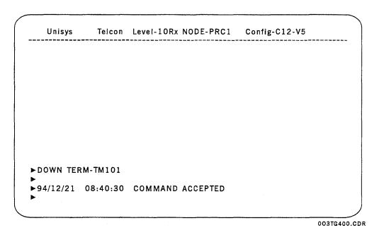
Figure 1-3. NMS Transmitted Command Example
