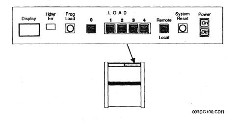
Figure 2-5. DCP/15 Operator Control Panel
