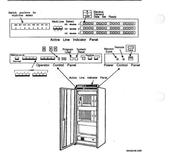
Figure 2-6. DCP/25,30,35,50,55 Operator Control Panel
