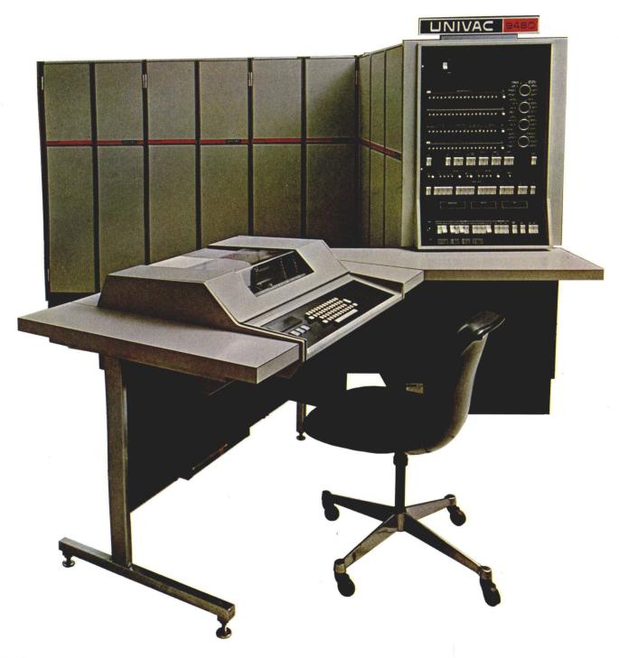
The UNIVAC® 9480 central processor, interval timer, operator's console with keyboard and printer, multiplexer channel capable of handling the keyboard/printer, plus seven subsystems on a shared basis.
