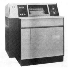
The UNIVAC 0768 Printer Subsystem is a freestanding, self-contained unit. The controlling and synchronizing circuitry, including the 132-character print buffer and the print mechanisms, are housed within the cabinet. This complete printer subsystem is connected to the UNIVAC 9480 System by means of the multiplexer channel. A separate multiplexer channel physical connection and shared subchannel address are required for each printer subsystem.
