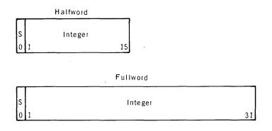
When a halfword binary number is called from storage, it is always expanded to a right-justified fullword; the sign is extended to the left.
