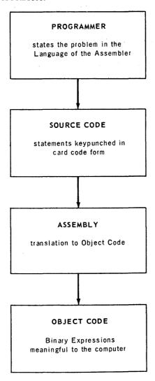
Figure 1-1. Source-to-Object Code Translation with Assembler
