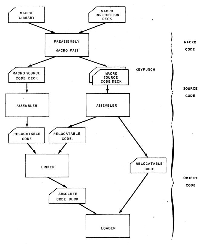
Figure 1-2. UNIVAC 9200/9300 Assembly System
