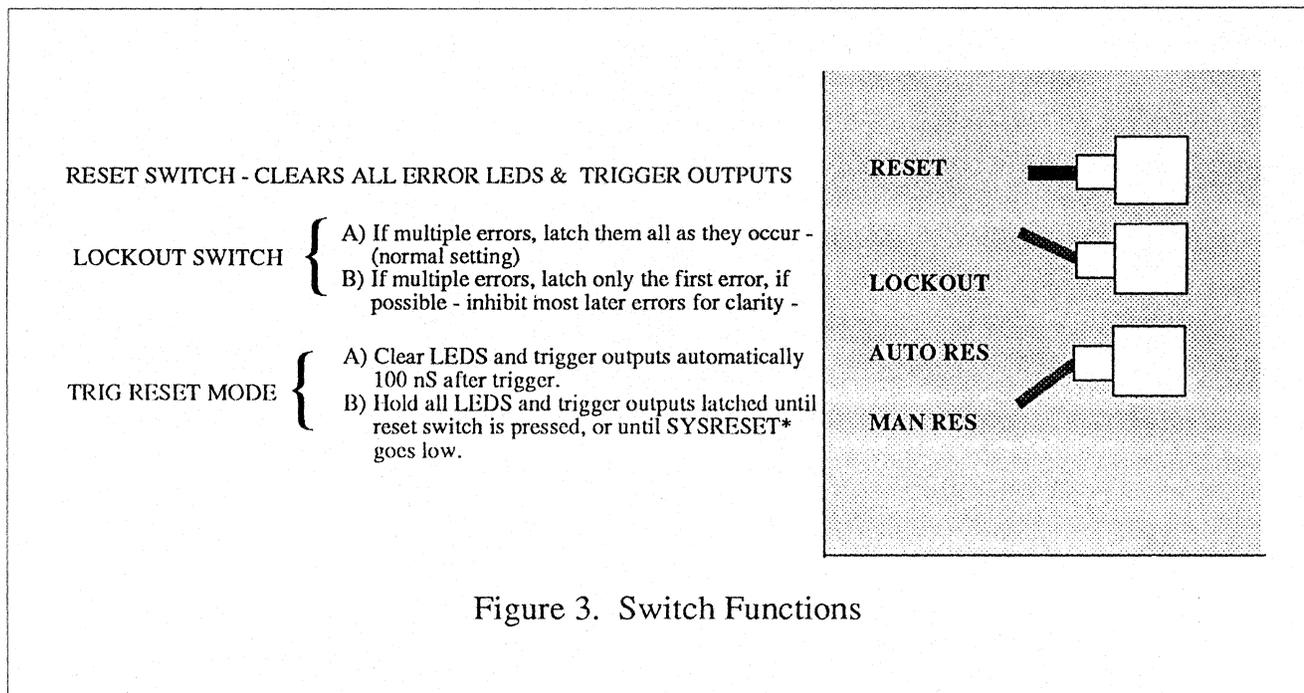
Figure 3. Switch Functions
