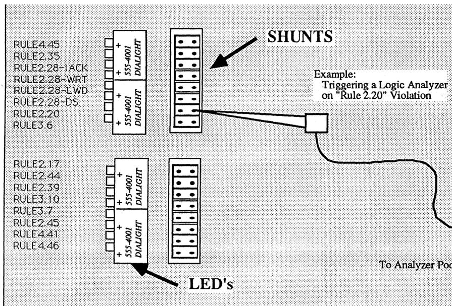
Figure 4. "Error-Enable" Jumpers
