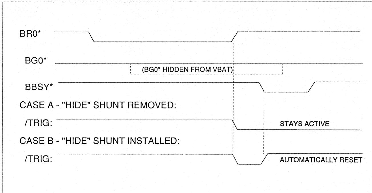
To prevent the above temporary false indication, locate the VBAT in as leftwards a slot as possible in the backplane (without locating it before the arbiter, of course). In this way the bus grant signal will not be blocked by a master using the bus.
