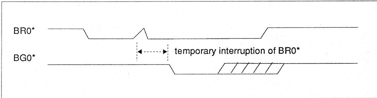
**CONDITION WHICH WOULD CAUSE A FALSE MOMENTARY ERROR INDICATON WHEN NONE IN FACT EXISTS:**
