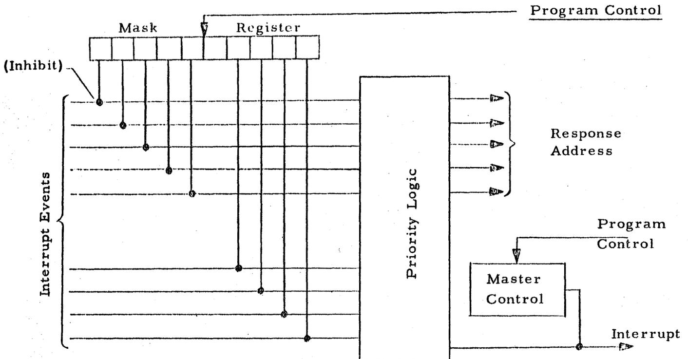
A master interrupt control is provided which is under program control. Individual interrupt mask registers enable program priority control over each interrupt as desired.
