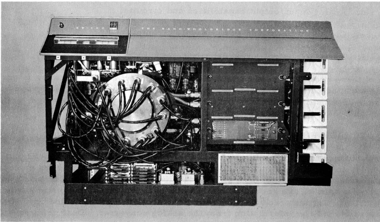
Figure 3-1. RW-300 with Front Panel Removed
