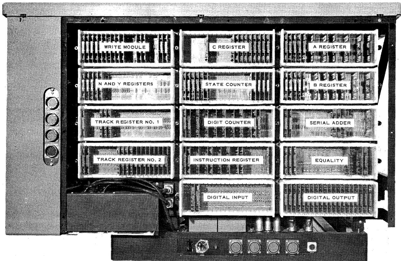
Figure 3-9. Back of RW-300 Computer with Rear Panel Removed to Show Location of Modules.
