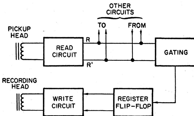
Figure 3-17. Typical 20-Bit Circulating Register, Block Diagram
