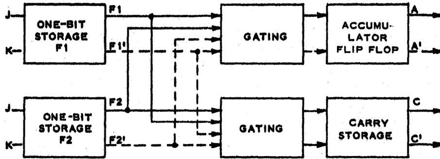
Figure 2-6. Functions (Logical Elements) Required For Binary Manipulation
