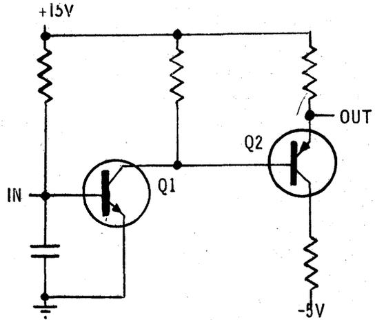
Figure 2-17. High Level D-C Converter, Schematic
