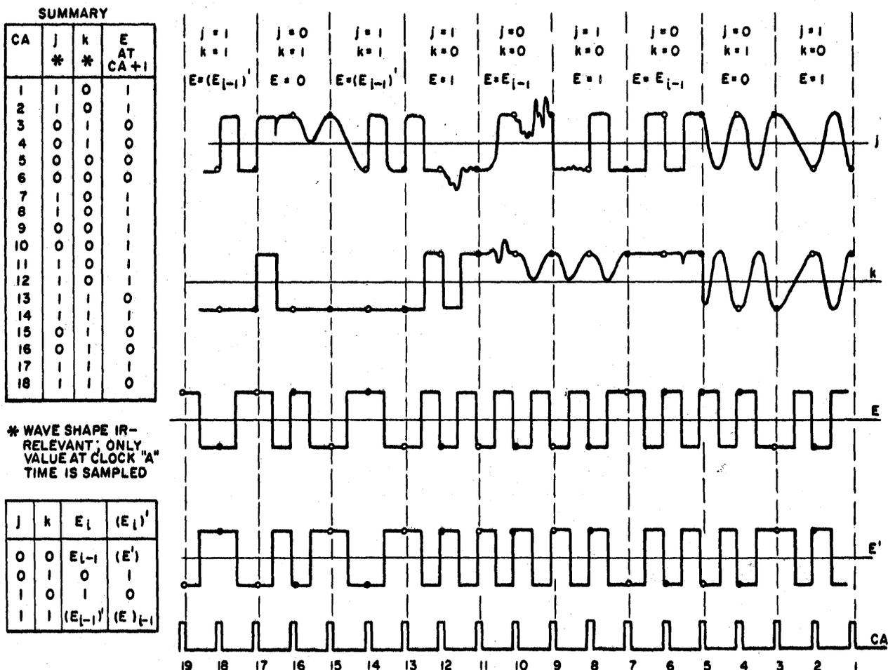
Figure 2-10. Idealized Waveshapes From A Dynamic Flip Flop Under Various Input Signal Conditions
