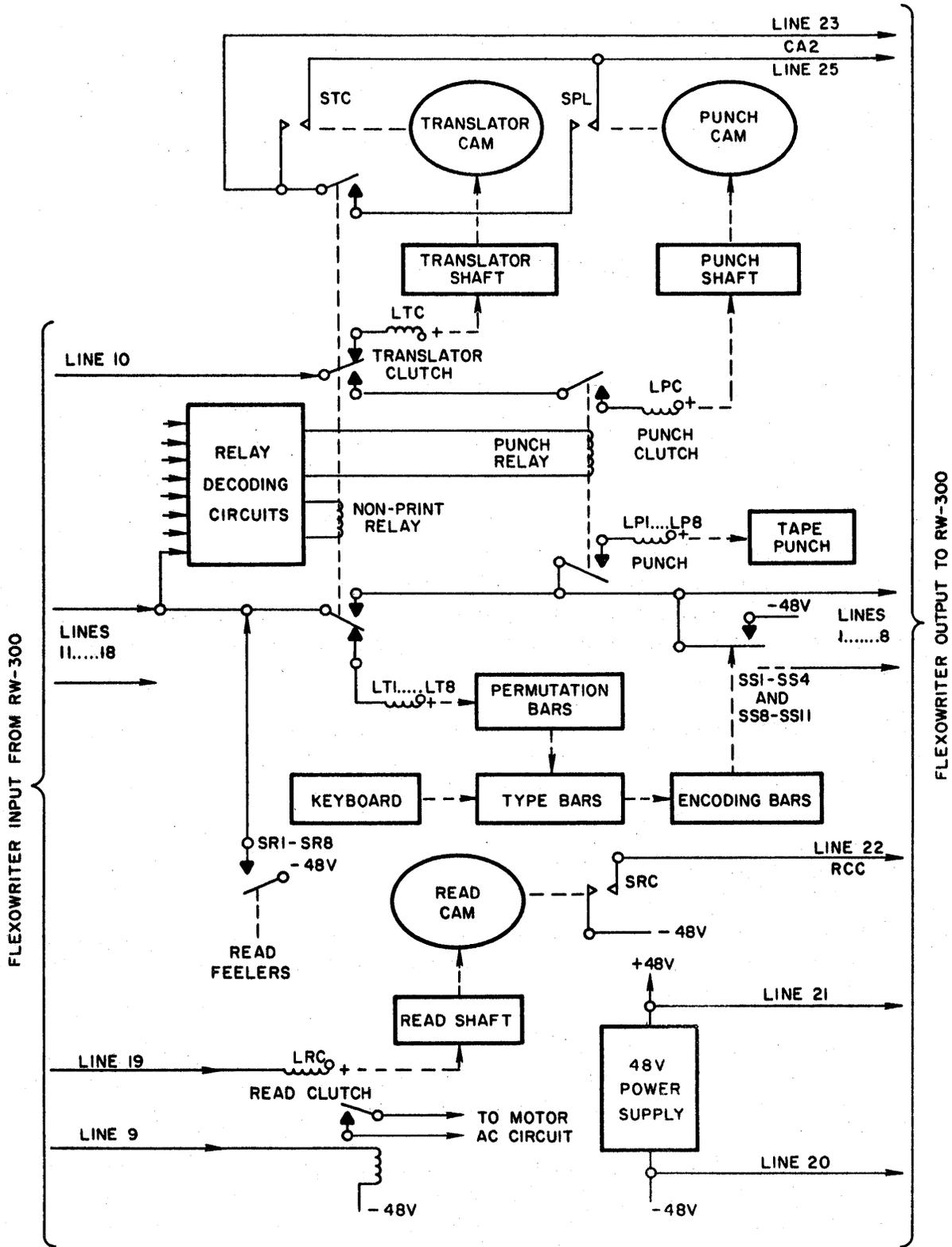
Figure 3-24. Flexowriter, Simplified Connections
