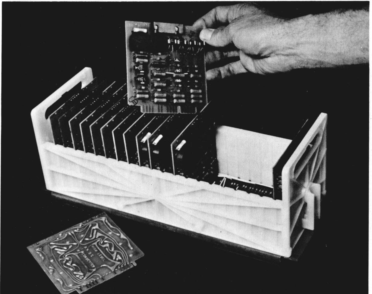
Figure 1-3. Typical RW-300 Module with Insert Card
