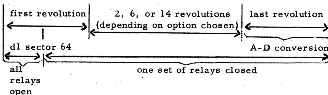
If the noise level is high on the low level inputs, 14 drum revolutions are necessary for amplifier stabilization and four flip flops are required in the counter. If the noise level is low, flip flop X13, or X13 and X12, may be omitted. In these cases, six or two drum revolutions occur between "first" and "last" revolutions.
