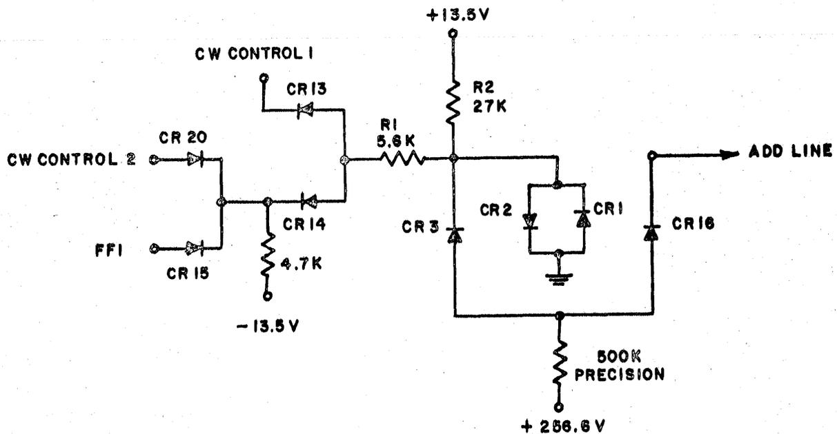
Figure 3-30. Current Conversion Technique, Partial Schematic
