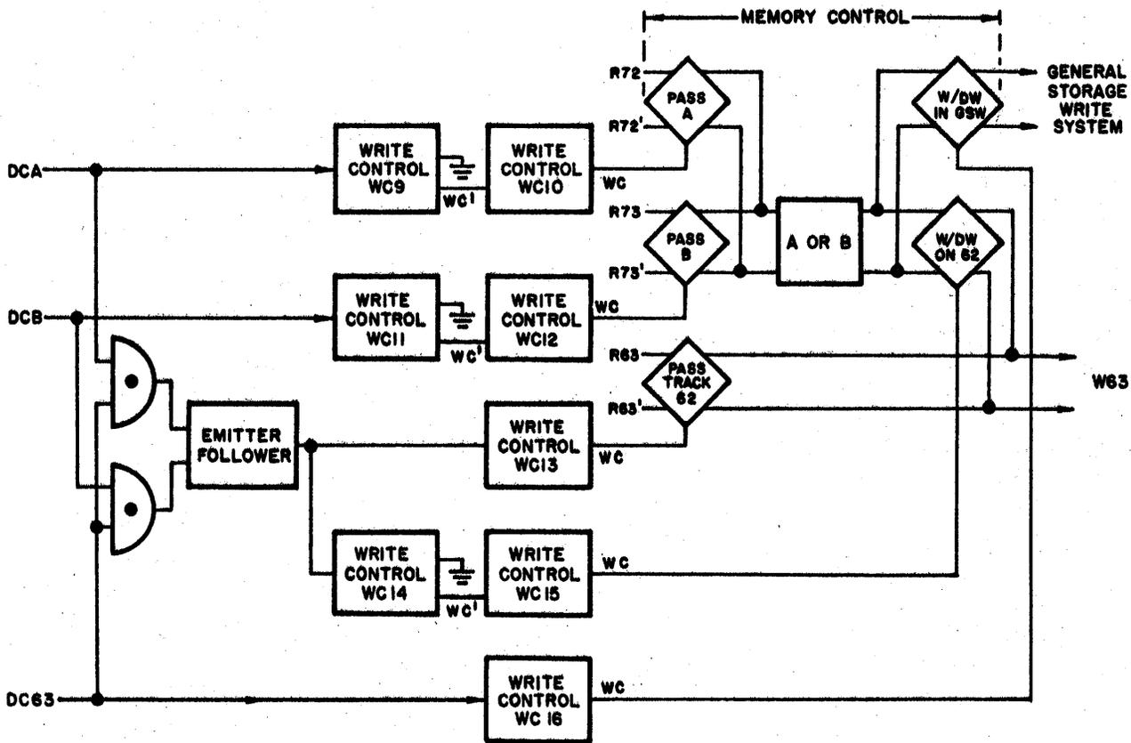
Figure 3-11. Write Control System, Block Diagram
