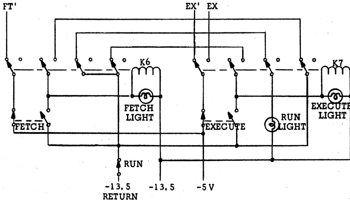
Figure 3-36. Circuit for Suspending Computer Operation, Simplified Schematic
