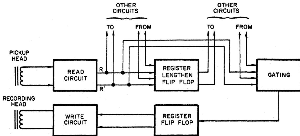
Figure 3-16. Typical 19-Bit Circulating Register, Block Diagram
