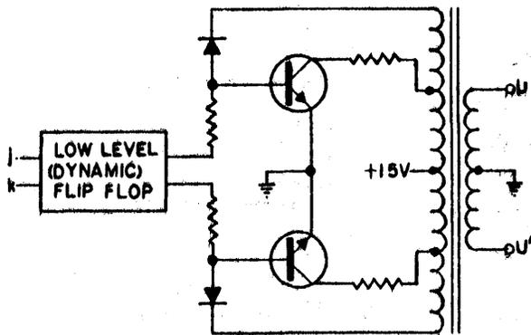
Figure 2-13. High Level Flip Flop, Simplified Diagram
