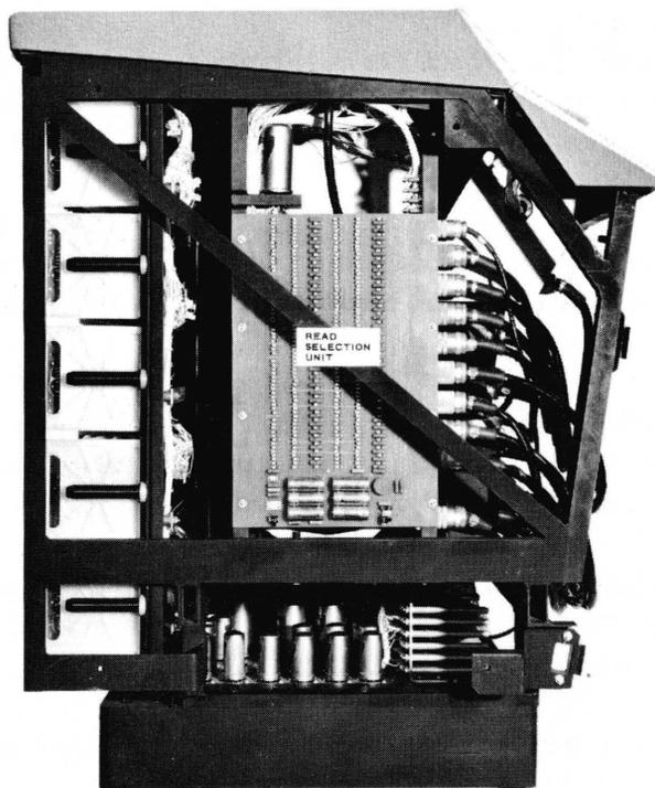
Figure 3-6. Left Side of RW-300 Computer with Side Panel Removed.
