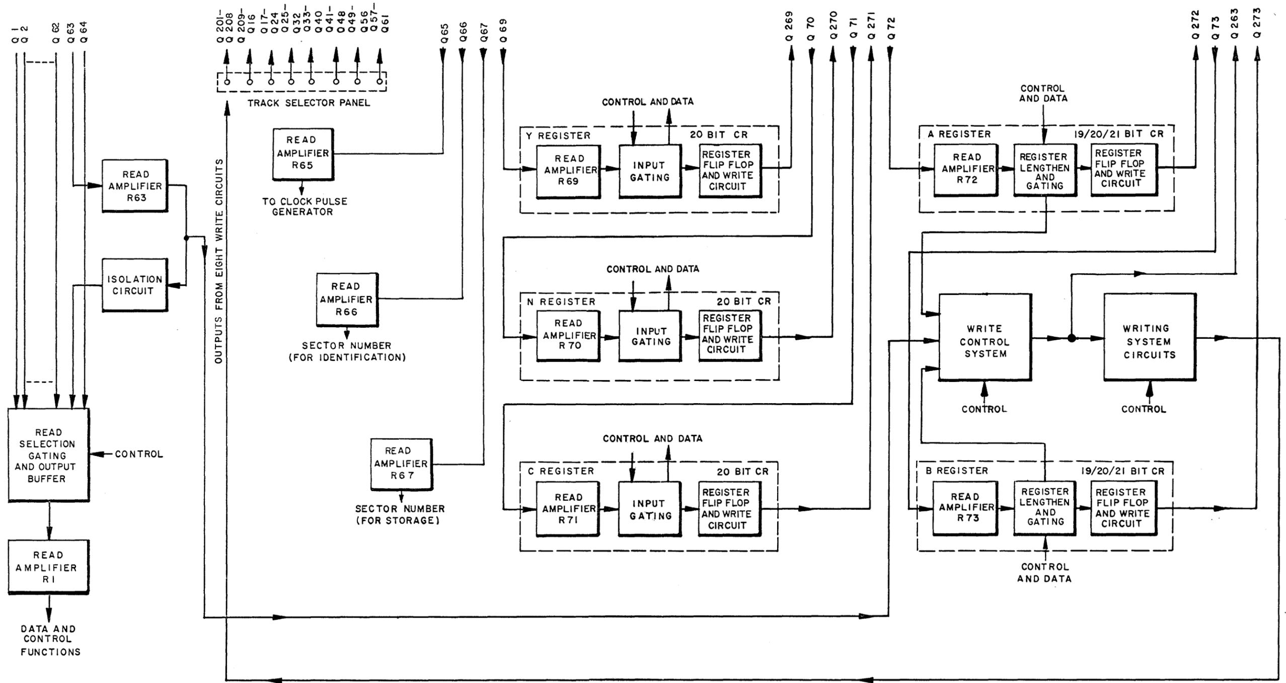
Figure 3-5. Read and Write System, Block Diagram
