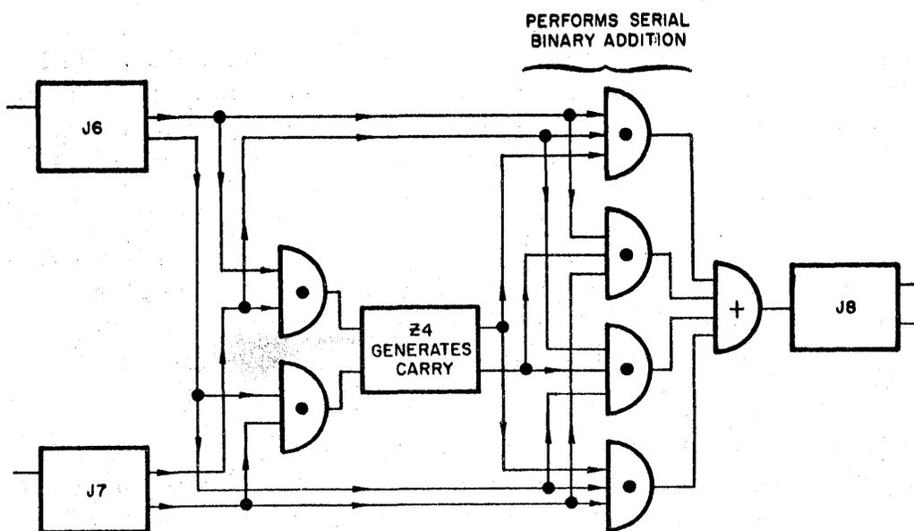
Figure 3-18. Adder Circuits, Simplified Block Diagram
