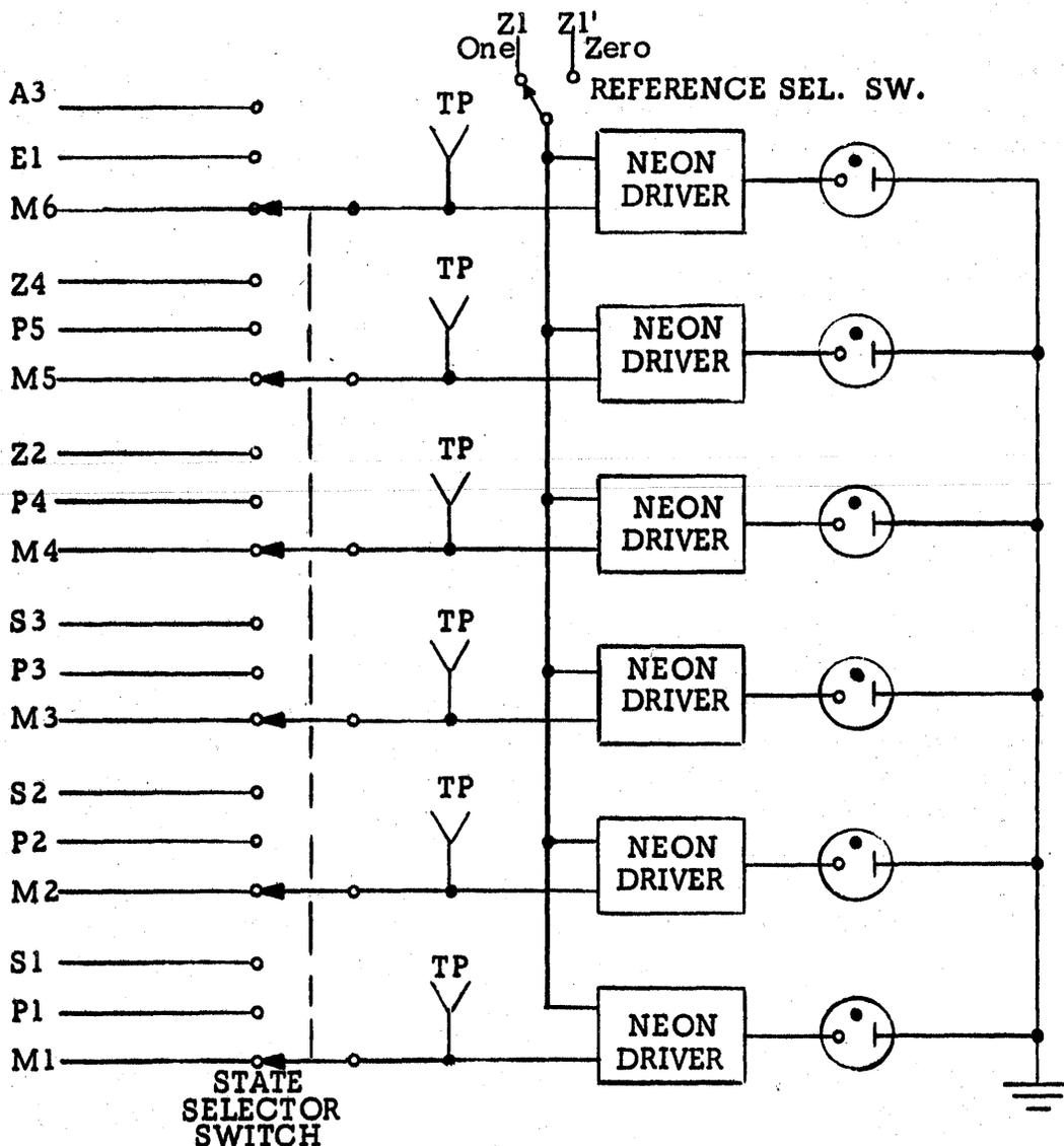
Figure 3-38. State Indicators, Simplified Schematic
