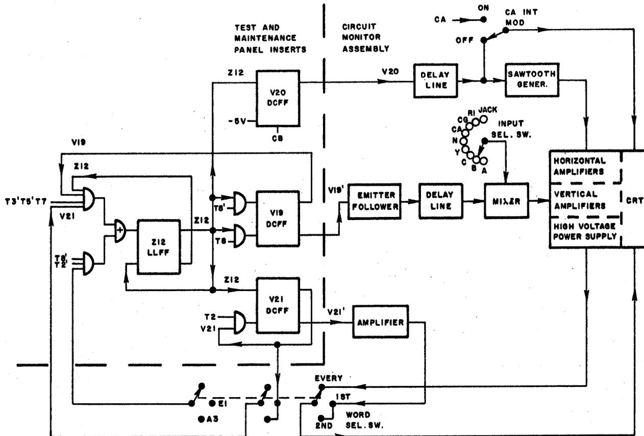
Figure 3-37. Circuit Monitor Display Functions, Block Diagram
