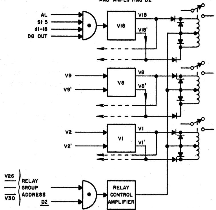
Figure 3-26. Digital Output Systems, Block Diagrams
