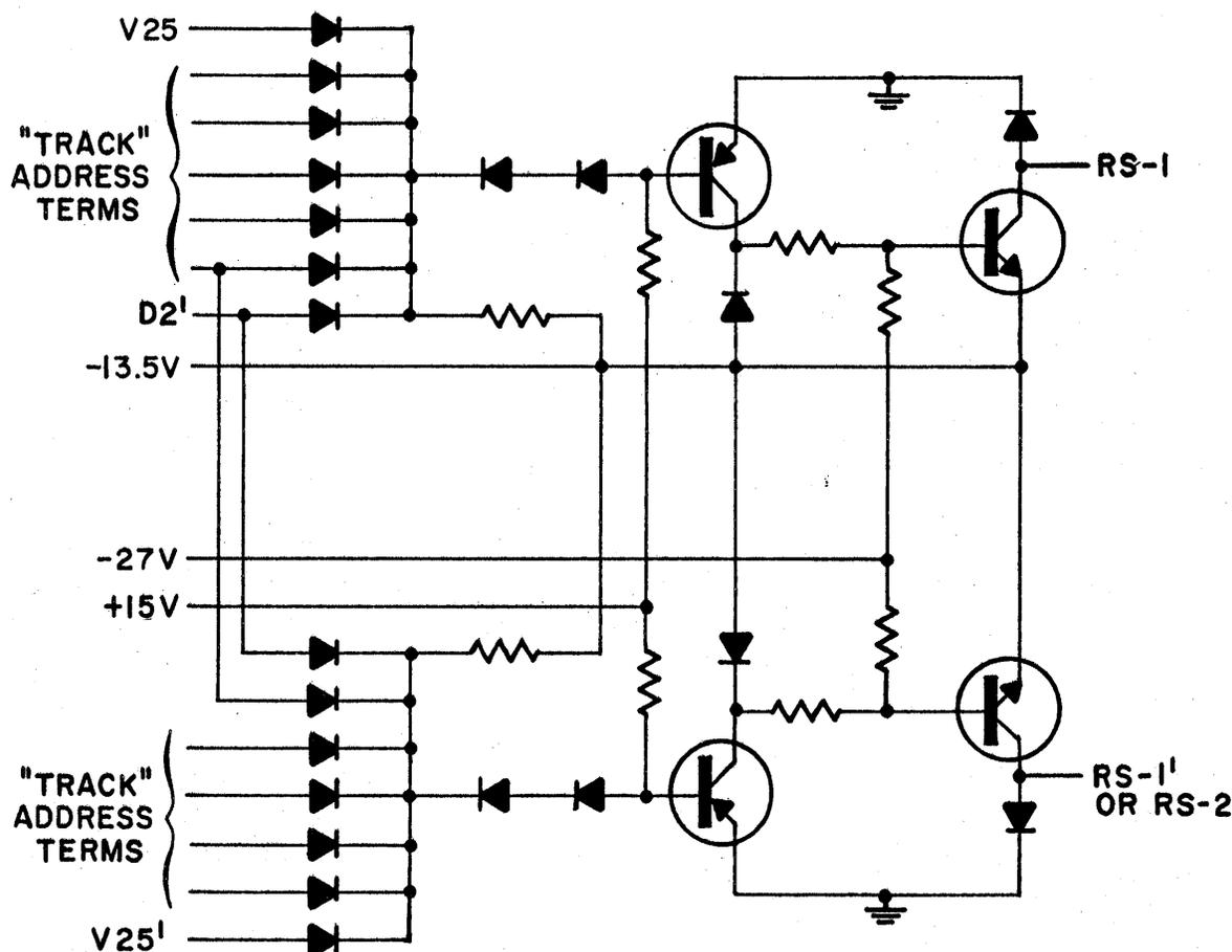
Figure 3-28. Relay Control Amplifier Pair, Schematic
