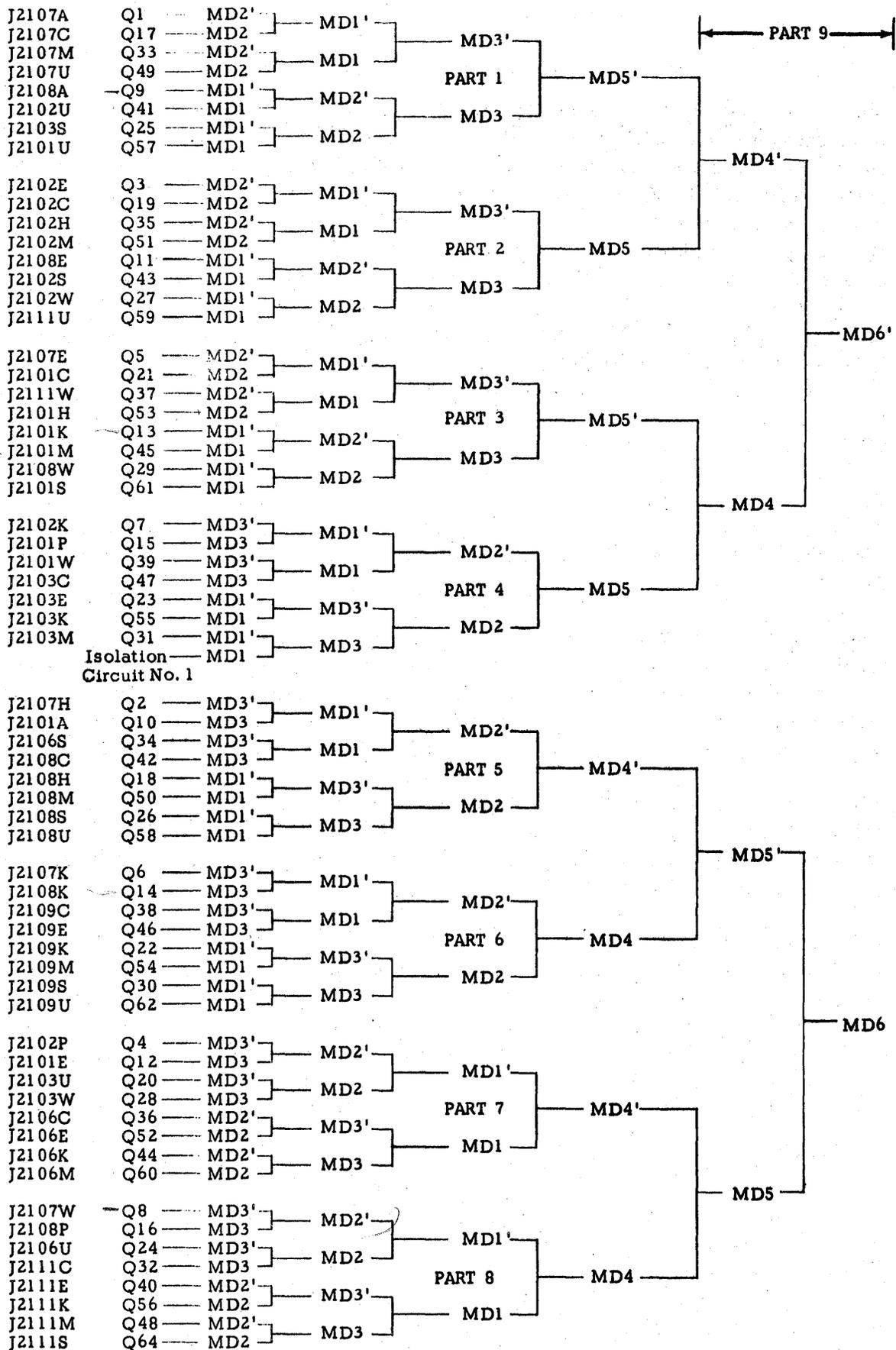
Figure 3-8. Reading Head Selection Gating
