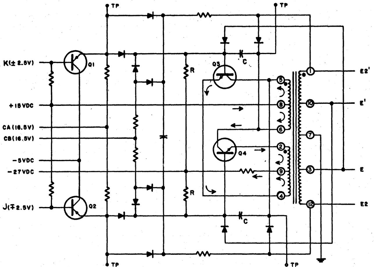
Figure 2-9. Dynamic Flip Flop, Basic Schematic
