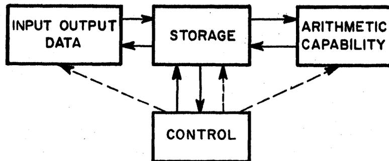
Figure 2-1. General Computer Functions, Block Diagram
