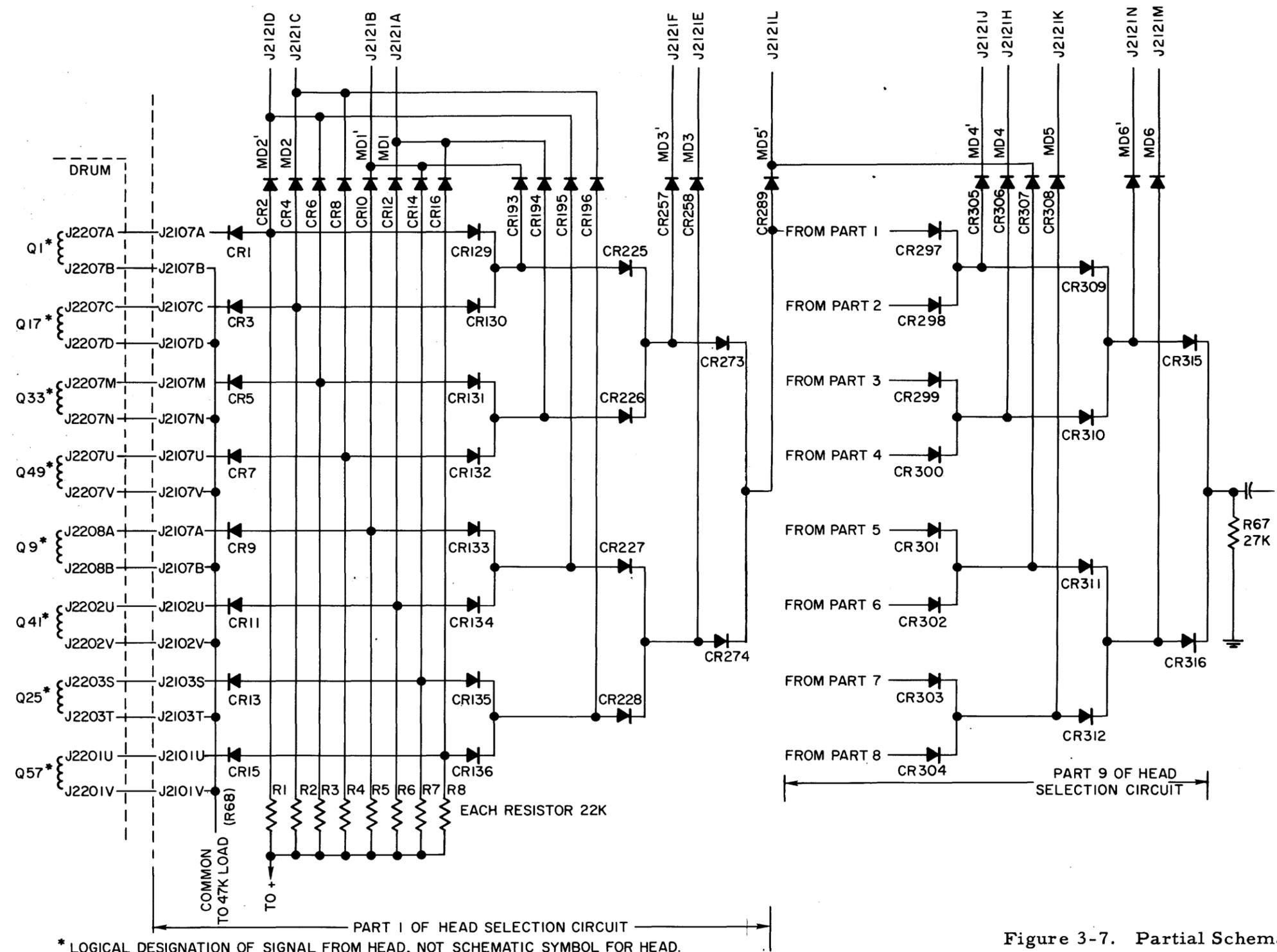
Figure 3-7. Partial Schematic of Gating Structure Used in RW-300 Read Selection Unit
