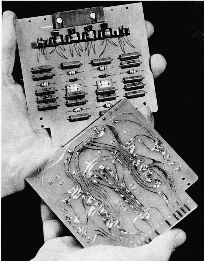
Figure 1-4. Typical Insert Card.
