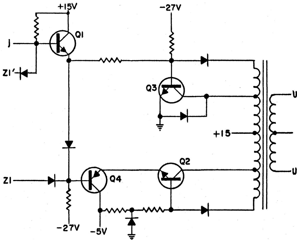
Figure 2-18. Matrix Amplifier, Schematic
