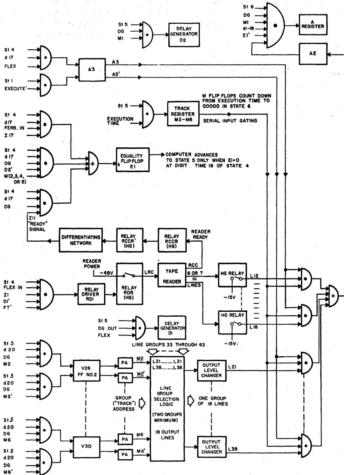
M2' IS IN PHASE TO M2, ETC., BUT IS FORMED BY INVERTING AND AMPLIFYING M2, ETC.
