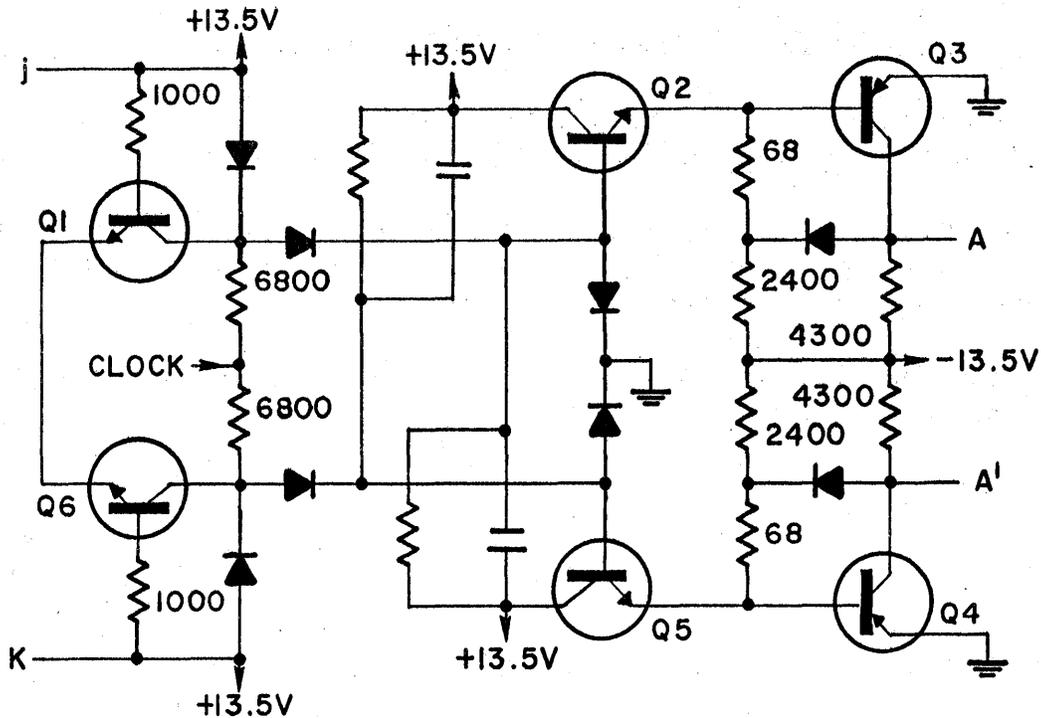
Figure 3-27. Flip Flop No. 2, Schematic
