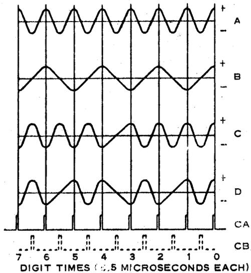
Figure 2-8. Typical Read Head Outputs
