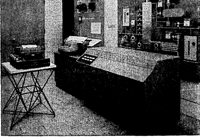
Figure 3. The Thompson Ramo Wooldridge RW-300 Digital Control Computer. Combined typewriter, paper tape punch, and tape reader (left); data-logging typewriter (center).
