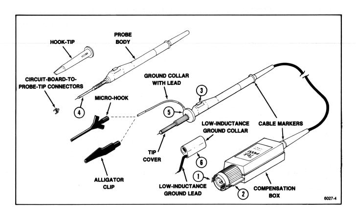
Figure 2-3. Controls, connectors, and probe accessories.
