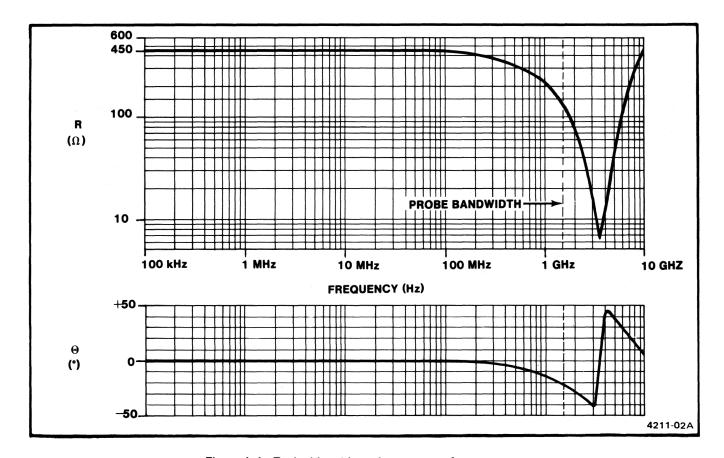
Figure 1-1. Typical input impedance versus frequency.
