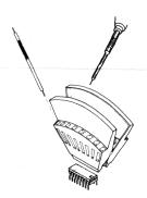
ECB to Probe-Tip Adapters provide high-quality connection test points when installed on circuit boards. The ribbed-plastic tip cover on the probe must be removed. The probe will then plug into the test point directly. Adapters are available in bags of 100 (see "Replaceable Parts.")
