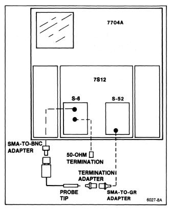
Figure 3-1. Offset check setup.
