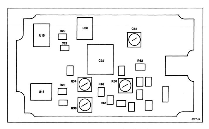
Figure 7-3. Main circuit board component layout for trouble shooting.
