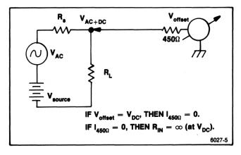
Figure 2-4. Example of reduced loading.
