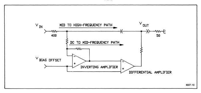
Figure 5-1. Functional block diagram.
