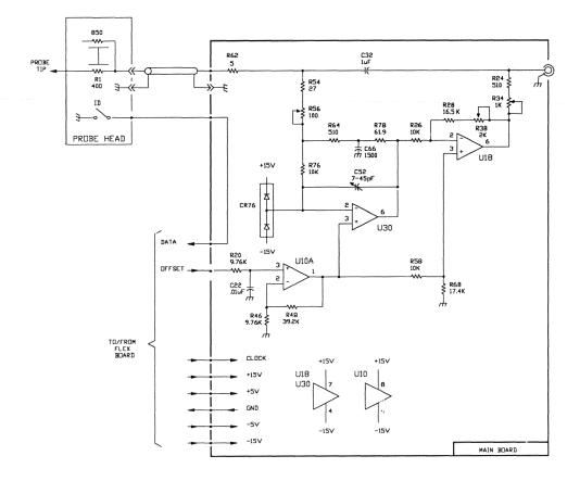
Figure 7-1. Main circuit board schematic.
