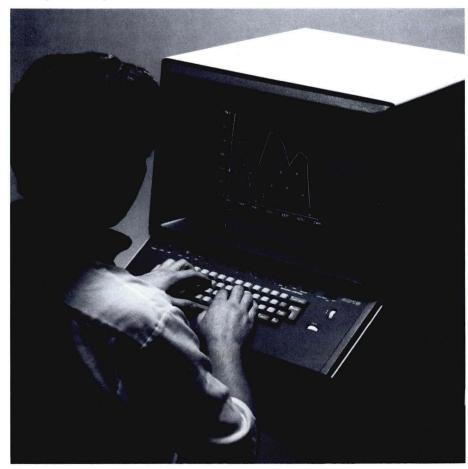
The 4015 Computer Display Terminal adds the powerful problemsolving APL language to the increased display power of the 19 inch screen, along with the full ASCII upper and lower case set and TTY subset.
