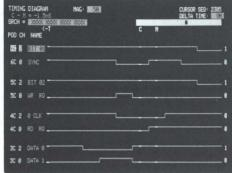
Figure 3. Delta Time timing diagram w/1.5 ns measurement
