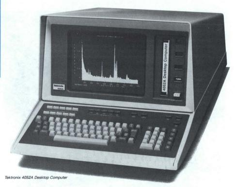
Tektronix 4050 Series systems have an exclusive high-resolution storage display for unexcelled graphic clarity and detail. There is no distracting screen flicker. All lines are continuous, never detracting from or distorting information.
