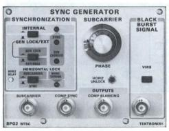
The SPG2 and SPG12 Sync Generators have gen-lock capability. The almost identical SPG1 and SPG11 do not.
