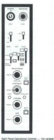
aperture control is concentric with the contrast control.
