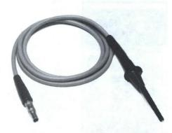
The P6601 Probe is a temperature measuring device designed to operate with the DM 502A and DM 501A Digital Multimeters. The temperature sensing element consists of a thin-film platinum resistor on the tip of the probe. Measurements are made by touching the sensing element to the surface whose temperature is in question. The thermal signal is transmitted to the associated digital multimeter through a two-conductor cable.
