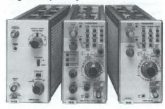
Plug-in compatibility. The 7104 is compatible with standard 7000 Series plug-in units that provide for full 7104 System performance.
