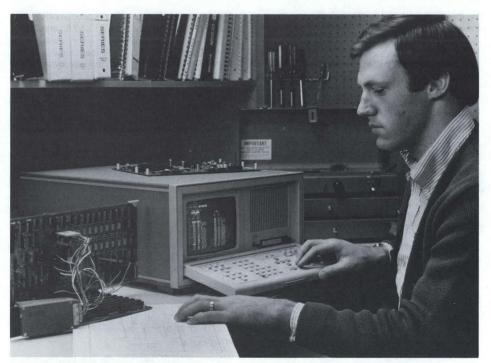
With versatile software and hardware analysis and stimulus capabilities, the DAS is complete design engineers tool.
