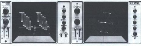
1420 NTSC Vectorscope shown side-by-side with a 528A Waveform Monitor
