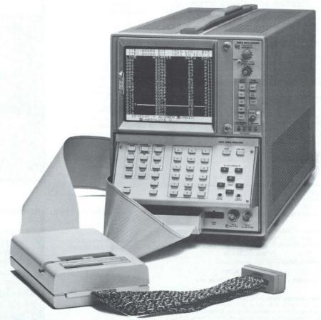
Setup/Hold Time - Determined by Personality Module used. Number of Qualifiers — Six maximum (can shift or divide qualified clocks by up to four positions or times).
