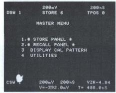
The master menu offers a convenient way to enable special functions such as the STORE and RECALL of front panel settings and also allows you to branch-out to other menus.
