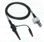
The P6125 is a low-capacitance, 5X attenuation passive probe specially designed for use with counter/timers. It makes possible more accurate time interval measurements of high speed logic signals. Five-times attenuation provides an optimum match between the counter input characteristics and the voltage levels of all common logic families. The low input capacitance permits acquisition of high frequency signals with minimum loading of the circuits under test.
