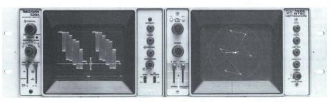
528A Waveform Monitor mounted side-by-side with a 1420 Vectorscope in optional rack adaptor.
