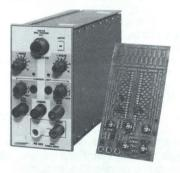
The front-panel circuit-board kit is a convenient way to mount small experimental circuits or fixtures right on the front of a TM 500 Power Supply.
