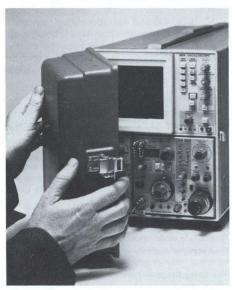
Option 08 protective front cover is shown with 7613 Mainframe.
