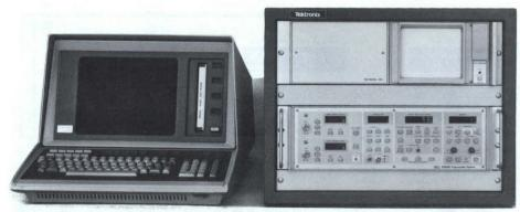
Figure 5. 390AD operating under control of a Tektronix 4052A Desktop Computer equipped with signal processing ROM Packs
