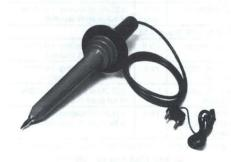
The High Voltage Probe will measure dc voltages from 1 kV to 40 kV with an accuracy of 1% at 25 kV. The division ratio is 1000:1. Common uses include measuring anode voltages on monitors or oscilloscopes. Probe plugs directly into the front end of the multimeter.
