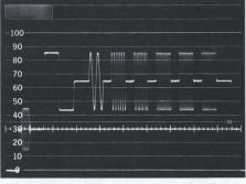
420 mV multiburst. Notice burst starts and stops precisely at the same level.
