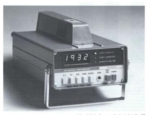
The Tektronix J16 is a portable digital photometer/radiometer capable of making a wide variety of light measurements—in the laboratory or in the field.
