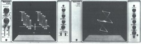
1424 XY Display Monitor shown side-by-side with a 528A Waveform Monitor
