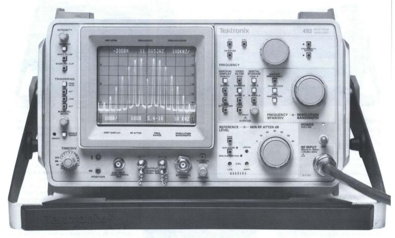
The 492P complies with IEEE Standard 488-1978, and with Tektronix Standard Codes and Formats.
