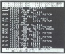
This 8086 mnemonic display shows disassembled instructions entering the 8086 queue. In this illustration instructions that enter the queue but are not executed are flagged with question marks. Operands for which there is no data (as when the instruction is flushed before the operand is retrieved) are marked with asterisks. (7D02 Display)
