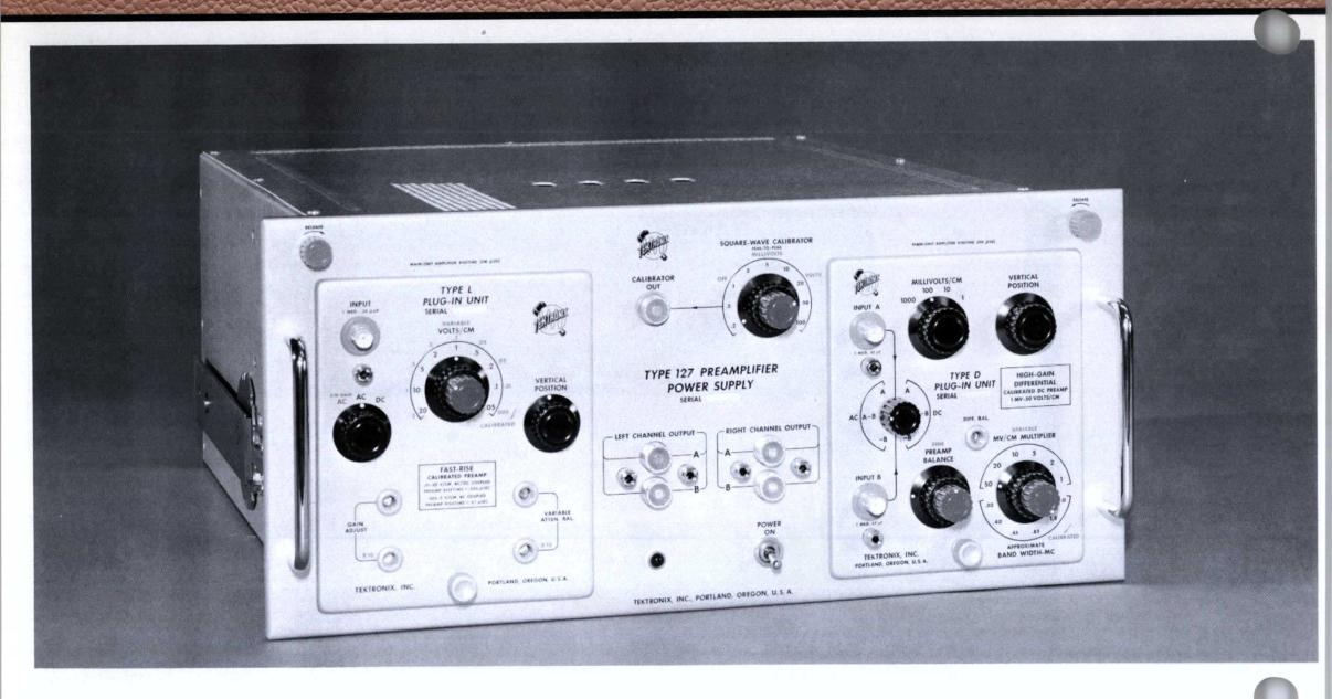
The Tektronix Type 127 Preamplifier Power Supply provides operating power to one or any combination of two Tektronix Letter Series or new '1' Series Plug-In Units. This permits the operation of Tektronix Plug-Ins separate from the oscilloscope in which they are normally used. For example, a double-differential dual-trace display can be obtained with a Type 127 and two Type D, E, or G Plug-In Units—when used in conjunction with an oscilloscope and Type C-A, 1A1, or 1A2 Plug-In Unit.
