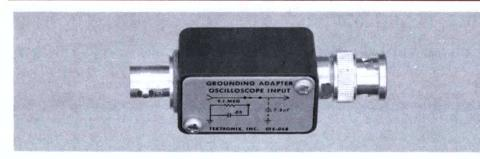
PROBE GROUNDING ADAPTER for Tektronix 10X probes provides a convenient method of establishing the vertical position of the oscilloscope trace in relation to the zero volts input at the probe tip. The adapter eliminates the need moving the probe tip from the signal source to ground.
