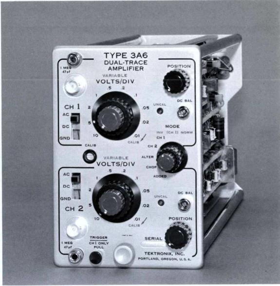
The Type 3A1 and Type 3A6 Amplifiers are general-purpose dual-trace plug-in Units. They are identical in every respect except that the Type 3A1 does not have a signal-delay line. The Type 3A6 does contain an internal 260 nanosecond signal-delay line that allows viewing of the leading edge of the sweep-triggering waveform when using a high-speed time base such as the Type 3A1, 3B3 and 3B4 Time-Base Units\*.
