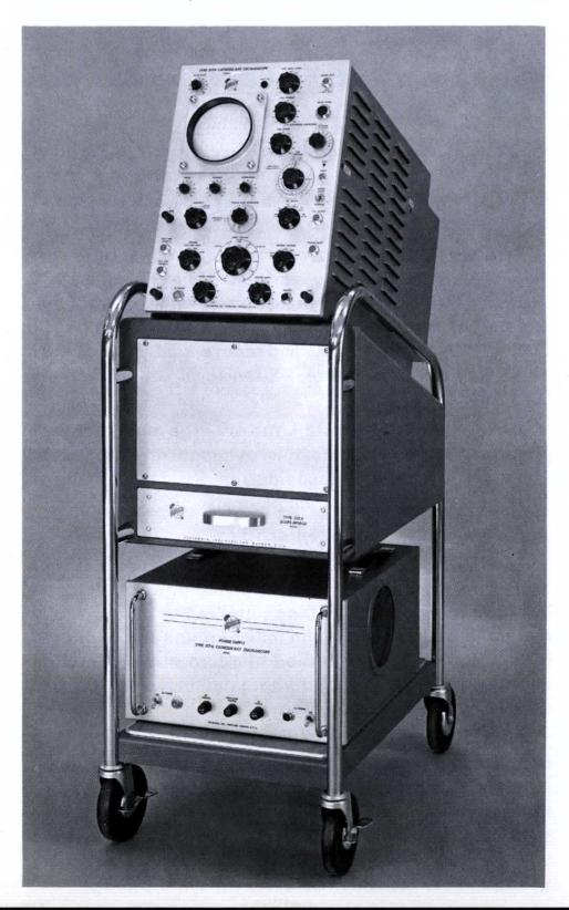
**Illuminated Graticule**—An edge-lighted graticule is marked in centimeter squares, 4 vertical and 8 horizontal, for convenience in making time and amplitude measurements. Illumination is controlled by a frontpanel knob.
