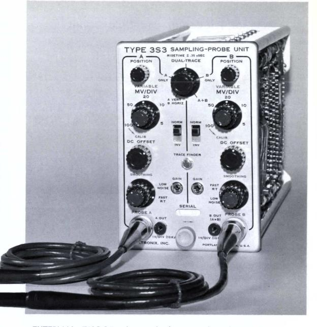
**EXTERNAL TRIGGER** is required, approximately 50 nsec prior to signal. Minimum repetition rate is 50 cps.
