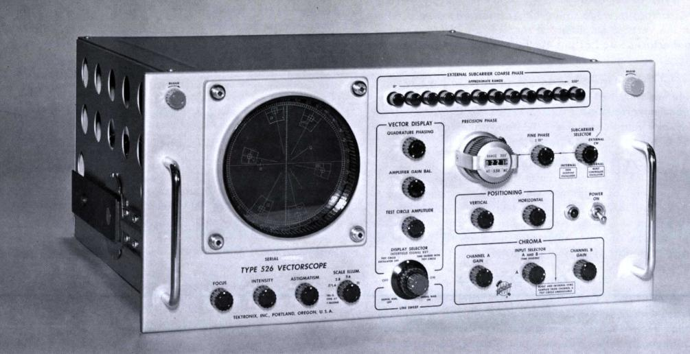
Differential Phase and Differential Gain Measurements—To 0.1° and under 1%.
