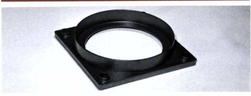
BEZEL—For mounting cameras, other than Tektronix types, on Tektronix 5" Oscilloscopes. Dimensions— $5\frac{7}{8}$ " square; ring  $\frac{7}{8}$ " deep, diameter  $\frac{55}{8}$ " outside,  $\frac{51}{8}$ " inside. Die-cast construction.
