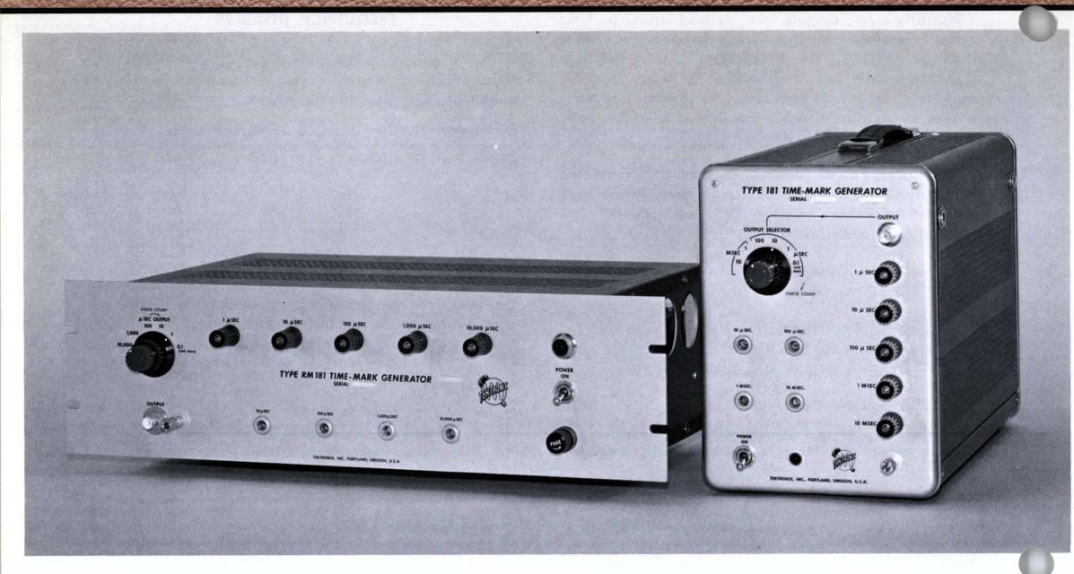
The Type 181 and RM181 provide accurate time-markers of 1, 10, 100, 1000, and 10,000 microseconds, plus a 10-Mc sine wave. These markers are used for oscilloscope sweep calibration and comparison time measurements. Any of the six signals can be switched to a front-panel output connector. Also the five time-markers are available separately at front-panel binding posts.
