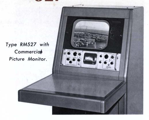
**Power Requirement**—105 v to 125 v or 210 v to 250 v, 50 to 60 cps, typically 206 watts at 117 v.
