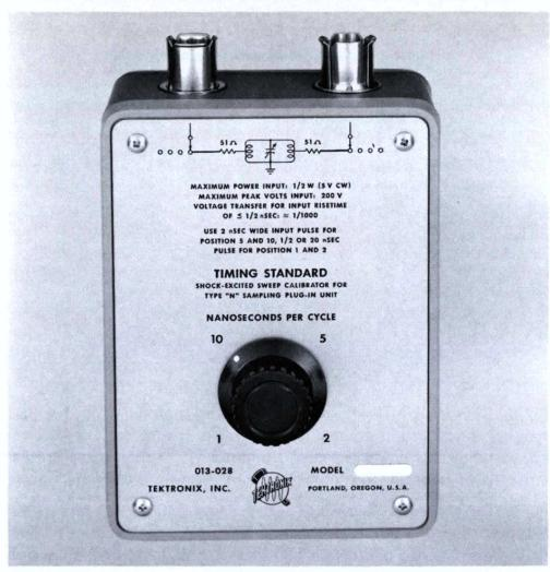
The Timing standard is a 3% device for calibrating equivalent sweep speeds of the Tektronix sampling systems. It is designed to ring at periods of 1, 2, 5, and 10 nsec when excited by a fast-rising pulse.
