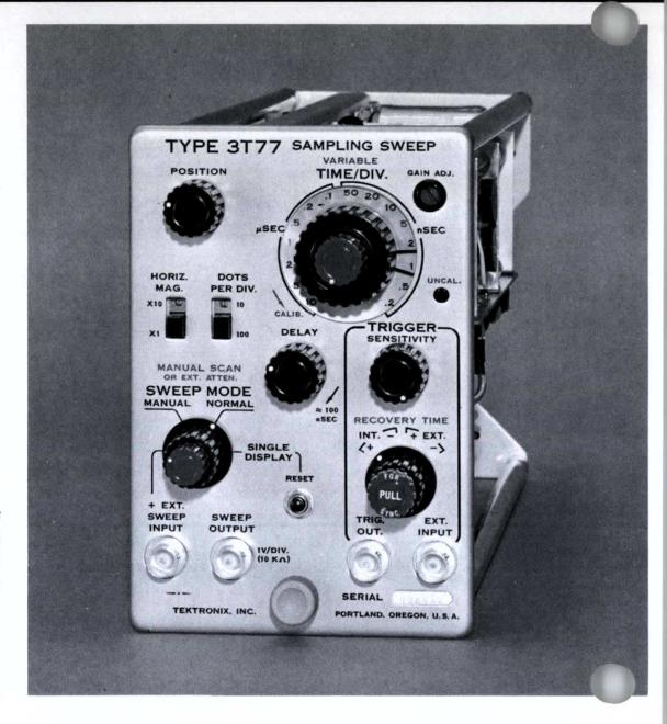
10X MAGNIFIER extends the calibrated sweep rate to 0.02 nsec/div.
