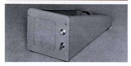
TYPE 310/310A FAN BASE provides filtered forced-air ventilation to reduce operating temperature when the instrument is used continuously for prolonged periods of time or in a hot or limited-ventilation area. The Fan Base tilts the oscilloscope to a convenient viewing angle.
