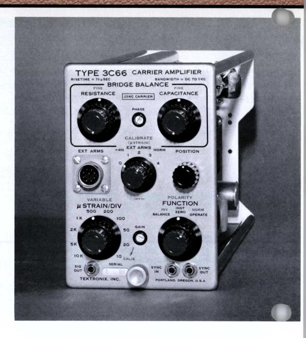
CALIBRATED SENSITIVITY is from 10 microstrain/div (microinches per inch/div) to 10,000 microstrain/div when the Type 3C66 is used with a single strain gage having a gage factor of approximately 2. Uncalibrated continuous control from 10 microstrain/div to 25,000 microstrain/div.
