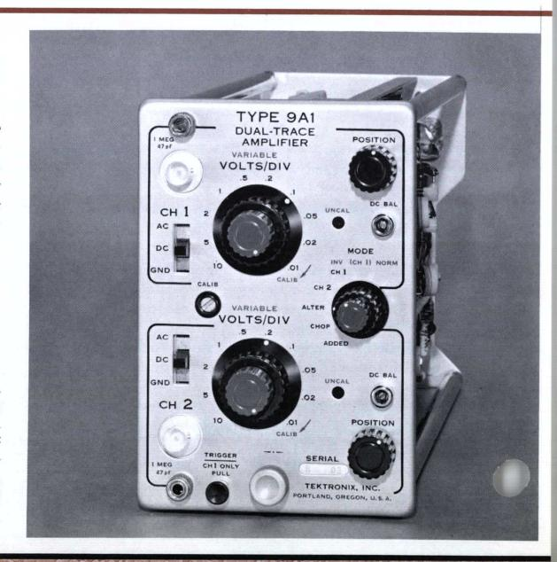
**CALIBRATED SENSITIVITY** is 10 mv/div to 10 v/div in 10 steps, 1-2-5 sequence. Variable control for each channel permits continuous, uncalibrated adjustment between steps and to 25 v/div. Accuracy of calibrated positions is  $\pm 3\%$  of indicated deflection (when unit is accurately adjusted at the 10 mv/div position).
