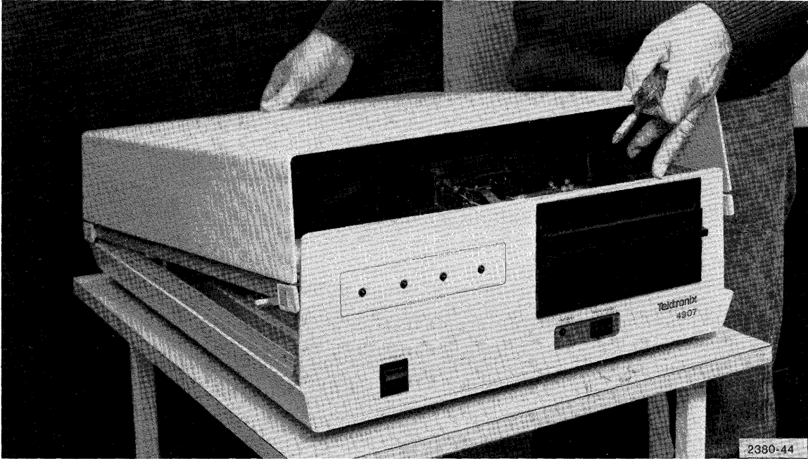
Figure E-3. Removing Main 4907 Cabinet Cover.
