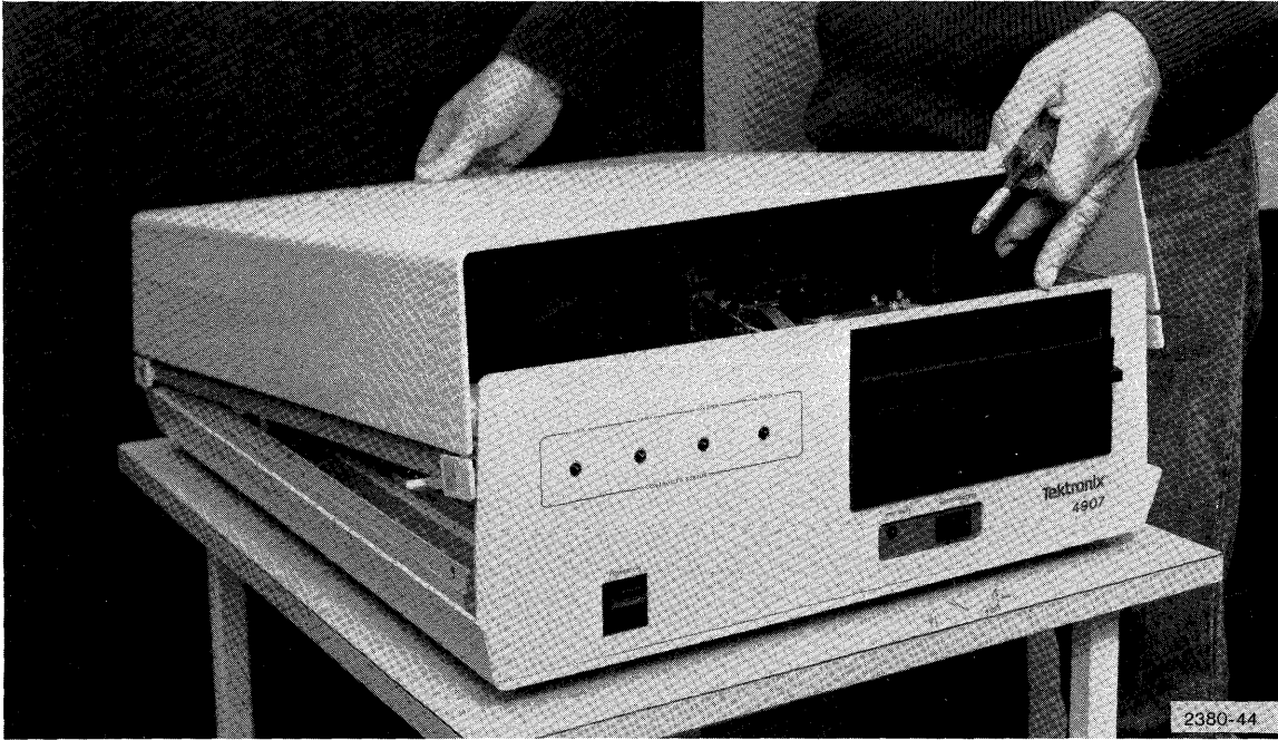
Figure E-1. Removing Main 4907 Cabinet Cover.
