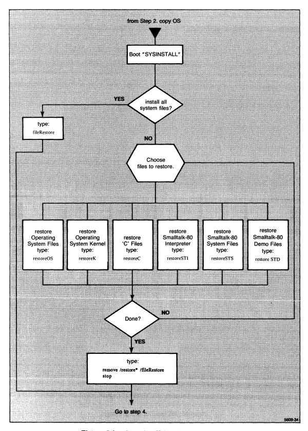
Figure 5-2. Step 1. Using DISKREPAIR.
