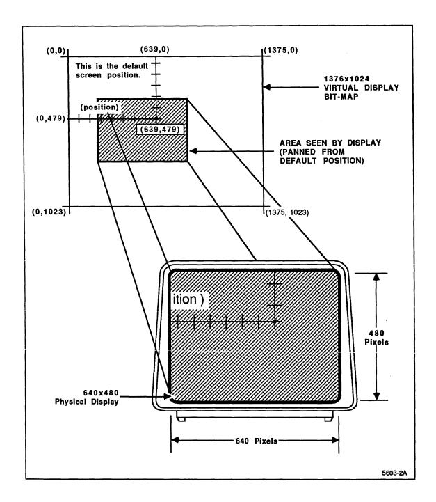
Figure 1-1. 640 X 480 Window Into 1376 X 1024 Bit-Map.
