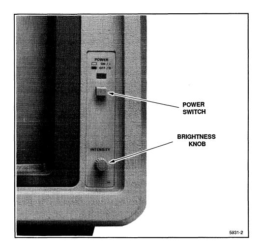
Figure 1-2. Display/CPU Front Panel Controls.
