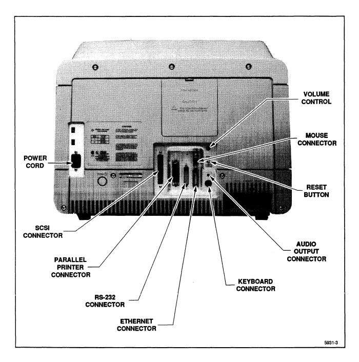
Figure 1-3. Display/CPU Rear Panel.
