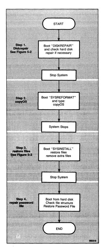
Figure 5-1. Non-Destructive System Rebuild Procedure.
