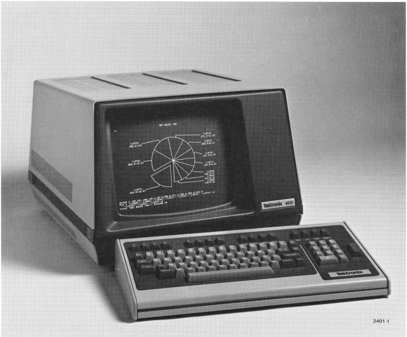
Fig. 1-1. 4025 Computer Display Terminal.
