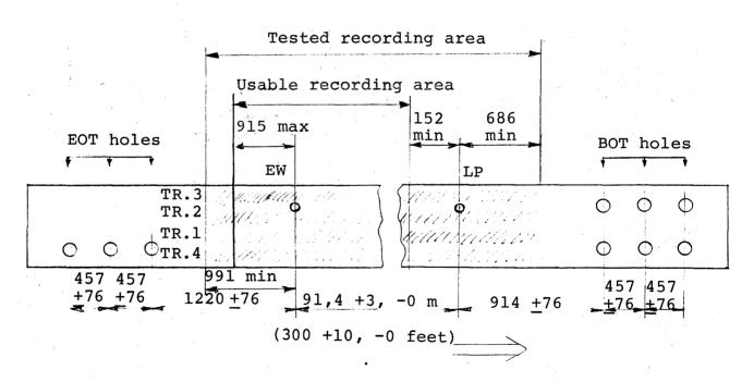
Dimensions in mmForward direction of tape travelexcept as noted(oxide side shown)
