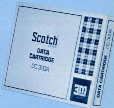
The Sykes Model TT140 Cartridge Recorder is an extremely reliable digital data storage device which incorporates the 3M DC300A quarter inch data cartridge.
