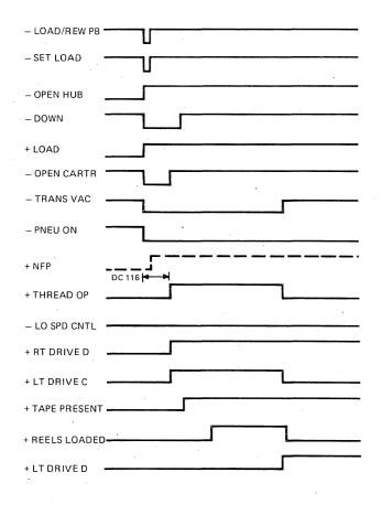
Figure 2-4. Thread Sequence Timing Chart
