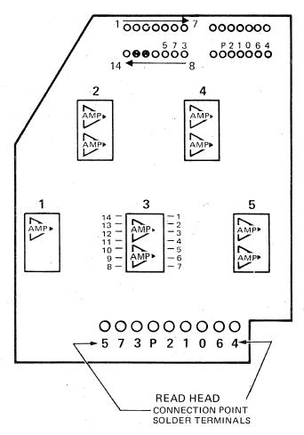
Figure 3-21. R/W Head Amplifier Card
