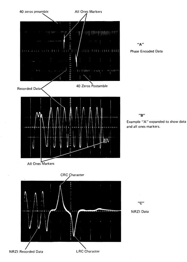
Figure 4-15. Scope View of Recorded Data
