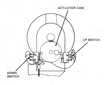
Figure 4-28. Power Window Switches
