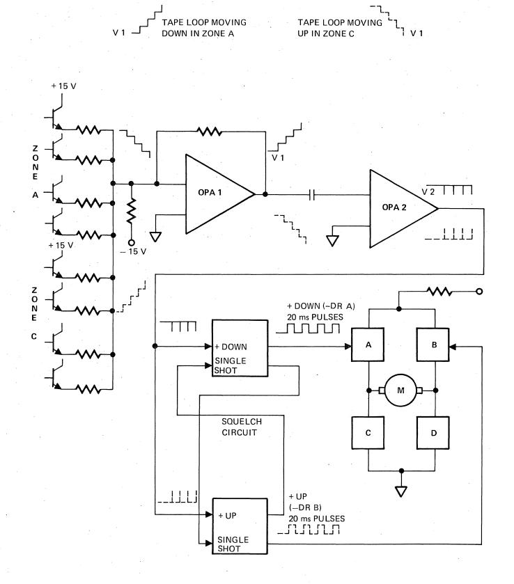
Figure 3-7. Velocity Feedback Control
