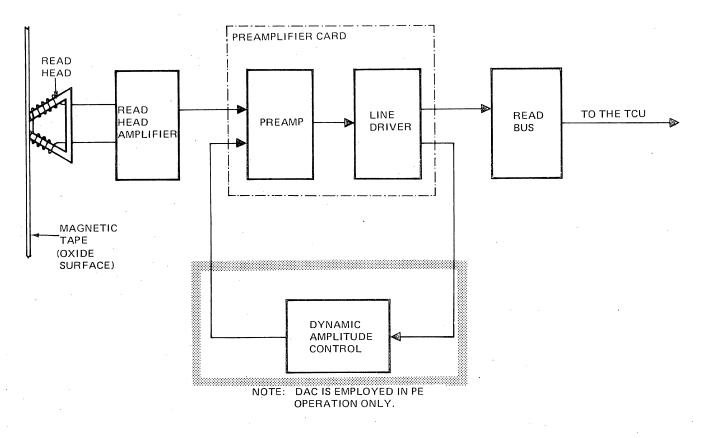
Figure 3-20. Read Circuit Simplified
