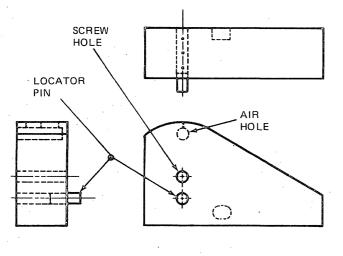
Figure 4-18. Right Guide Assembly PE Only
