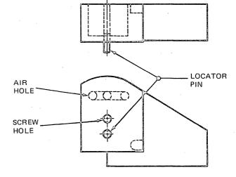
Figure 4-20. Right Guide Assembly (all DD except 3470)
