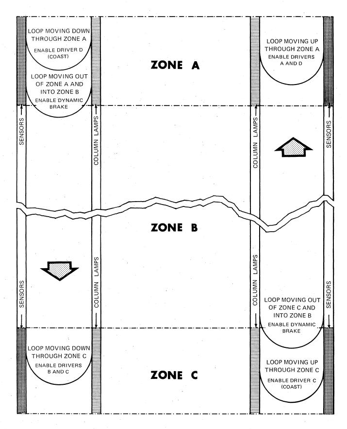
Figure 3-2. Column Sensors and Zones
