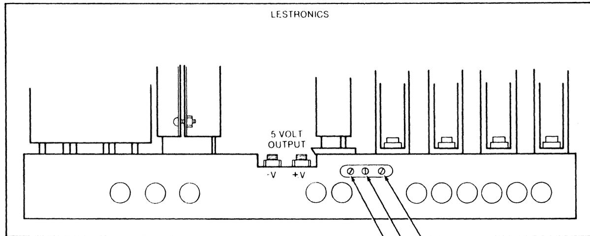
NOTE: Some power supplies have +15 and -15 volt adjustment potentiometers reversed and mislabeled. ADJUST WITH CARE!
