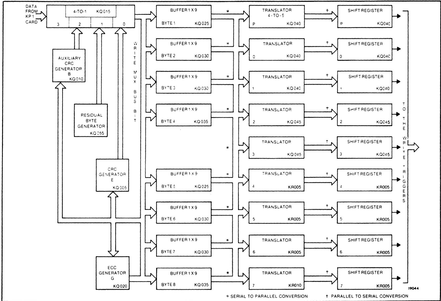
Figure 5-7. Write Data Path (GCR Only)
