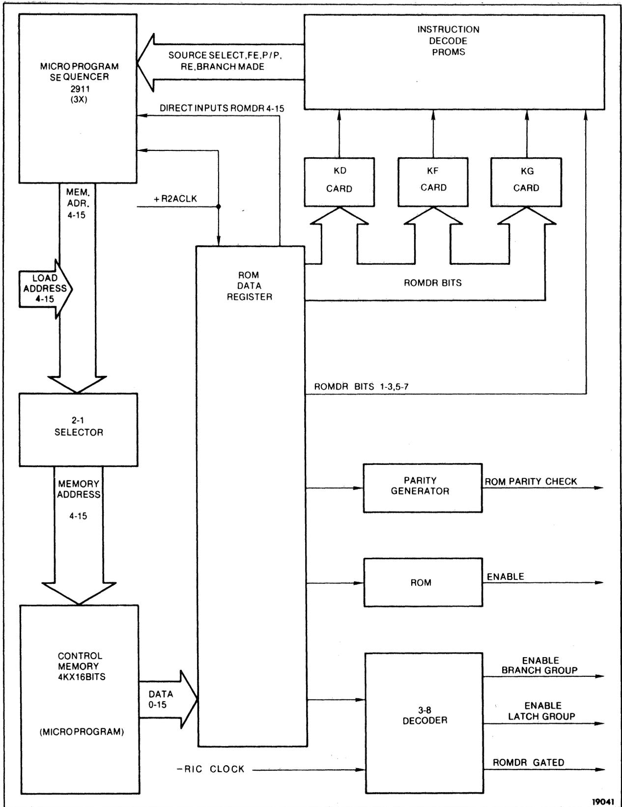
Figure 5-2. Microcontroller Block Diagram
