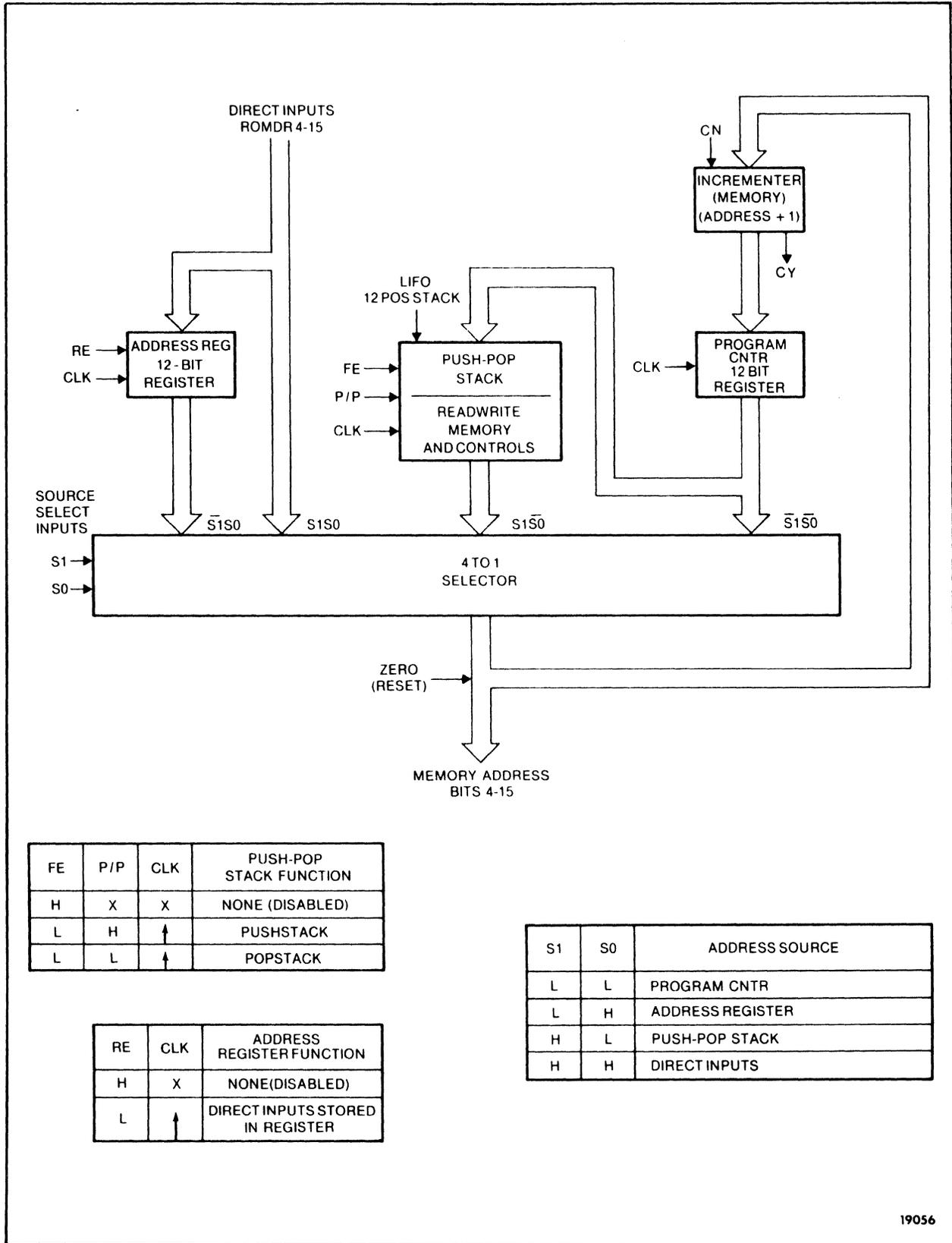
Figure 5-3. Microprogram Sequencer Block Diagram
