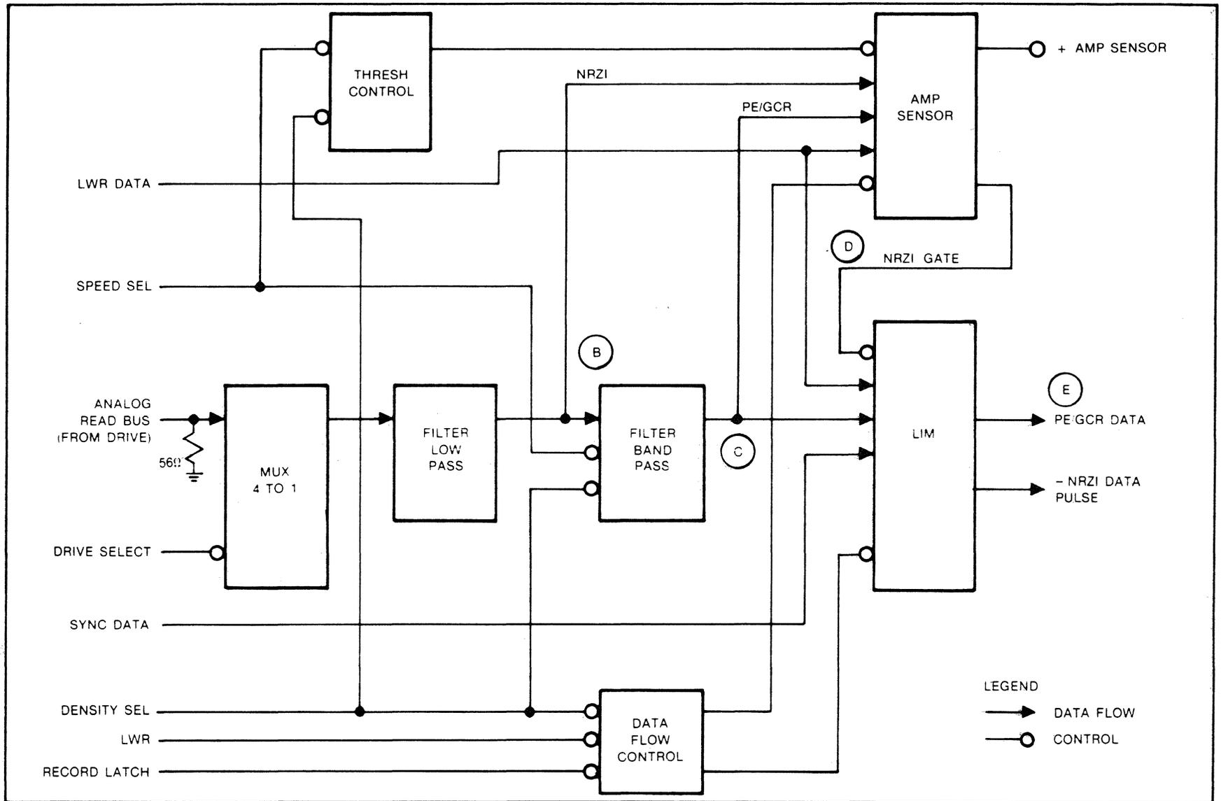
Figure 5-9. Read Analog-to-Digital Conversion (One Track)
