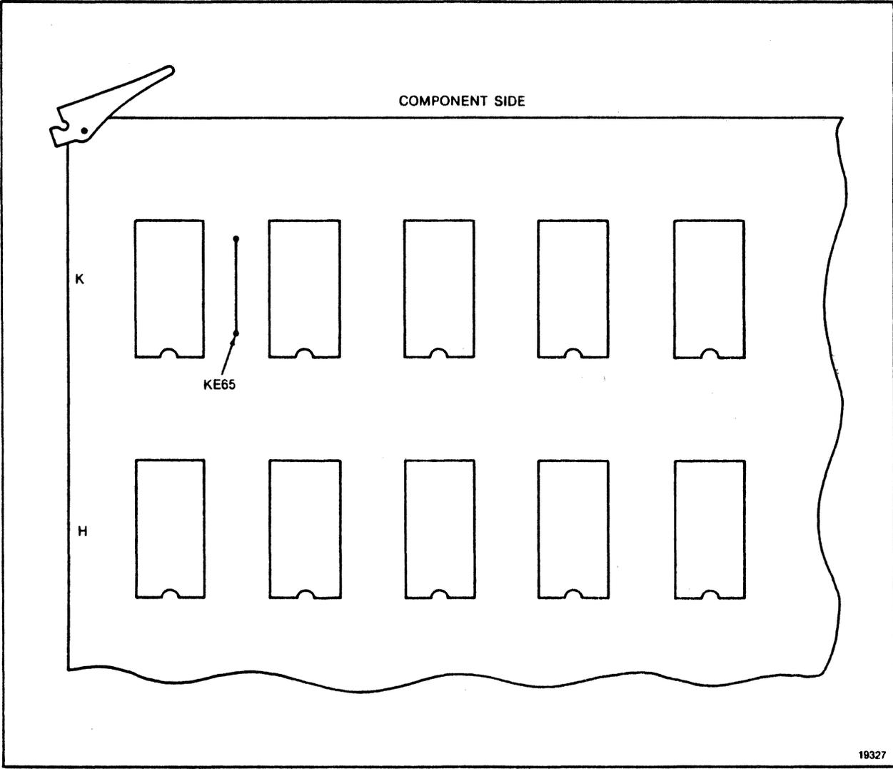
Figure 2-7. KG Card Jumper Location
