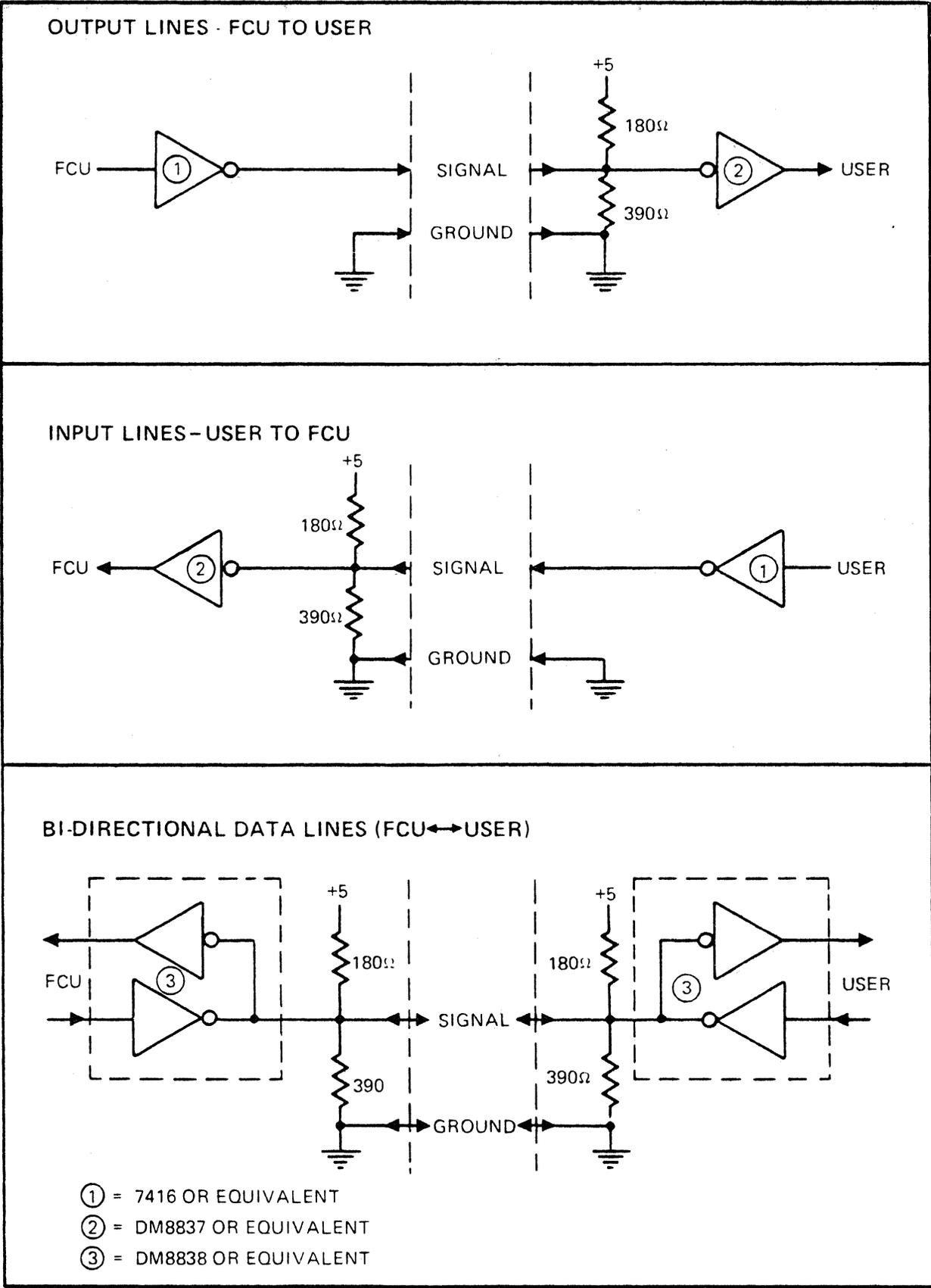
Figure 3-1. FCU-USER Interface Circuits
