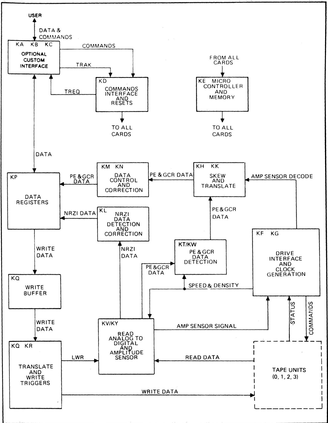
Figure 5-1. FCU Functional Block Diagram
