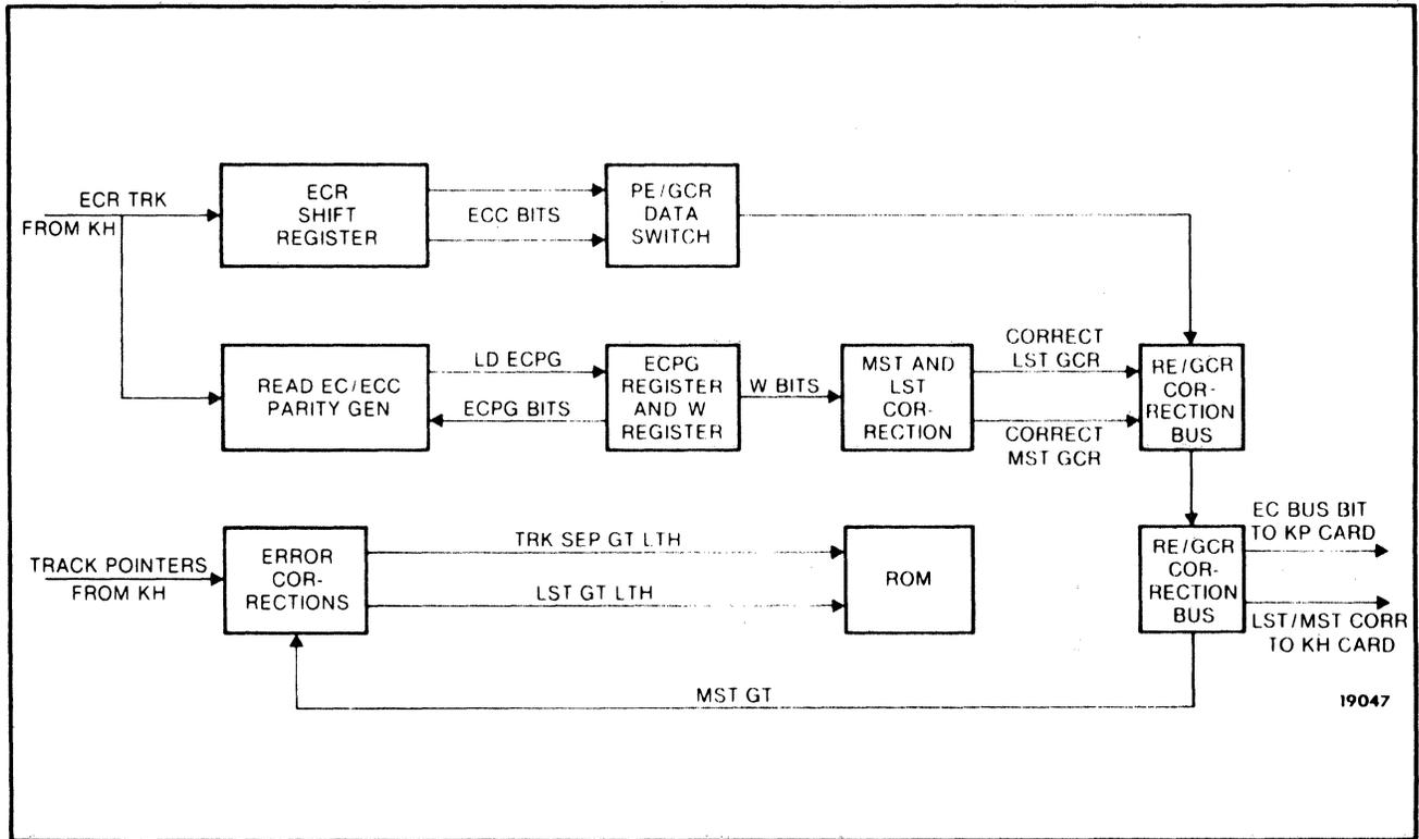
Figure 5-12. PE/GCR Read Data Path (KM Card)
