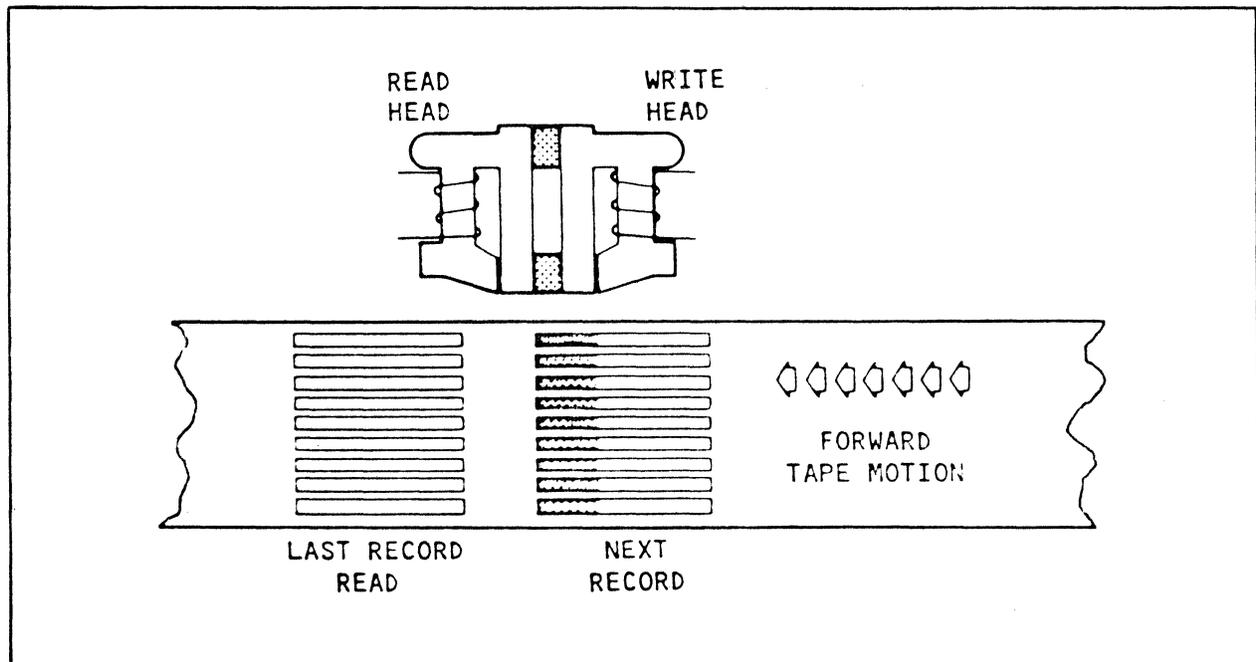
Figure 3-3. Read Forward/Write Partial Record Problem
