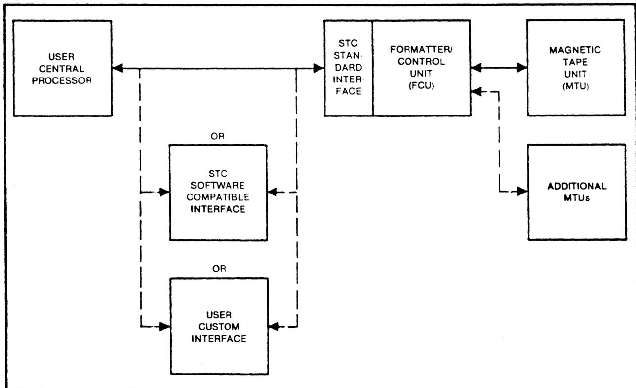
Figure 1-2. Tape Subsystem Configuration
