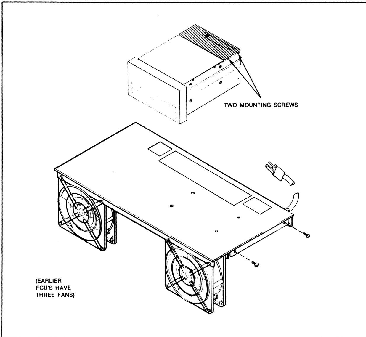
Figure 6-4. Cooling Fan Replacement
