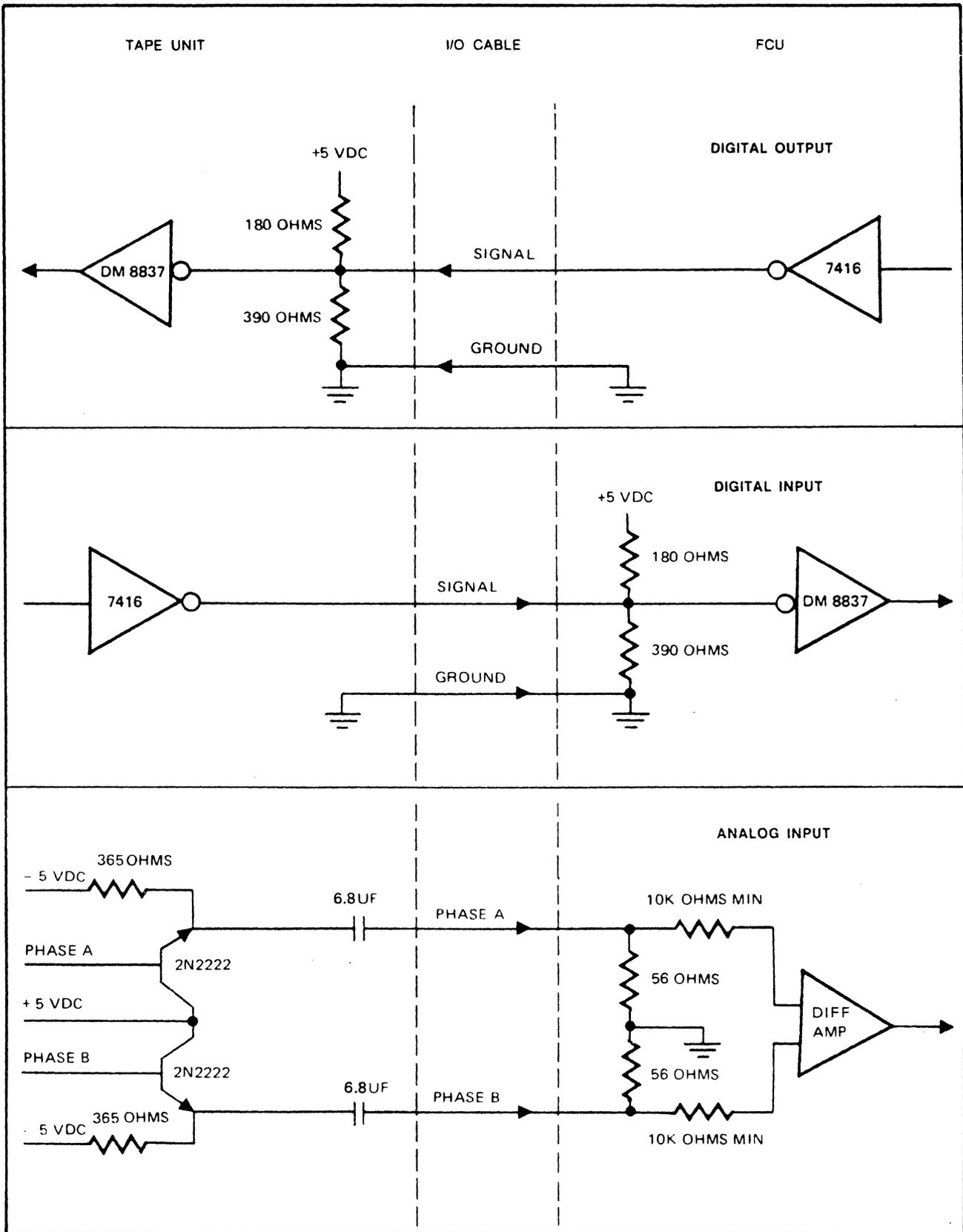
Figure 4-1. FCU/TU Interface Circuits
