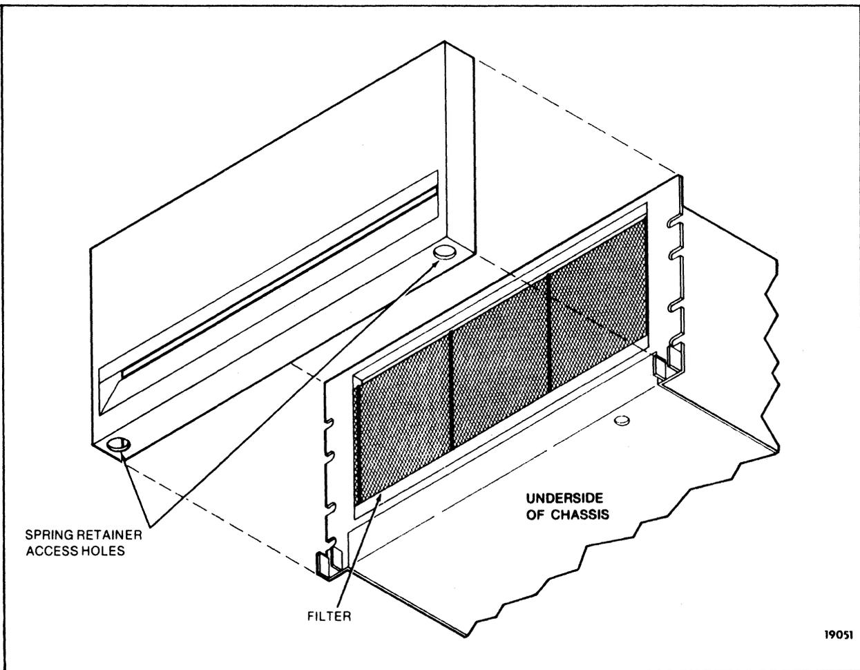
Figure 6-3. Filter Removal
