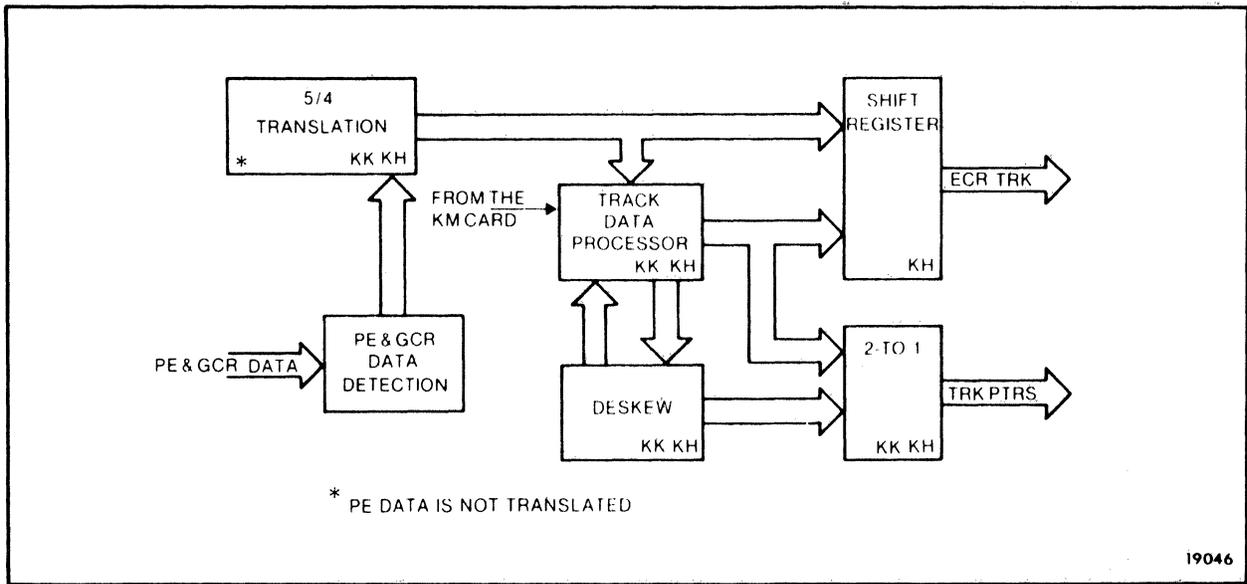
Figure 5-11. PE/GCR Read Detection
