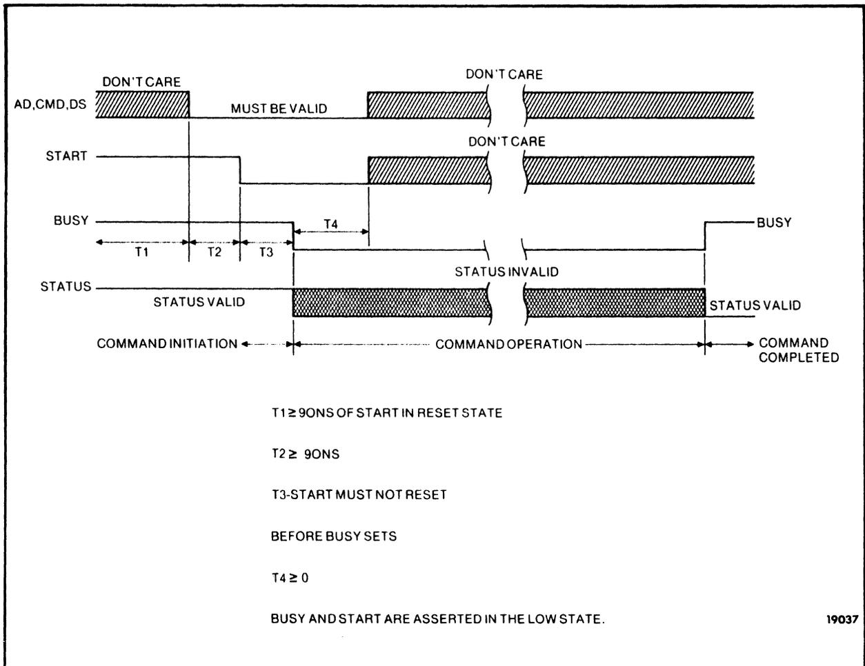
Figure 3-2. Command Initiation, Operation, and Completion
