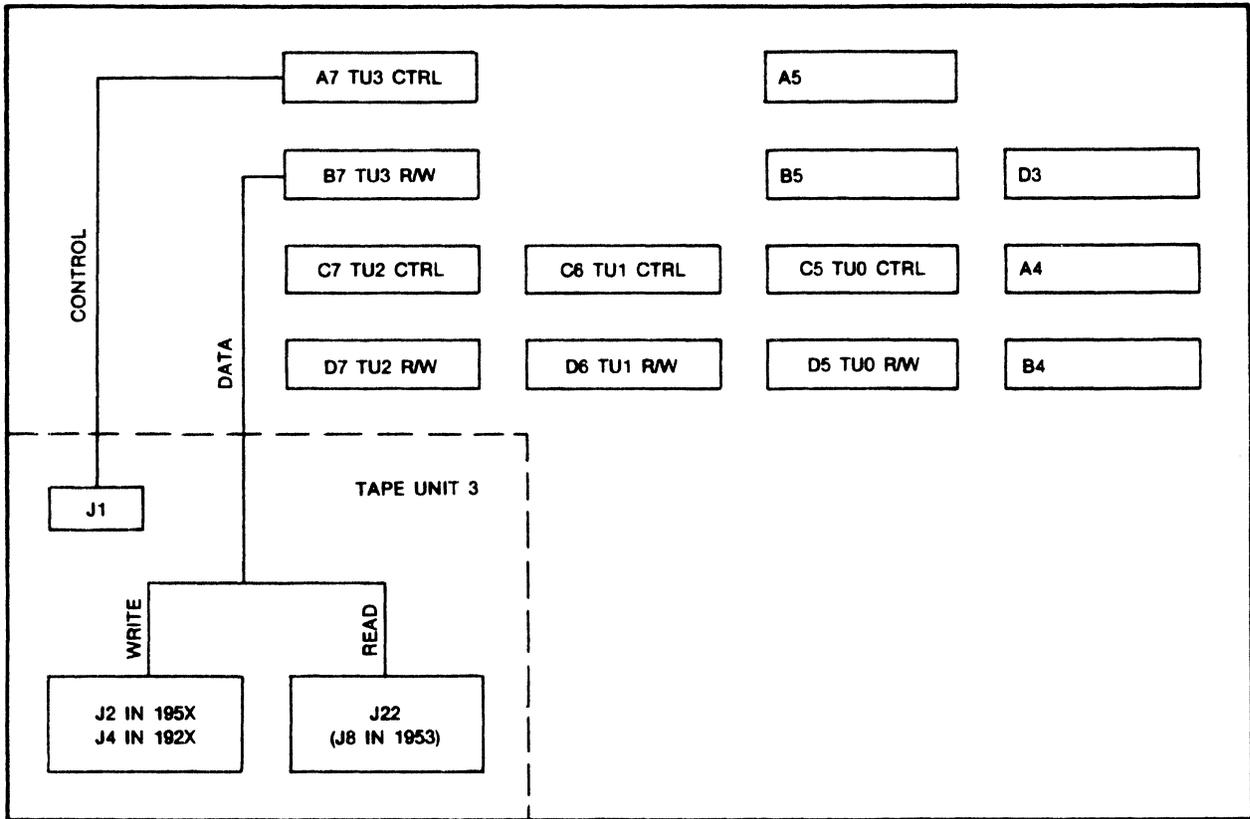
Figure 2-4. FCU/TU Interface Cable Connection
