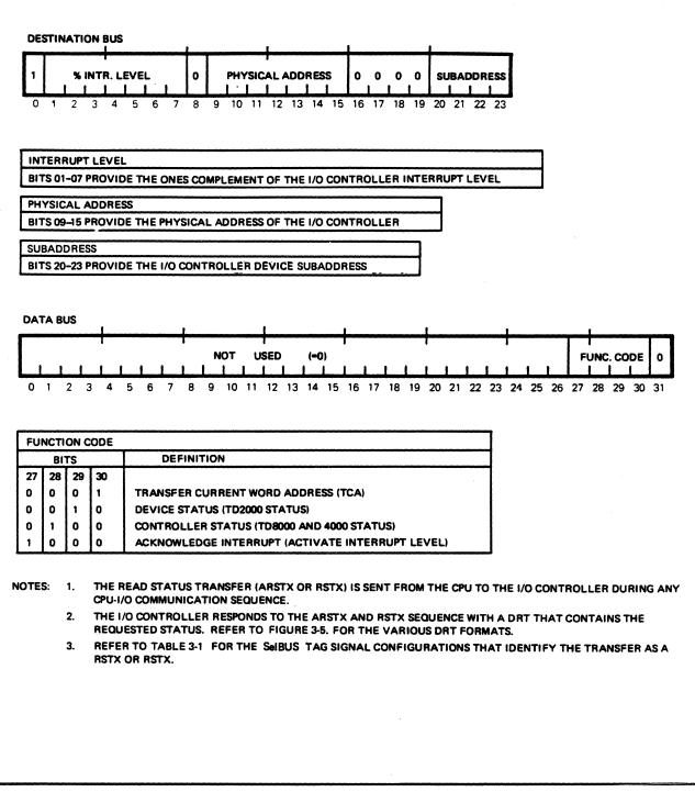
Figure 3-4. Advance Read Status Transfer (ARSTX) and Read Status Transfer (RSTX) Formats
