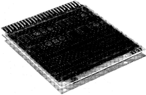
The ZT37 Breadboard Module has a versatile etch circuit pattern arranged for convenient mounting of all standard components, including diodes, capacitors, resistors, transistors or IC's in TO-5 cans, flat packs, or the 14-lead or 16-lead dual-in-line package. This module permits custom building of special circuits while retaining the advantages and mechanical compatibility of J Series etch circuit construction.
