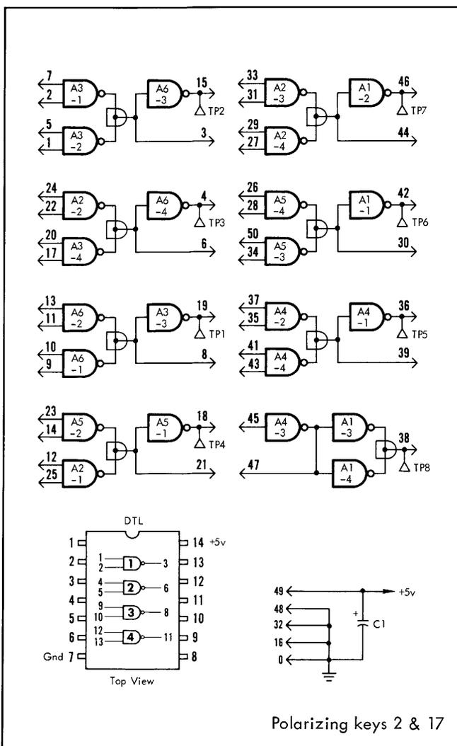
The LJ16 module contains a 4-bit parallel binary full-adder with ripple carry between stages. The module also contains four 2-input NANDs which permit the adder to be used with single-ended (True input only) data signals. The NANDs can be used for other logic functions if not needed at adder input. Refer to logic diagrams 1 and 2, and schematic diagram.
