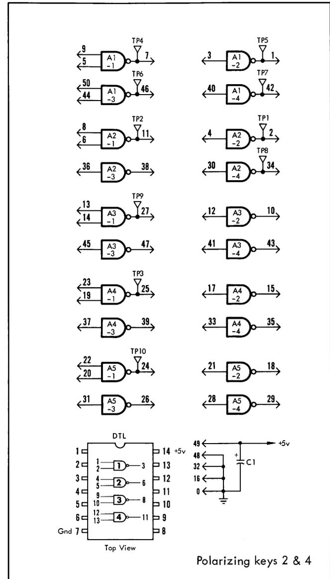
The IJ13 module contains sixteen power NANDs arranged in pairs with a strobe input common to each pair. Two independent 2-input power NANDs are also provided. Type 944 DTL power gates are used, with an external 1.1K ohm (3 unit load) pull-up resistor connected to each gate output.
