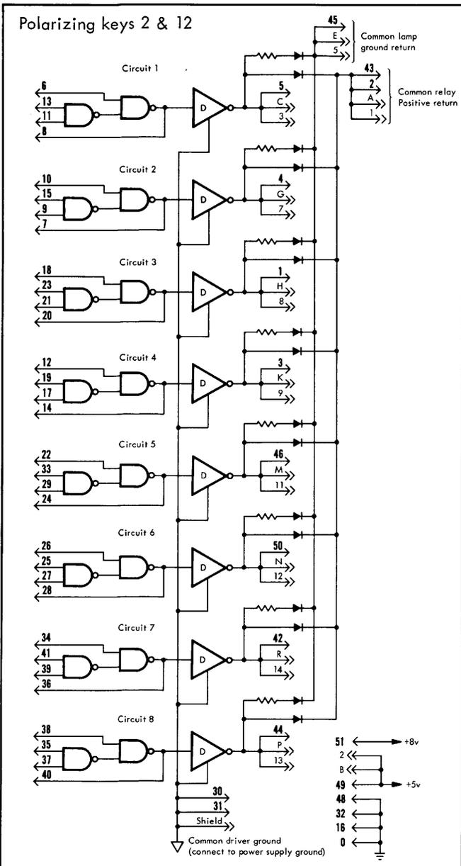
for an ET11 connector to permit routing of outputs to remote lamps or relays. (The single connector symbols indicate back panel contacts).
