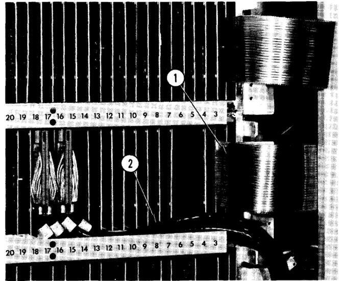
The ZT52 wire used to interconnect backpanel wire wrap pins has two special mechanical features. The insulation is especially tough, to resist cold flow; and, the copper conductor has the proper tensile strength to provide a firm wrap without loosening the pin. Electrically, the wire behaves as a 150-ohm transmission line, when pushed close to the ground plane that is built into all SDS mounting cases. The ground plane protects the signal.
