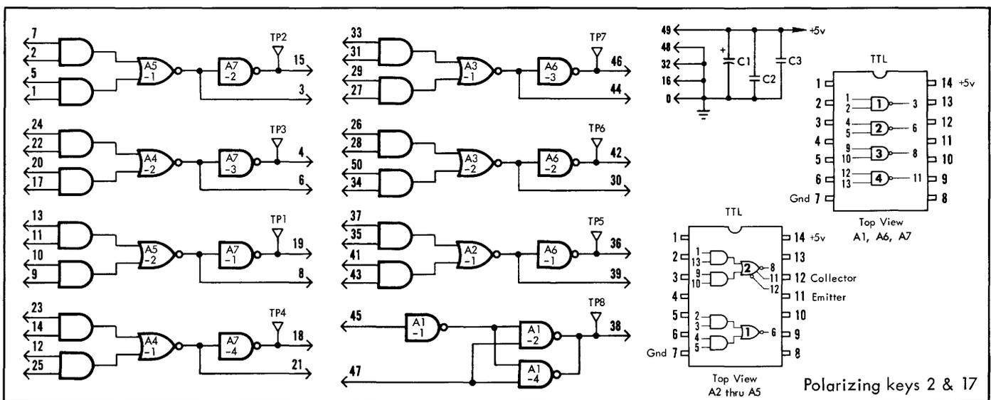
The LJ66 module contains a 4-bit parallel binary full-adder with ripple carry between stages. The module also contains four 2-input NANDs which permit the adder to be used with single-ended (True input only) data signals. The NANDs can be used for other logic functions if not needed at adder input. Refer to logic diagrams 1 and 2, and schematic diagram.
