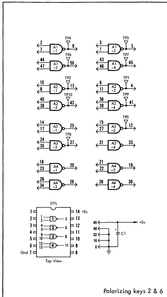
The IJ11 module contains six 4-input NAND gates and four 3-input NAND gates, which perform the function  $Q = \overline{ABCD}$  and  $Q = \overline{ABC}$  respectively. An unwired input functions as if it were wired True.
