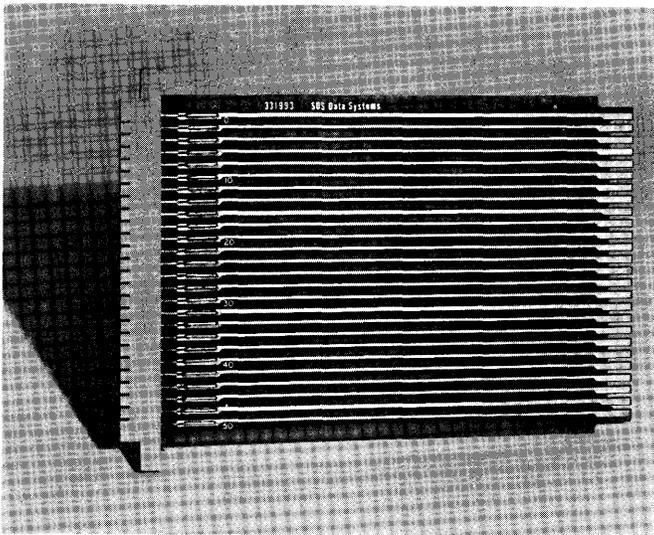
The ZT53 Extender Module has a straight-through etched circuit pattern and a VT12 connector mounted on its front edge. It permits the user to extend any module in front of the rack so that circuit operation may be investigated while the module is plugged into the system. Contacts are Rhodium plated for long life. ZT53 has polarizing slots in all positions.
