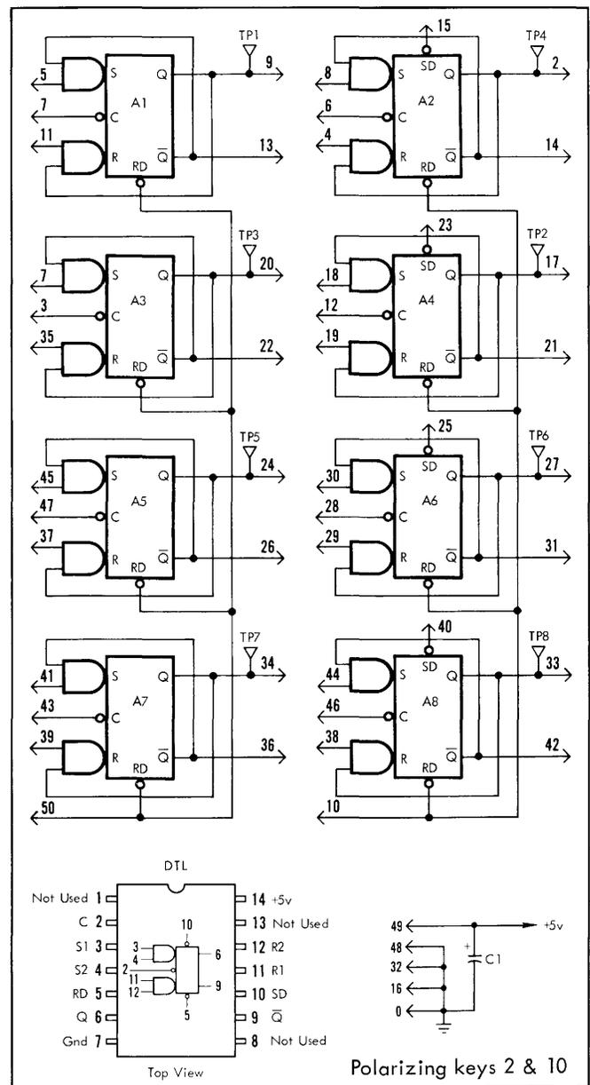
The FJ11 contains four JK flip-flops and gating to permit operation as a 4-bit synchronous binary up-counter, a 4-bit synchronous binary down-counter, a 4-bit right-shift register, or a 4-bit left-shift register.
