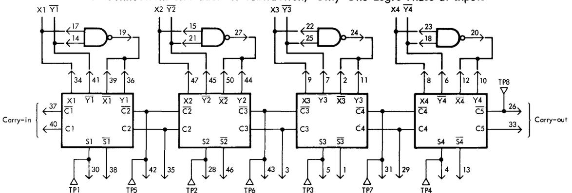
Note:  $S$  = sum.  $X$  and  $Y$  are the bits to be added.  $C1$  is carry-in.  $C2$  is carry-out of first stage and carry-in to second stage.  $C3$  is carry-out of second stage and carry-in to third stage.  $C4$  is carry-out of third stage, and carry-in to fourth stage.  $C5$  is carry-out of adder.  $A$  and  $B$  are independent NAND gate inputs, and  $G$  is NAND gate output (see schematic diagram on next page).
