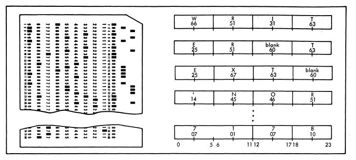
Figure 9. Card Read Into Memory in Hollerith
