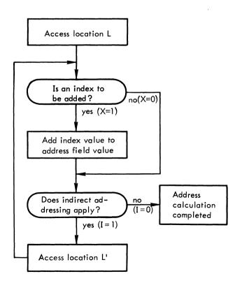
Figure 4. Effective Virtual Address Calculation
