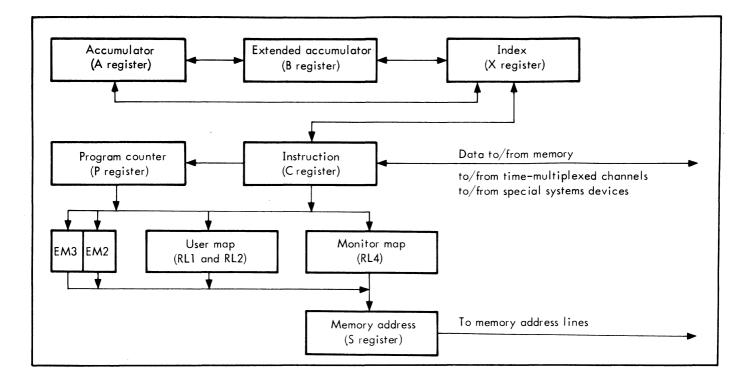
Figure 2. Basic 940 Register Flow Diagram
