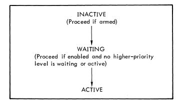
Figure 5. Interrupt Arm/Enable Response
