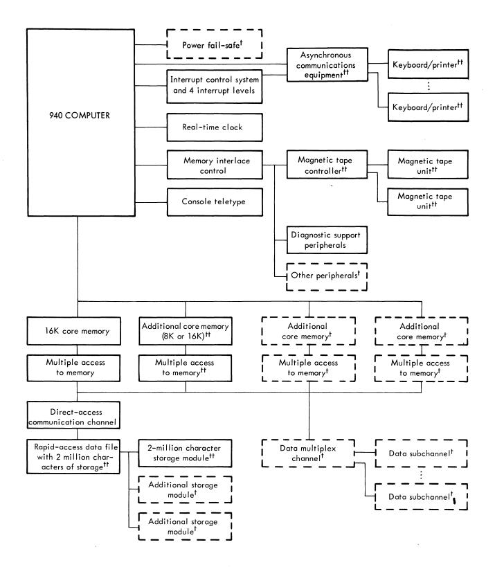
Figure 1. SDS 940 Time-Sharing Computer System
