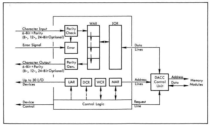
Figure 7. Typical SDS 940 Direct-Access Communication Channel, Block Diagram
