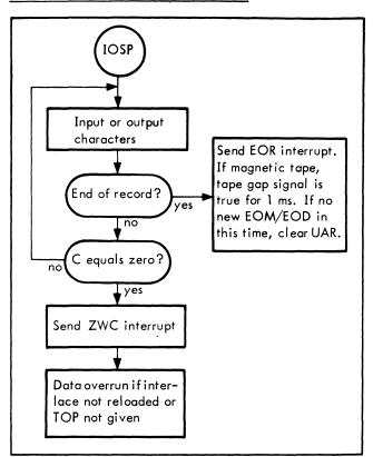
Input C Words. If the channel receives C words before the peripheral device encounters the end-of-record, the channel generates a zero word count interrupt (if armed). The program should reload the interlace portion of the channel to continue reading the record. Failure to reload the interlace before the peripheral device sends enough characters to overfill the word assembly register causes a character rate error; this sets the channel error indicator.
