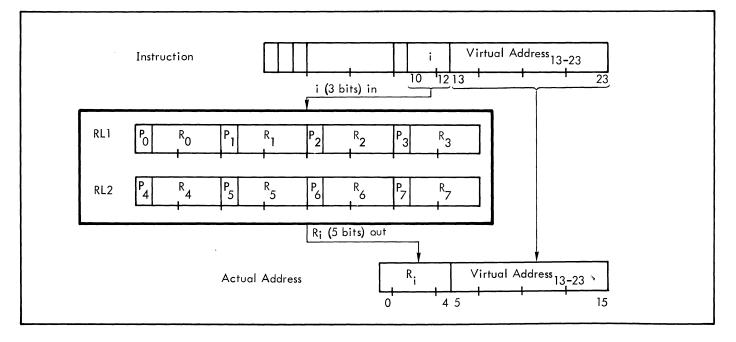
Figure 3. SDS 940 Mapping Process
