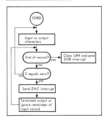
A program should not use the IORD function with devices that do not have end-of-record conditions on output (e.g., devices such as the paper tape punch and typewriter). These devices do terminate output but give the program no indication when they receive the last characters. Input C Words. If C words are received before the end-ofrecord is detected, the rest of the record is ignored. At the end-of-record, the peripheral device is disconnected and the channel becomes inactive.
