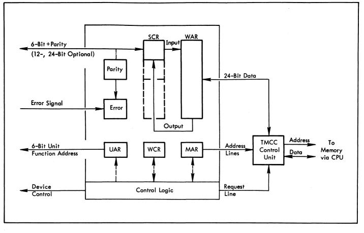
Figure 6. Typical SDS 940 Time-Multiplexed Communication Channel, Block Diagram
