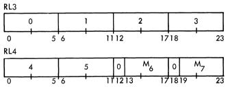
Actually, only the portions of the two registers labeled  $M_6$  and  $M_7$  are implemented with flip-flops. The other six registers may be thought of as though they permanently contained the following values:
