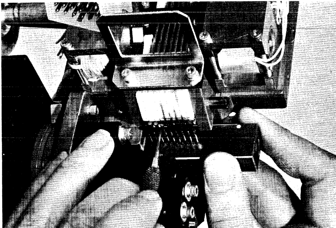
Figure 6-3. Punch Pin Alignment and Insertion Into Pin Driver.
