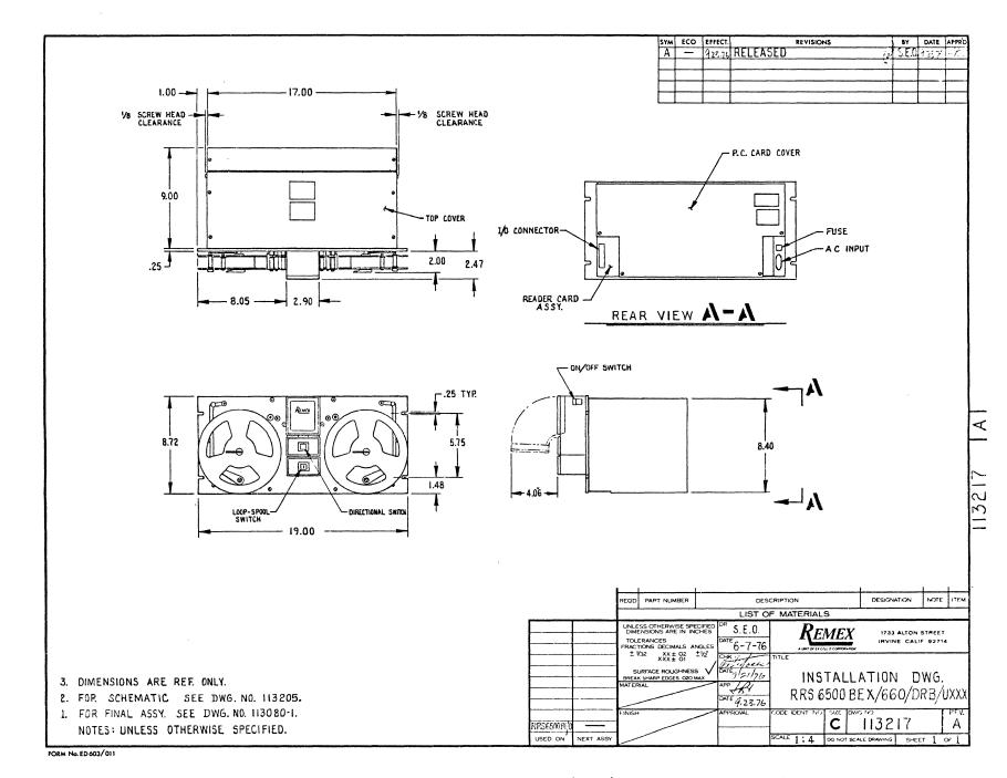
Figure 1-3. Installation Drawing, Model RRS6500BEX/66X/DRB. The dimensions for model RRS6500BEX/66X/ARB are identical except the 2.00 is 2.51, the 8.72 is 10.47 and the 5.75 is 7.50.
