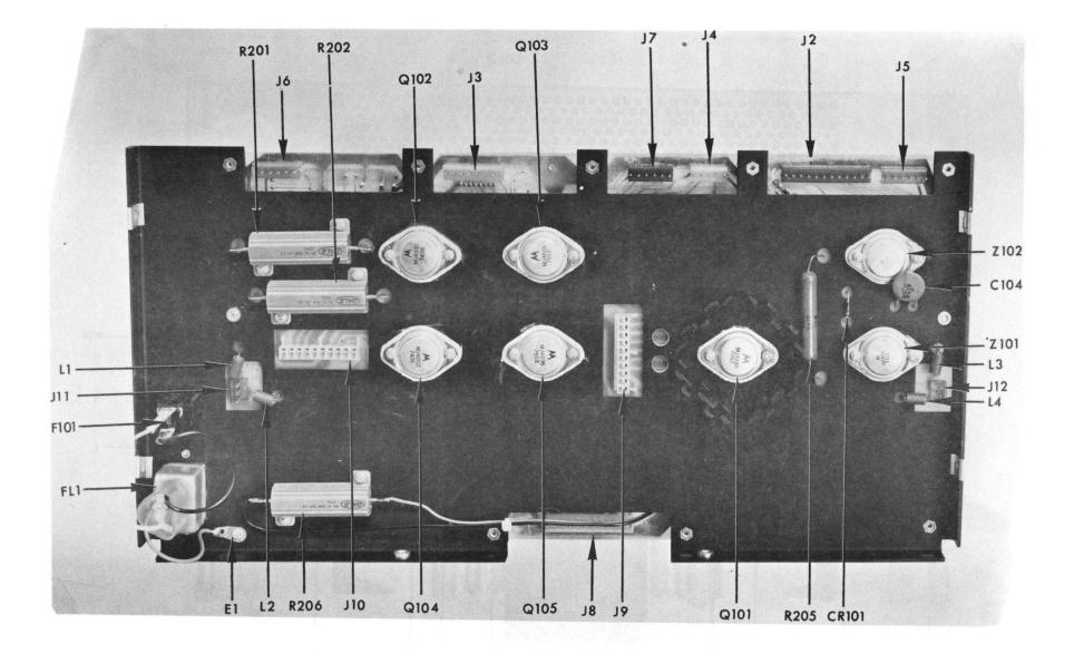
Figure 7-5. Power Driver Panel Assembly 111021-3.
