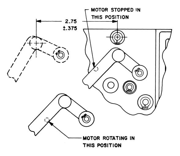
**MMC 501** Figure 5-6. Switch Actuation Points for the Left Arm.
