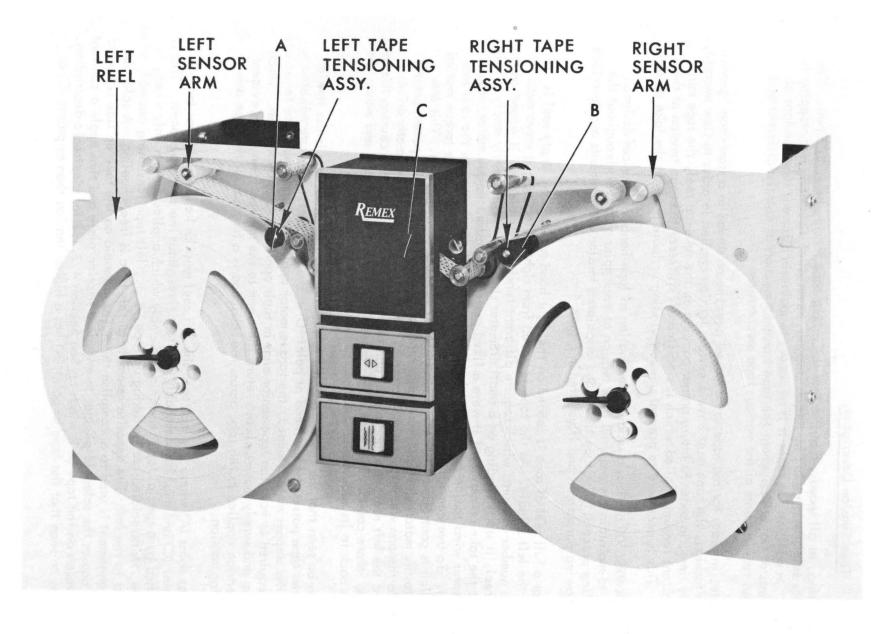
Figure 4-6. Front View Showing Various Points of Tape Tension.
