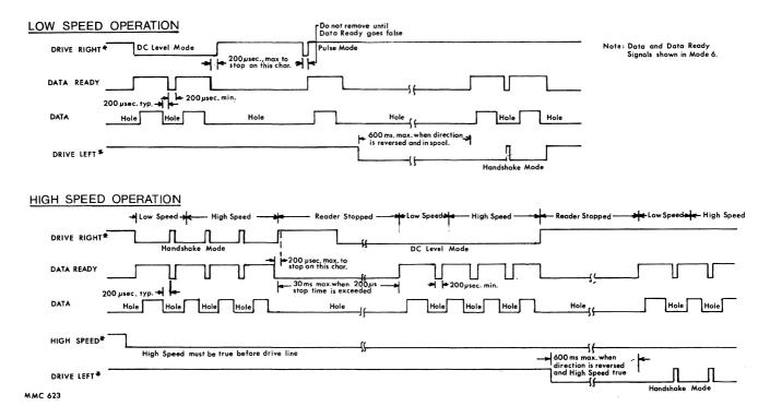
Figure 3-1. Timing Diagram for RRS6500.
