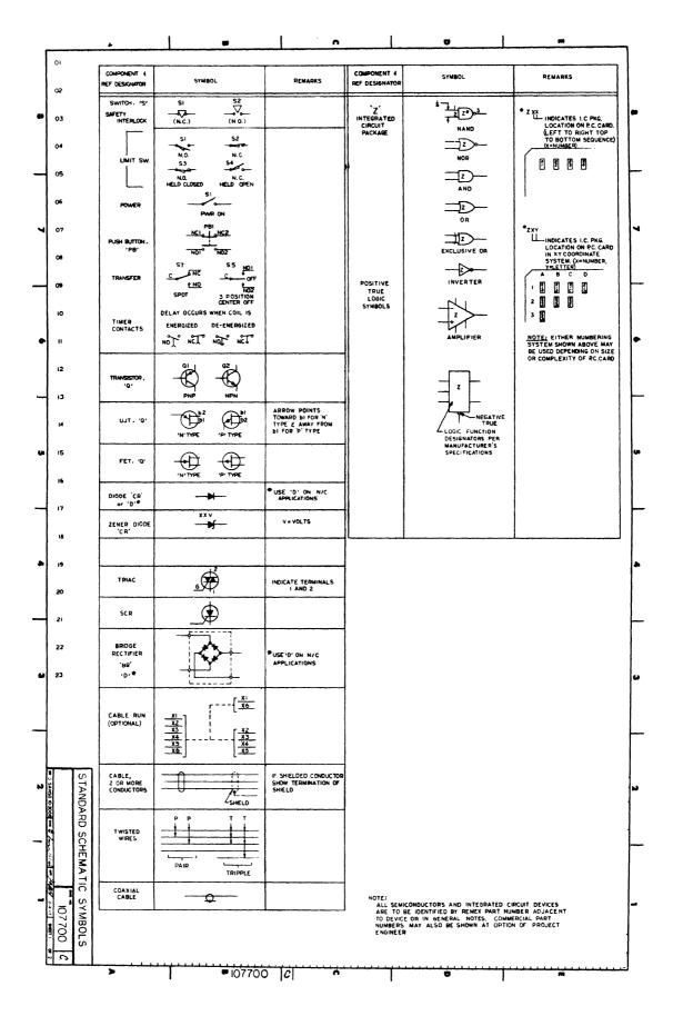
Figure 8-4. REMEX Standard Schematic Symbols (Sheet 1 of 2)
