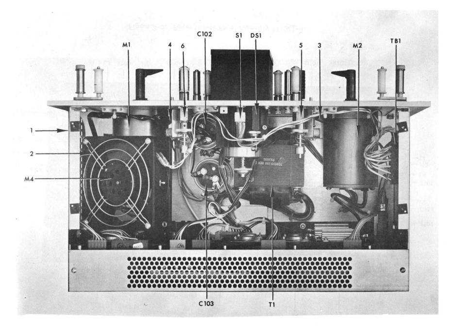
Figure 7-4. Rear View of Front Panel, RRS6500BEX/660/ARB. The location of components on the RRS6500BEX/660/DRB is approximately the same.
