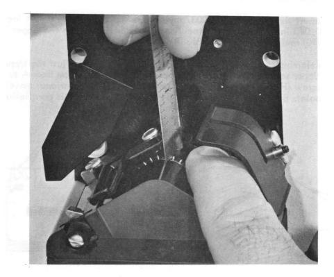
Figure 5–2. Setting of the Sprocket in Relation to the Tape Riding Surface.
