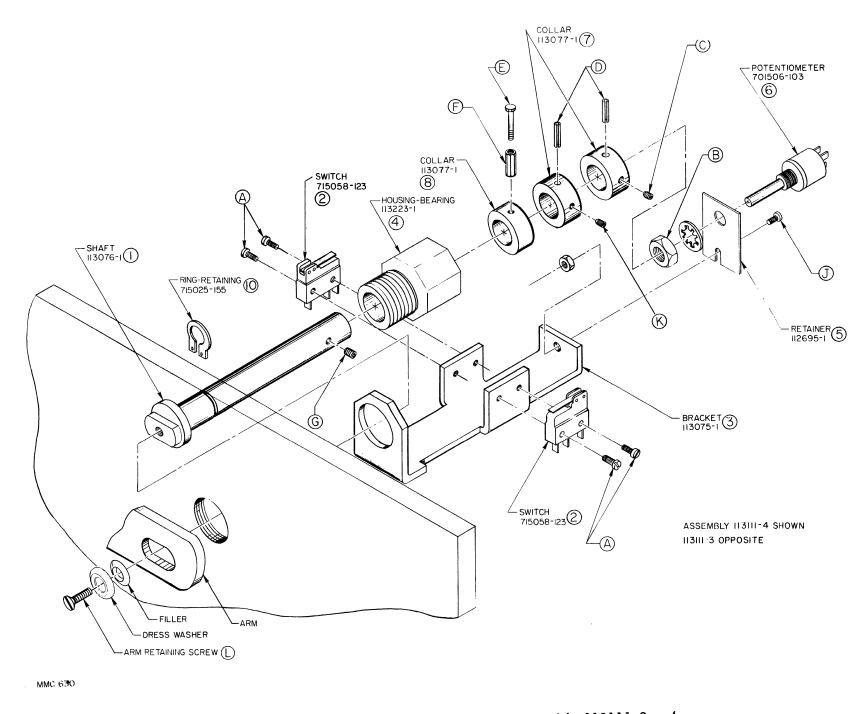
Figure 6-1. Exploded Drawing of Tape Break Switch Assembly 113111-3, -4.
