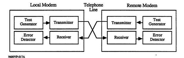
Figure 7-5. End-to-End Self-Test
