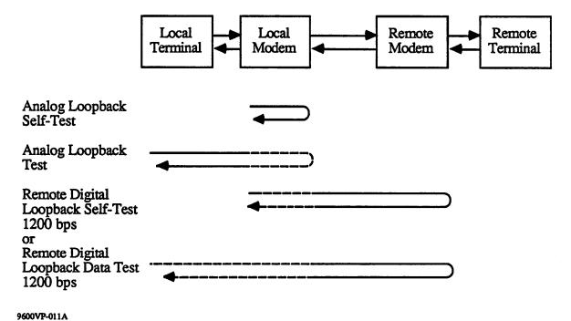
Figure 7-2. Test Sequence without a Remote Operator
