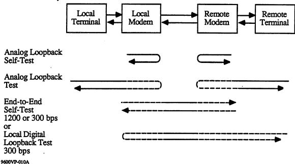
Figure 7-1. Test Sequence with a Remote Operator
