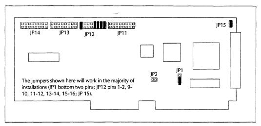
Figure 3-1 Host Adapter (UltraStor 14F) Jumper Installation
