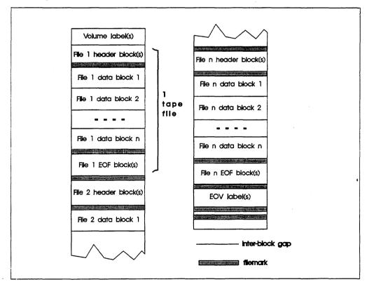
Figure 19-1 Standard Labeled Tape Format
