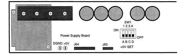
Figure 10-10 +5 Volt Regulator Adjustment Location
