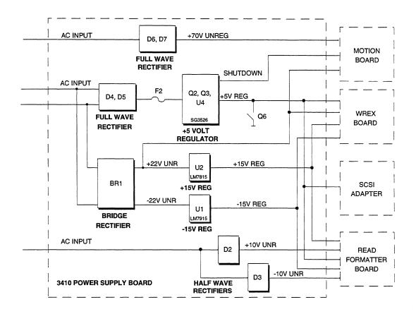
Figure 4-3 Power Supply Block Diagram
