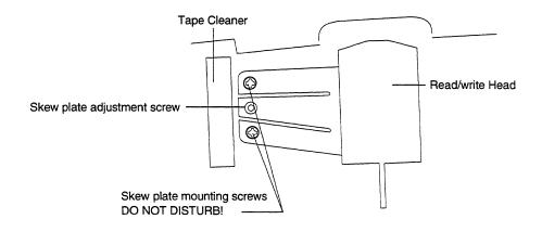
Figure 10-8 Adjustable Skew Plate
