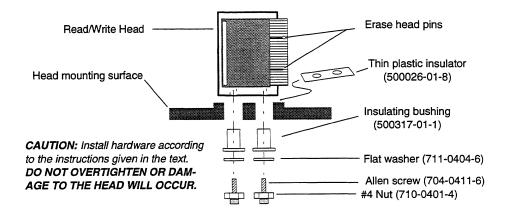
Figure 9-6 Head Installation Hardware
