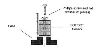
Figure 9-8 EOT/BOT Sensor Assembly Mounting
