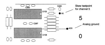
Figure 10-4 Skew Testpoints (500557 PCBA)
