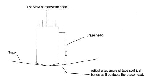
Figure 9-7 Tape/Erase head contact.
