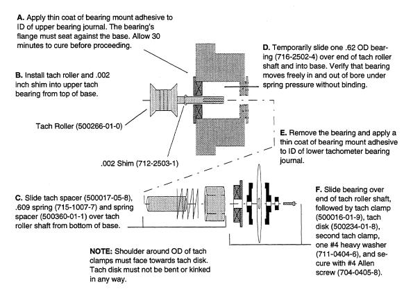
Figure 11-2 Tachometer Bearing Installation
