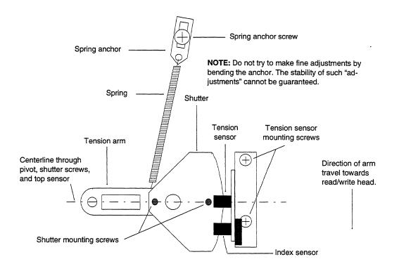
Figure 10-9 Tension Arm Adjustment Components
