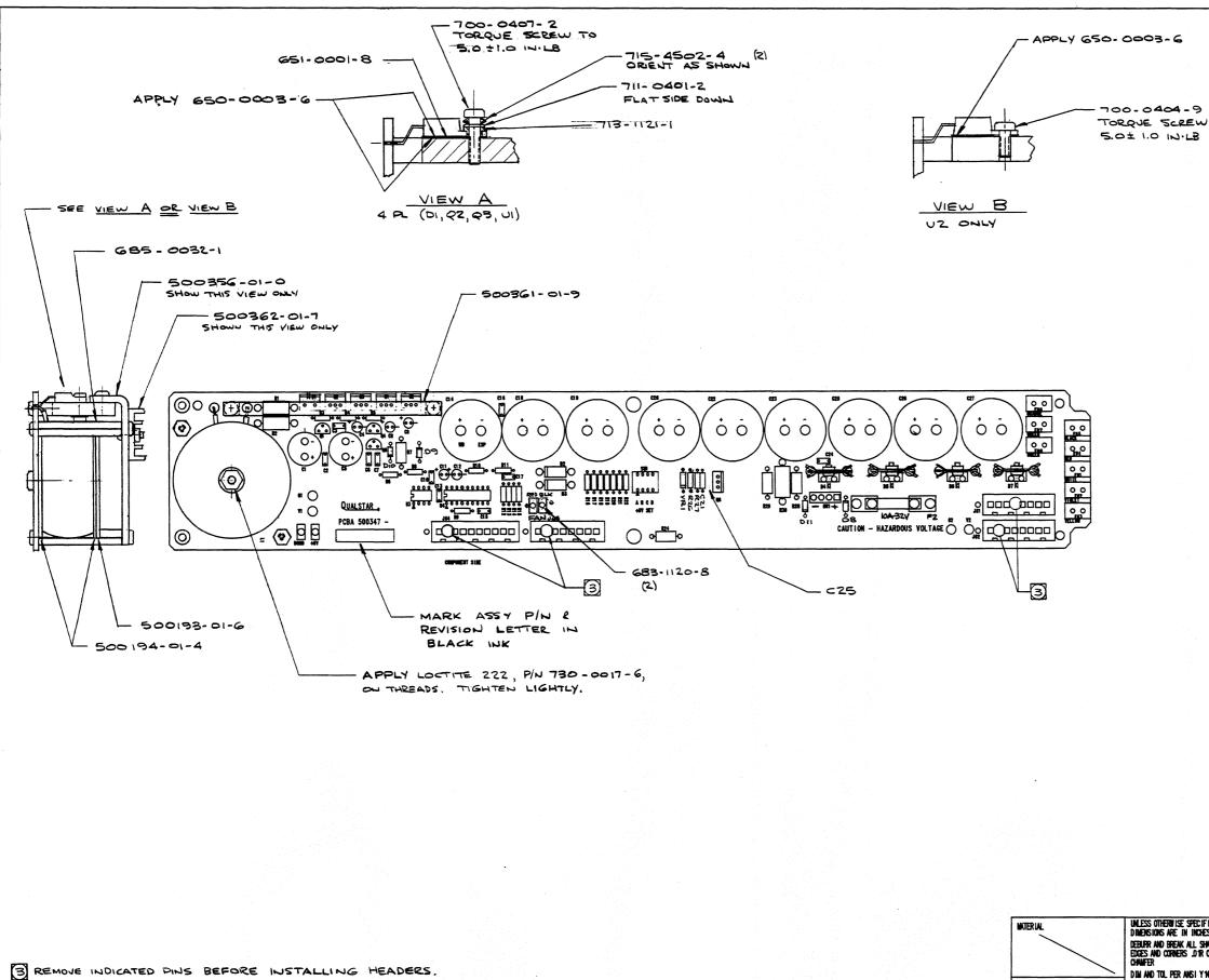
2. THIS BOARD IS MADE WITH 4 OZ COPPER. I. SEE LM FOR ASSY PIN. & REV NOTES: UNLESS OTHERWISE SPECIFIED
