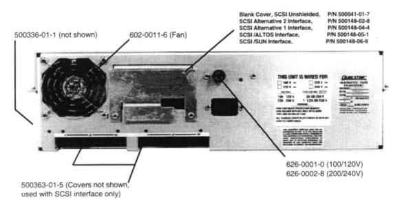
Figure 13-2 34XX Tape Drive, Rear View
