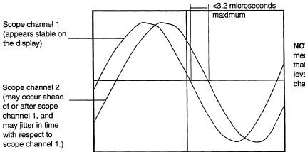
**NOTE:** Before making measurements, insure that the DC reference level of both scope channels are the same.
