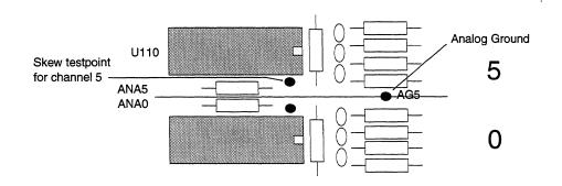
Figure 10-3 Skew Testpoints (500497 PCBA)
