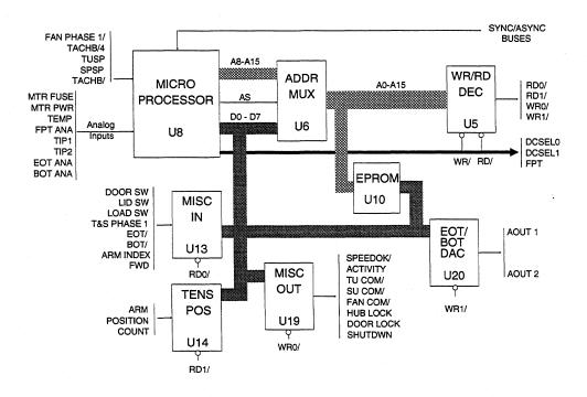
Figure 4-1 Motion Board Microcomputer Block Diagram
