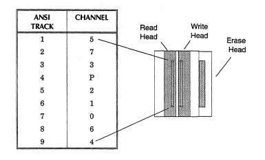
Figure 10-7 Track layout as seen from face of head
