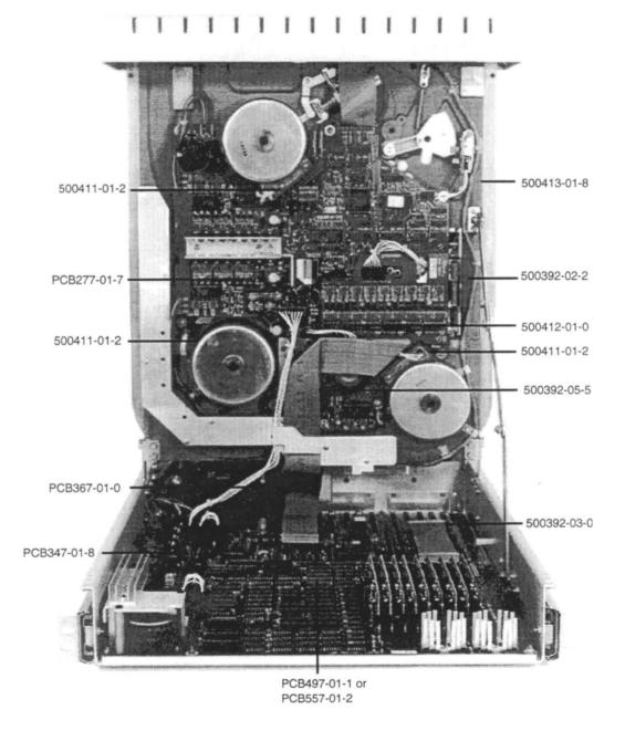
Figure 13-3 3410/3412 Internal Component Locations
