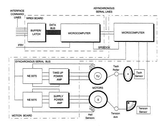
Figure 4-2 Motor Control Block Diagram
