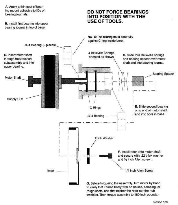
Figure 11-1 Motor Bearing Replacement Instructions
