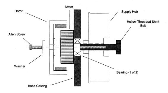
Figure 9-9 Typical Motor Assembly
