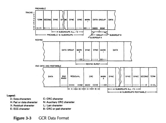
detect and track the data fields. Although the 3410/3412 tape drive records all control subgroups per ANSI specifications, not all of the control subgroups are required by the read recovery circuits.
