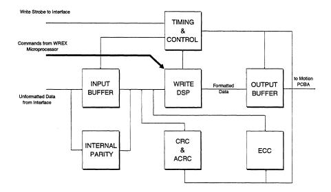
Figure 5-1 Write Formatter Block Diagram
