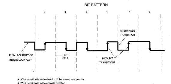
Figure 3-1 PE Data Bit Pattern
