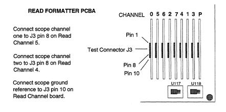
Figure 10-2 Skew Testpoints (500377 PCBA)
