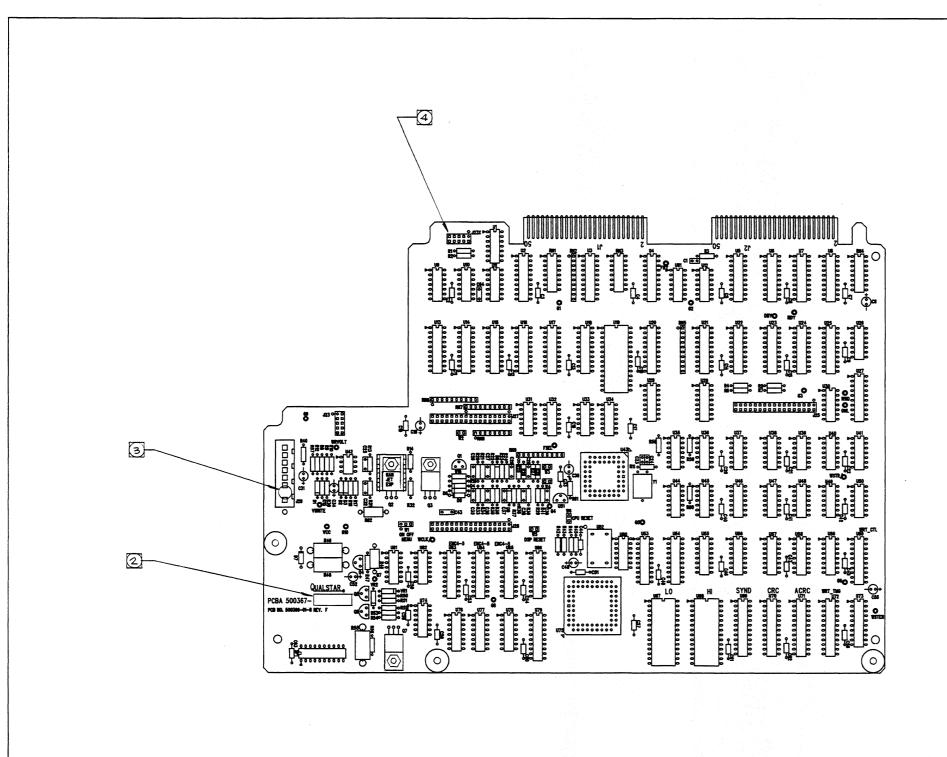
4 CONNECTOR PADS ARE FOR TEST ONLY, DO NOT INSTALL ANY CONNECTOR IN THIS LOCATION. 3 REMOVE PIN 2 BEFORE INSTALLING HEADER 2 MARK ASSY P/N AND REVISION LETTER IN BLACK INK.
