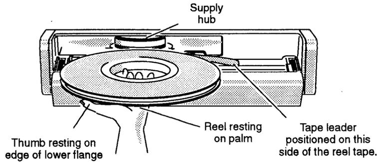
**Figure 3-5 Correct Way to Insert Reel**
