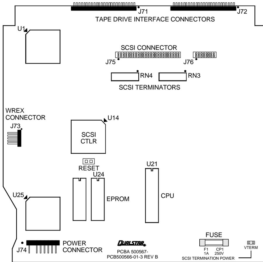
Figure 1-4 SCSI Single-Ended PCBA Layout – 500567 PCBA
