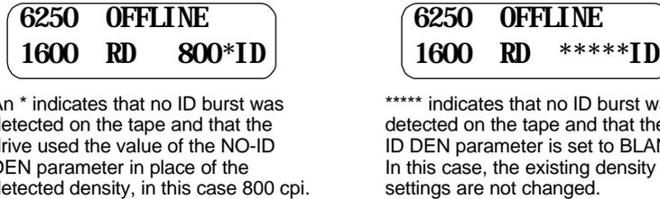
**Figure 3-10 Front panel display when no ID burst has been detected**
