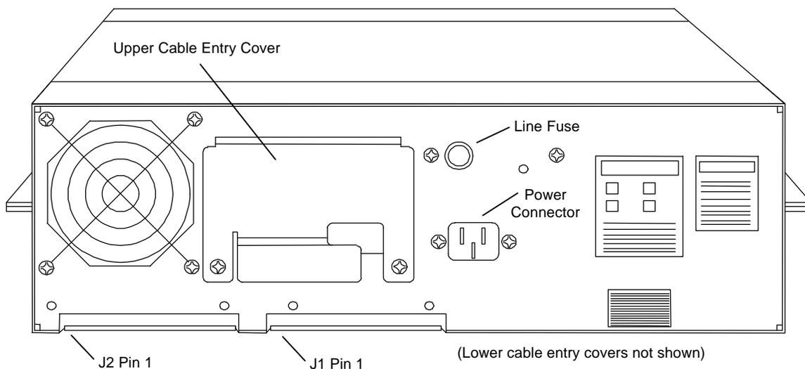
**Figure 1-10 Industry Standard Interface Connector Placement**
