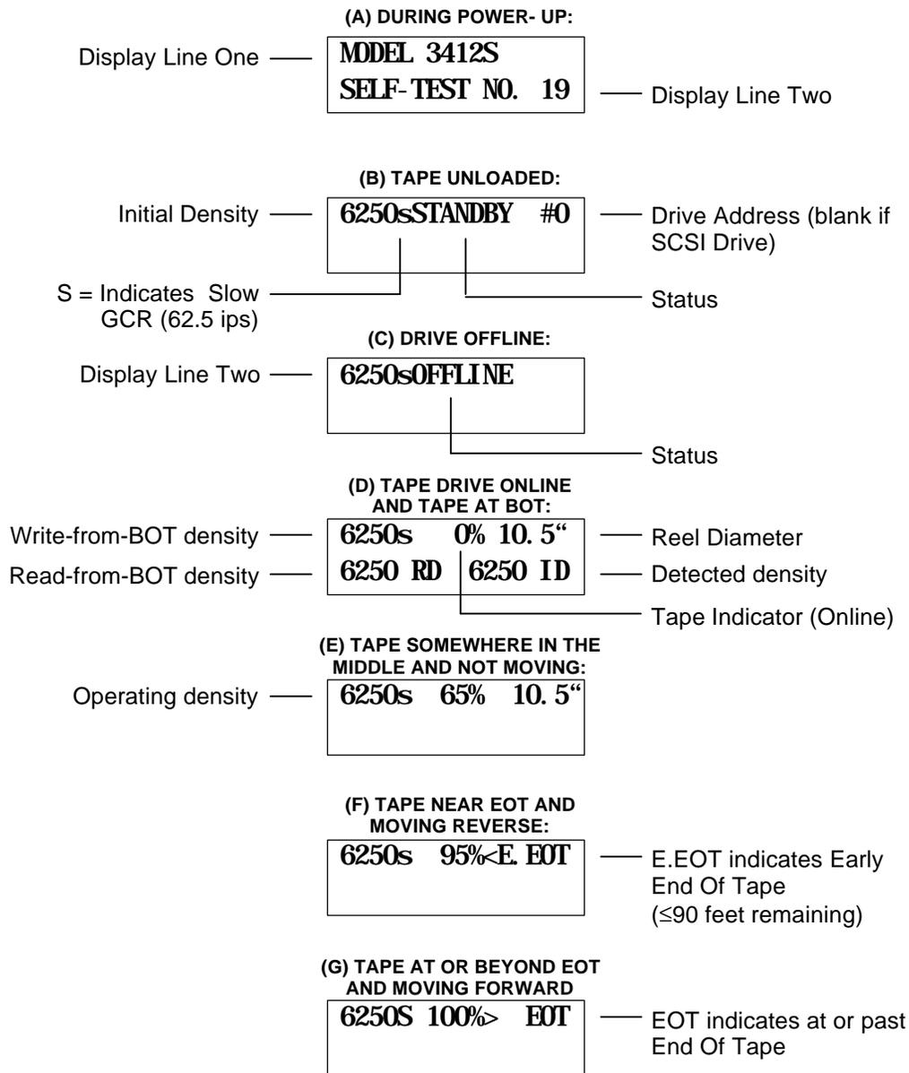
Figure 2-2 LCD during Various Phases of Operation
