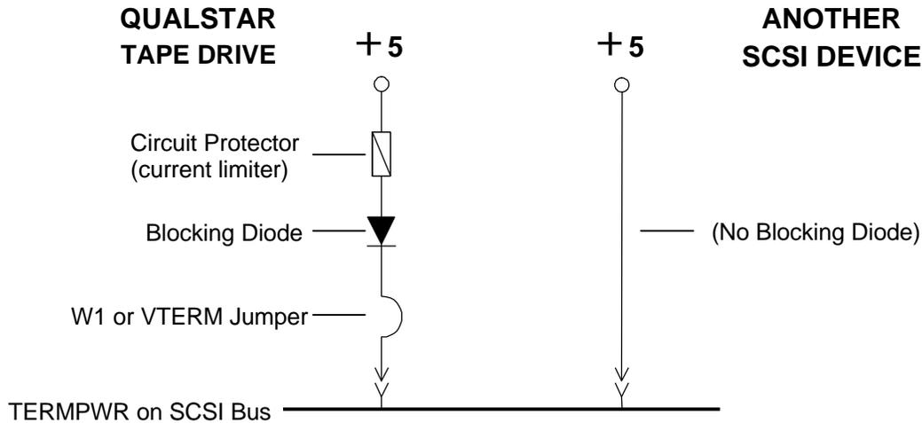
Figure 1-9 Diagram of SCSI Termination Power
