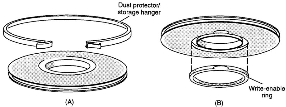
**Figure 3-3 Dust Protector and Write-enable Ring**
