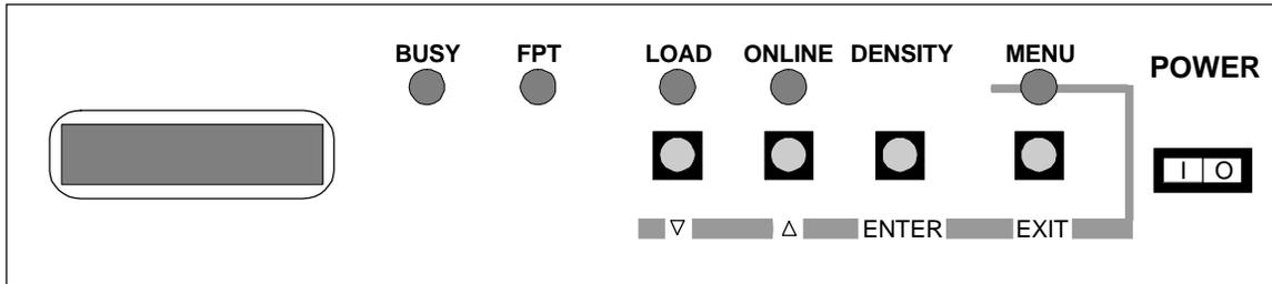
Figure 2-1 Front Control Panels
