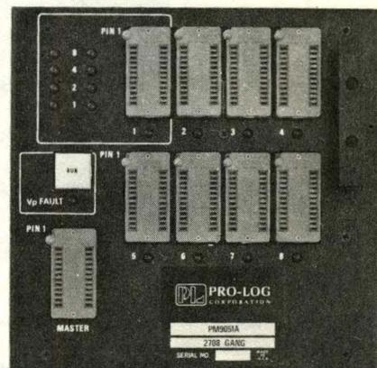
\*Due to the increased current drain of multiple device programming, M900 and M920 Control Units manufactured prior to October 1, 1977 should be returned to PRO-LOG for updating to Gang Module compatibility. Contact Customer Service for return authorization. Cost of retrofit: \$50 FOB Monterey.
