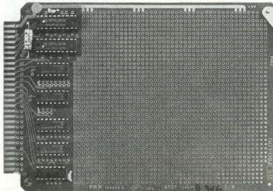
7904 Decoded Input/Output Utility Card
