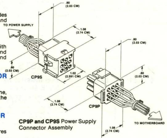
**CP9P and CP9S Power Supply Connector Assembly**
