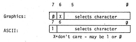
Ø is "on" or "bright," l "off" or "dark." Thus, storing ØllØlØlØB (6AH) at a screen location produced this graphic at that location:
