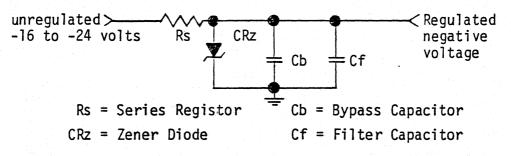
The bypass capacitor (Cb) should be a  $0.1_{\rm U}$  F or  $0.01_{\rm U}$  F ceramic disc; the value is not critical. The filter capacitor (Cf) should be a  $10_{\rm U}$  F 25-35 volt tantalum with the positive lead to ground (ground is positive with respect to the negative regulated voltage).
