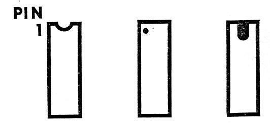
To install a DIP into the socket, insert the pins on one side a very slight distance into the socket. Apply a slight sideways pressure on the pins of this side. Now, reverse the procedure. Bend the pins only until both sides begin to enter the socket holes.
