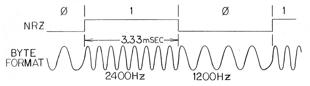
FIG1a. NRZ and Byte format per bit.
