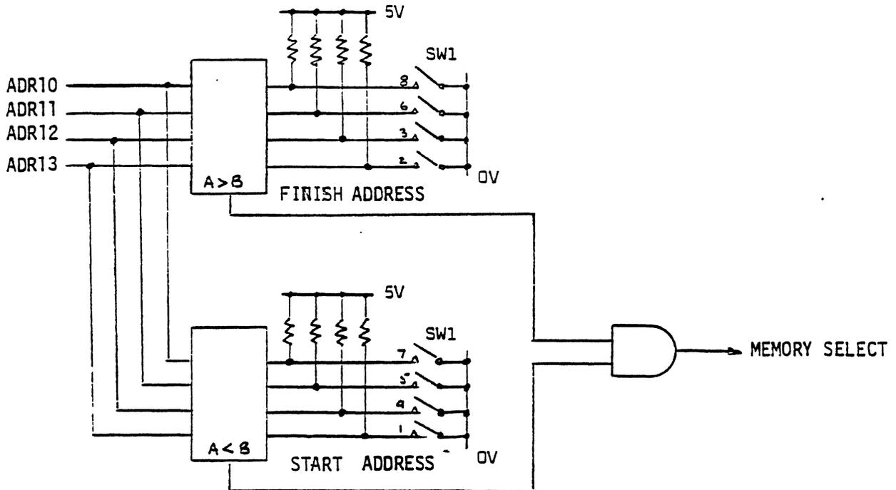
The finish address is determined by switch positions 2, 3, 6 and 8.
