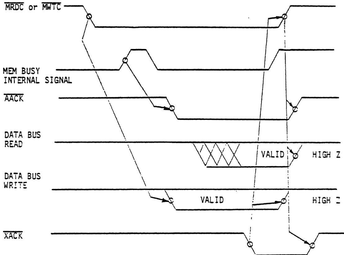
AACK and XACK delayed if MRDC or MWTC while Refresh Cycle is in progress.
