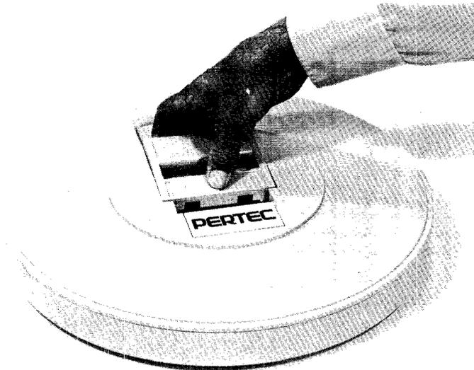
Figure 3-5. Cartridge Loading, Top Load Models (Release/Lock Down)
