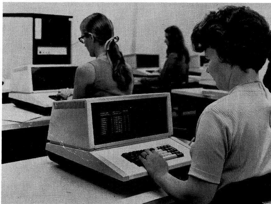
*The 1900 CADE System supports up to 32 of the CRT keystations shown here. The display is arranged in 12 lines of 40 characters each, and the keyboard is available in standard keypunch, keypunch/adding machine, or typewriter arrangements. The control processor cabinet is shown in the left background.*
