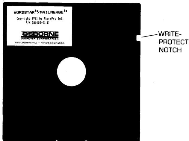
When the write-protect notch is covered, information can still be read from your protected diskette, but data cannot be written onto the diskette. Valuable programs and data should be protected in this manner to prevent accidental overwrites or erasures.
