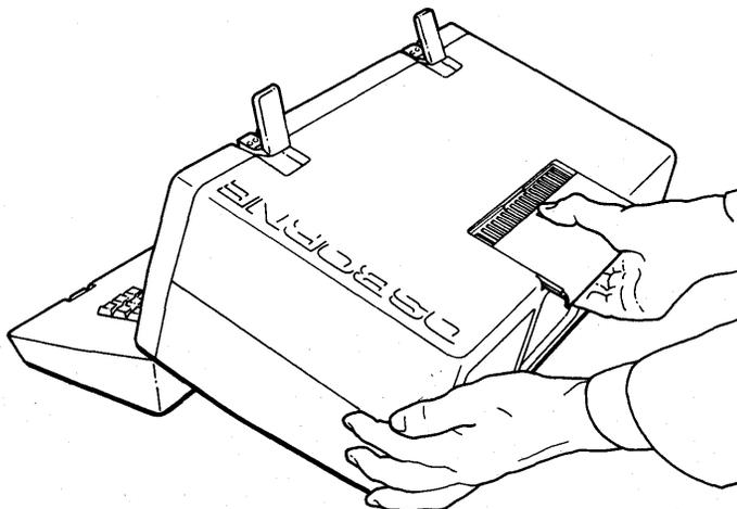
The power cord, power switch, fuse card, and circuit breaker fuse are all located in the covered power well, next to the handle. The hatch covering the power well opens very easily, just pull the tab and lift upward.
