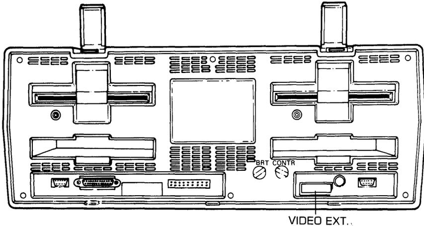
The plug that comes with your Osborne 1 selects the 5-inch built-in monitor as the display location. If you like, a special adaptor may be purchased which allows an external monitor to be connected through this slot.
