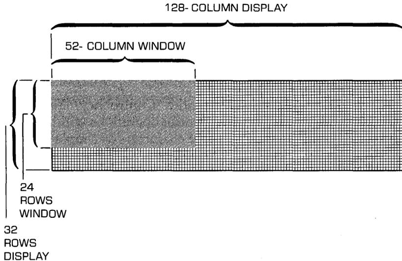
The monitor built into the Osborne 1 has a 5-inch diagonal screen. Optional external monitors are larger, usually 12 inches diagonally. Since an optional monitor displays the same number of characters, the characters will appear bigger.
