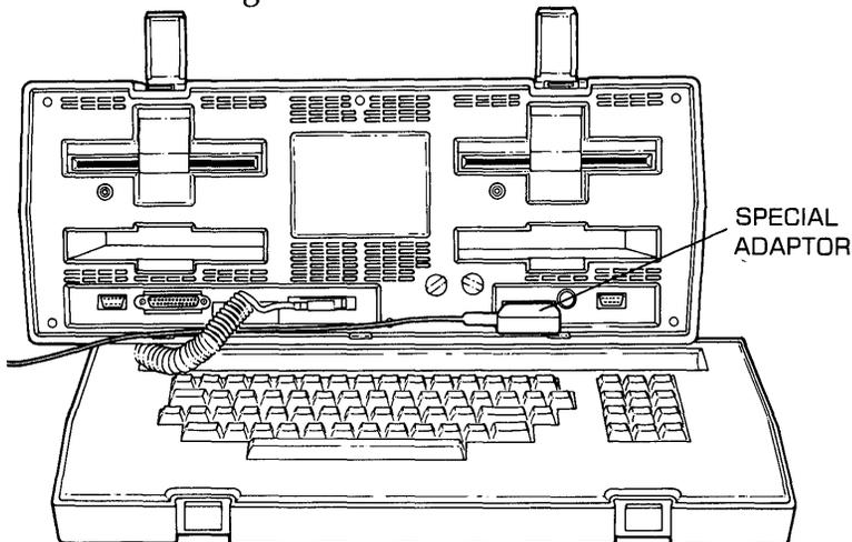
Sometimes rough shipping of the computer may result in the brightness and contrast controls being slightly out of adjustment. If you're still not getting a display, try "twiddling" with the knobs labeled **BRT** (for brightness) and **CONTR** (for contrast). These controls work very much like those on your television set. The proper method for setting the brightness and contrast levels is as follows:
