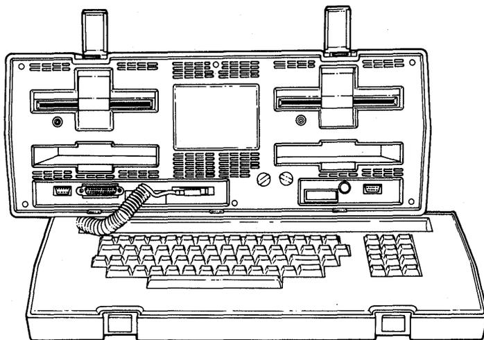
There is a vent on the Osborne 1 used to dissipate heat when the computer is in use. The vent, located on the top side (when the computer is set up for use), should always be uncovered. To open the vent, press the finger-sized, corrugated depression and slide the cover in the direction of the handle.
