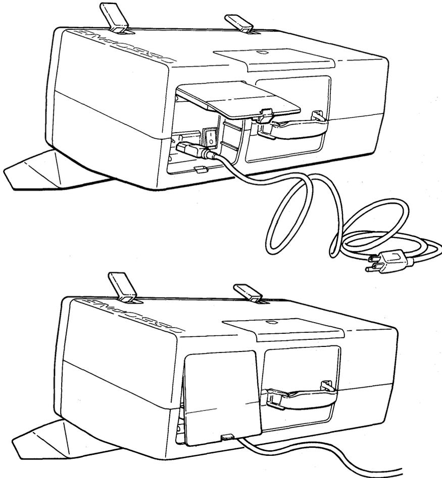
When you power up the computer, some information should appear on the screen (referred to as the "monitor"). We will discuss the information displayed on the monitor in chapter 2. If after a few moments nothing appears, check the small opening below the monitor and slightly to the right, labeled **EXT VIDEO**. A rectangular-shaped plug should securely fit this slot. If this plug is loose or disconnected, **TURN OFF THE POWER TO THE COMPUTER** and then reconnect it.
