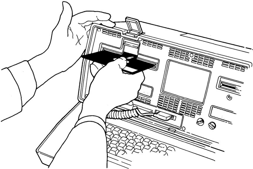
When the diskette is securely in the drive, close the door. This door must be closed for the disk drive to work properly. To remove the diskette, flip the door open and gently pull the diskette out. When inserting or removing the diskette, do not bend it.
