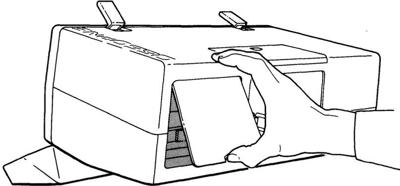
Notice that the fuse and fuse card are accessible by sliding the clear plastic fuse cover over the three-pronged plug. A one-amp fuse protects the internal components from damage caused by power overloads. To replace the fuse, slide the fuse cover away from the fuse, then pull upward on the "fuse pull" tab.
