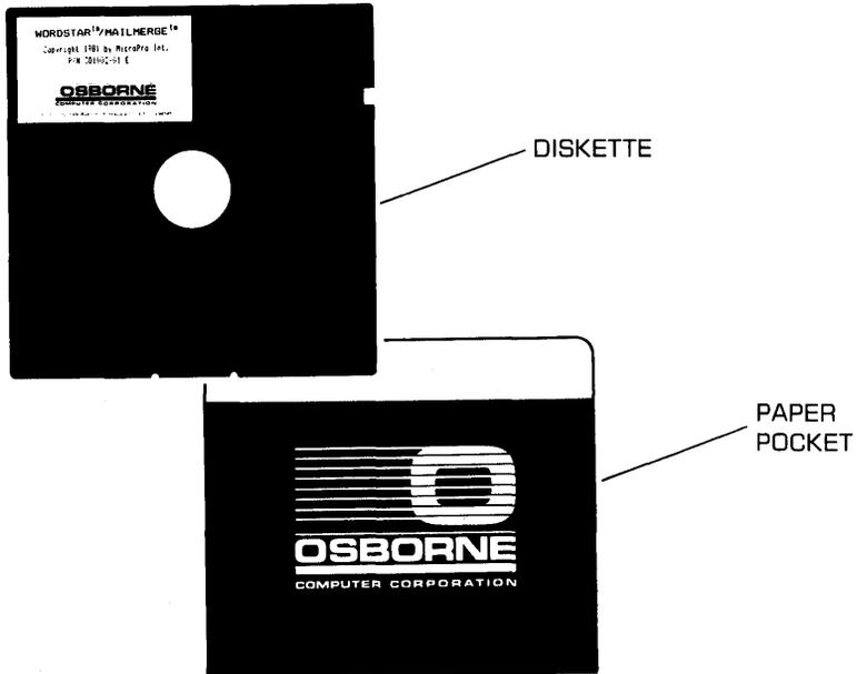
To use a diskette you must remove it from the paper pocket. Do not try to remove the plastic disk from the cardboard envelope, or you will destroy the diskette.
