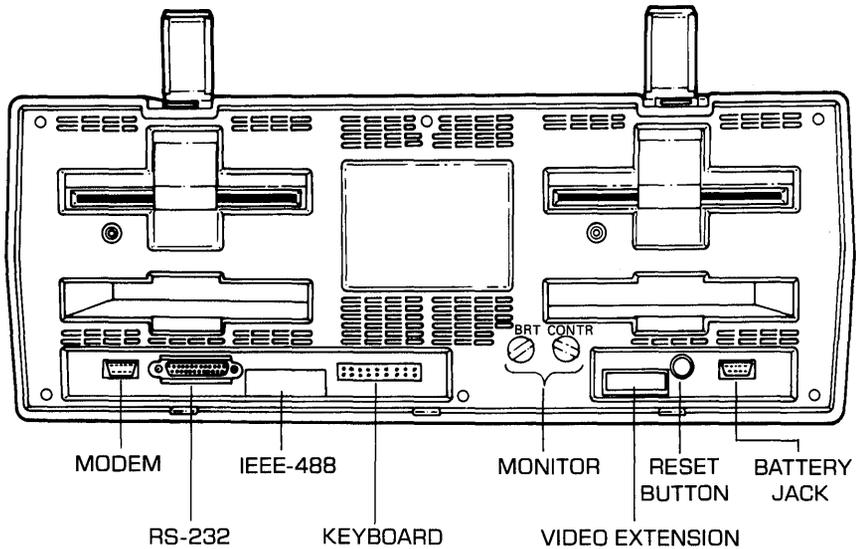
Immediately to the right of the modem connector is one labeled **SERIAL RS232**. RS-232 refers to a computer-industry standardized method of connecting devices to a computer. Your Osborne 1 is compatible with many other devices through this port. Most printers use the RS-232 method of “communicating” with the computer, for instance.
