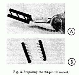
position. Solder all 24 pins with the thin solder.
