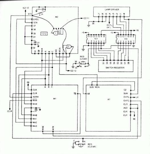
Fig. 88-1. Serial BCD Adder.
