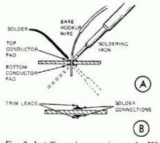
Fig. 2. Installing a jumper wire on the M3 circuit board. (A) soldering the jumper, and (B) the completed connection.
