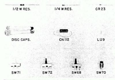
Fig. 1. Some of the experimental parts for this training kit are shown above.
