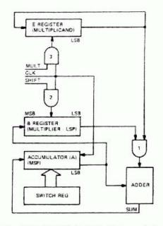
Fig. 86-4. Simplified block diagram of the Serial Multiplier.
