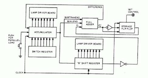
Fig. 85-6. Block diagram of circuit used in Step 2.
