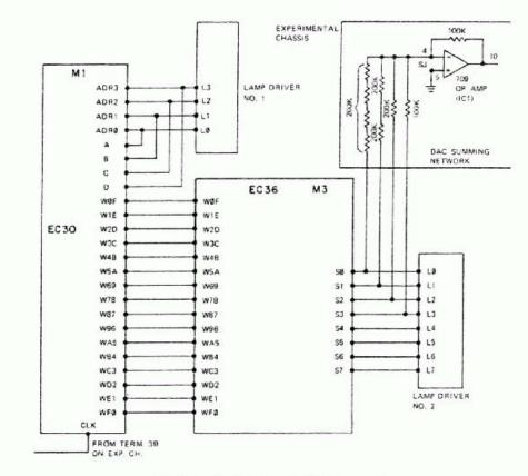
Fig. 82-1. Circuit for Step 1, Experiment 82.
