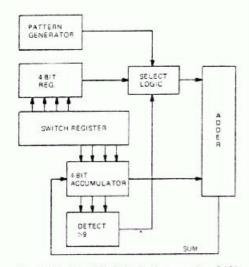
Fig. 88-2. Simplified block diagram of an 8421 BCD Serial Adder.
