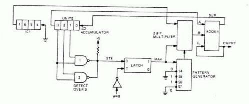
Fig. 88-3. Select Logic Operation.
