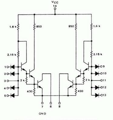
Fig. 81-2. Circuit of 15844 (or 944) IC used in the memory.
