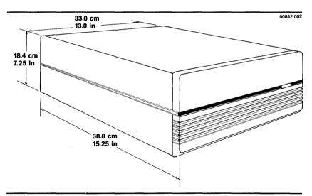
■ Figure 1-2. Dimensions of the  $\mu$ Analyst 2000 Mainframe.
