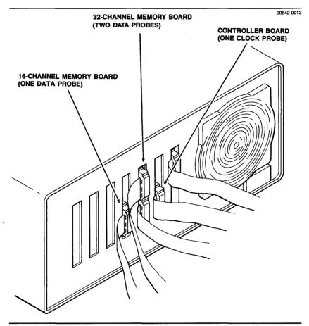
Figure 2-12. Connecting the probes to the boards.
