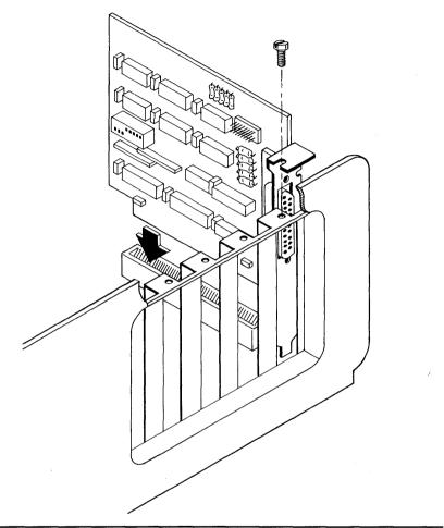
■ Figure 2-7. Installing the PC interface board.
