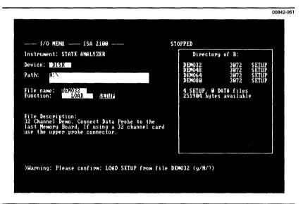
Figure 7-7. Loading the demo file.
