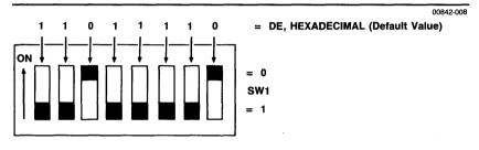
■ Figure 2-6. Address switches on the PC interface board. These switches are factory-set to the address range DE000—DEFFF, hexadecimal. The polarity of the switches is inverted so that ON=0 and OFF=1.
