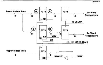
Figure 7-17. Input circuitry of the memory board.
