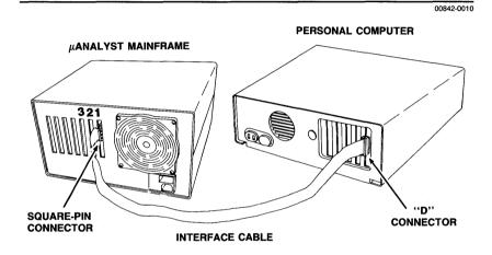
■ Figure 2-8. Connecting the interface cable.
