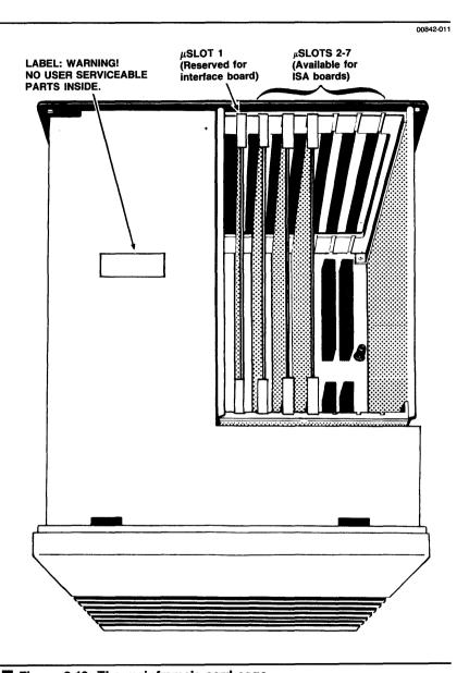
Figure 2-10. The mainframe's card cage.
