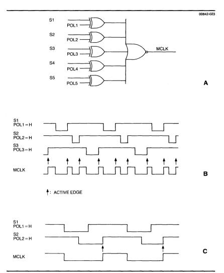
■ Figure 4-4. Using the five sample clocks to form the master clock.
