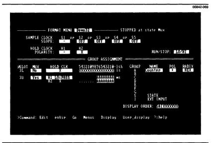
Figure 7-15. Setting up to detect a hold clock.
