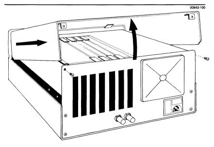
■ Figure 2-9. Removing the mainframe's cover.
