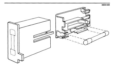
Figure 2-4. Detaching the fuse-holder circuit board.
