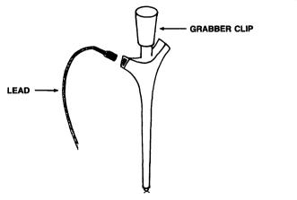
Figure 2-14. Installing a grabber clip.
