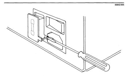
Figure 2-3. Removing the fuse holder.
