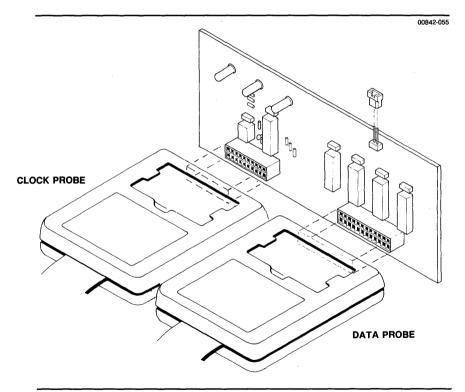
Figure 7-1. Installing the demo circuit board.
