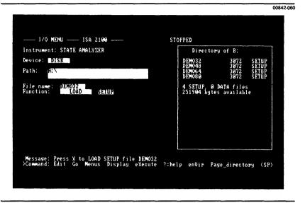
Figure 7-6. Setting up the I/O Menu to load the demo file.
