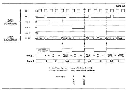
■ Figure 4-7. Using sample and hold clocks with a multiplexed microprocessor.
