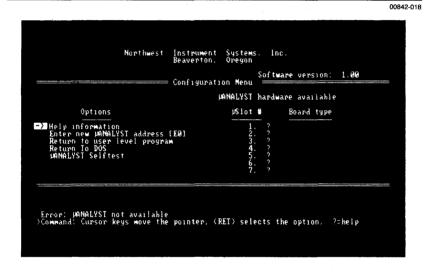
Figure 3-3. Start-up error condition.
