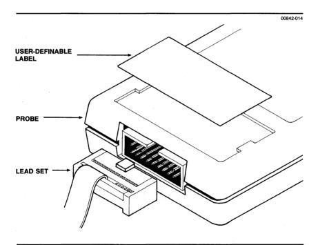
■ Figure 2-13. Installing a lead set on a probe.
