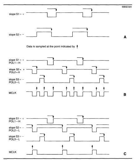
■ Figure 4-5. The effects of sample clock polarity.
