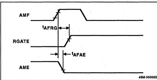
**Figure 14. One-Bit Transfer Timing (to Drive)**
