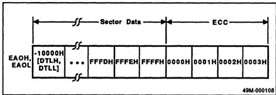
**Figure 25. Detect Error Command; Error Pattern (EPT)**
