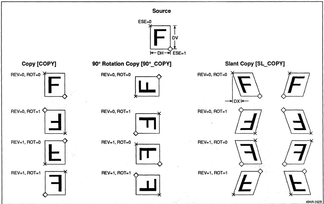
Figure 27. Copy Commands; Enlarge/Shrink, Rotate
