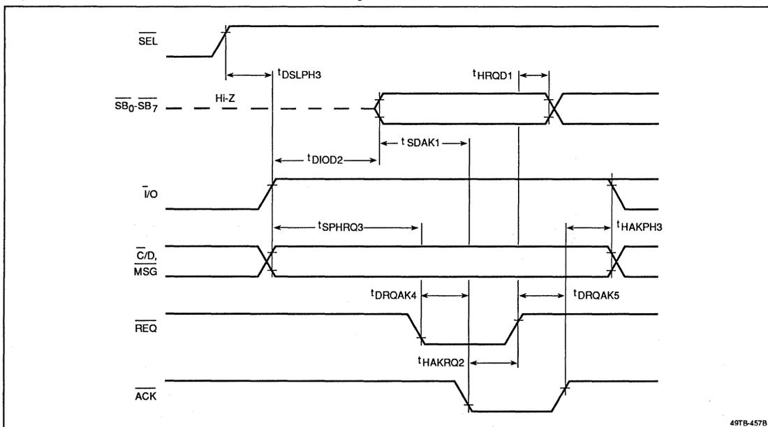
**Figure 15. SCSI Bus; Reception as Target in Async Mode**
