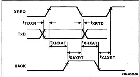
**Figure 15. One-Bit Transfer Timing (from Drive)**
