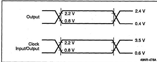
**Figure 3. Reset Waveform**
