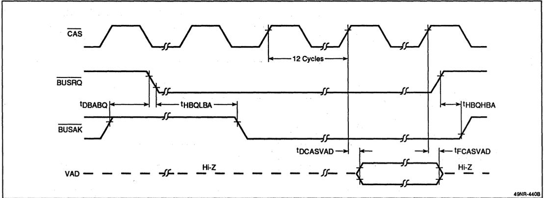
Figure 11. Data Transfer Cycle
