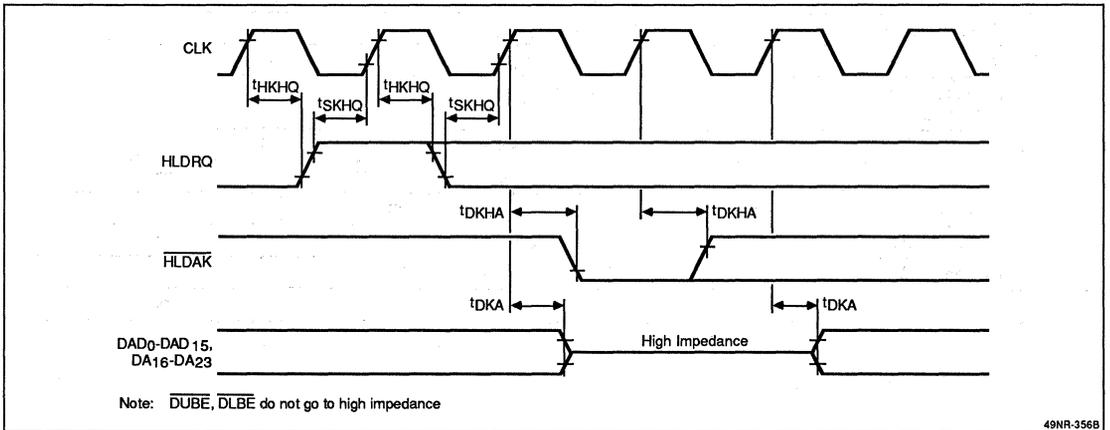
Figure 5. DMA Read Cycle
