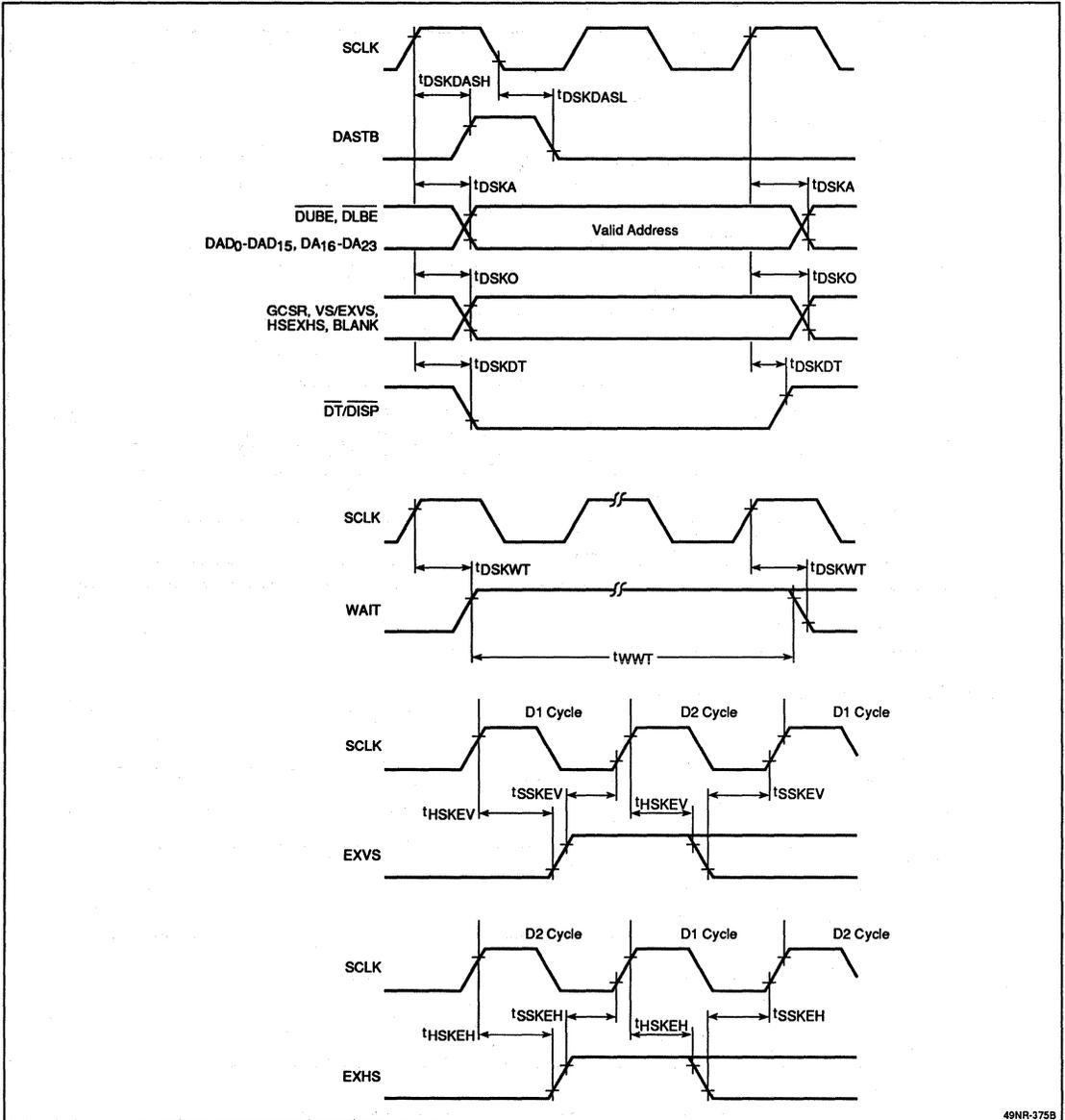
**Figure 12. Display Refresh Cycle (DT Mode)**
