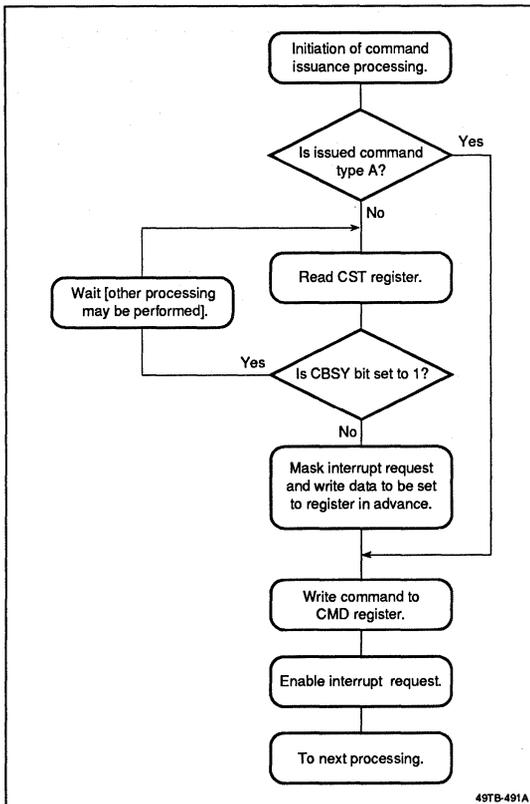
**Figure 45. Interrupt Processing Flow**
