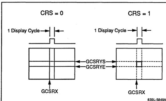
Figure 23. Horizontal and Vertical Timing Parameters
