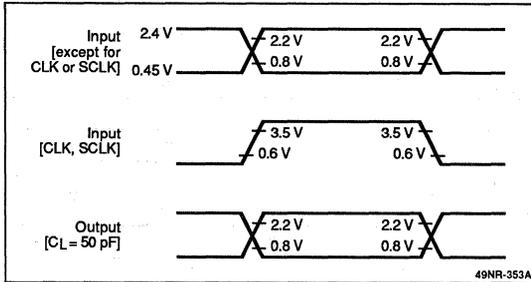
**Figure 3. Reset and Interrupt Waveforms**
