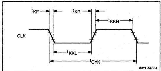
Figure 3. DMA Transfer Timing on Image Bus
