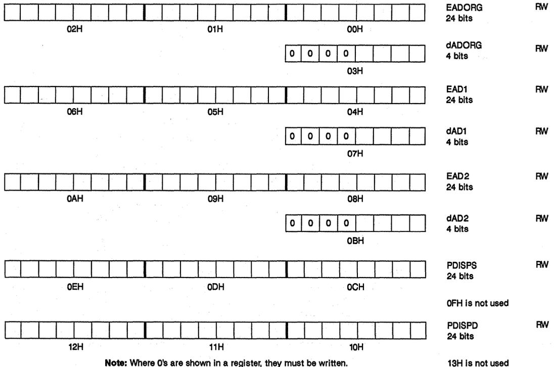
**Figure 14. Register Configurations (cont)**
