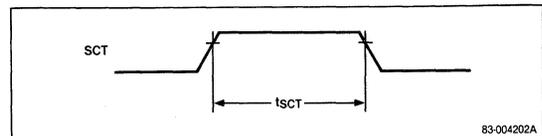
**Timing Waveforms — ST506-Type Interface**
