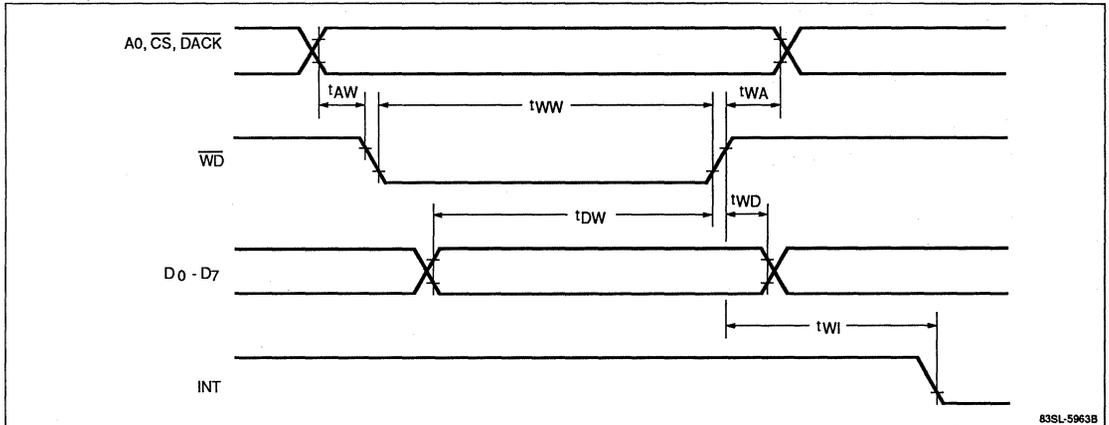
Figure 4. DMA Operation
