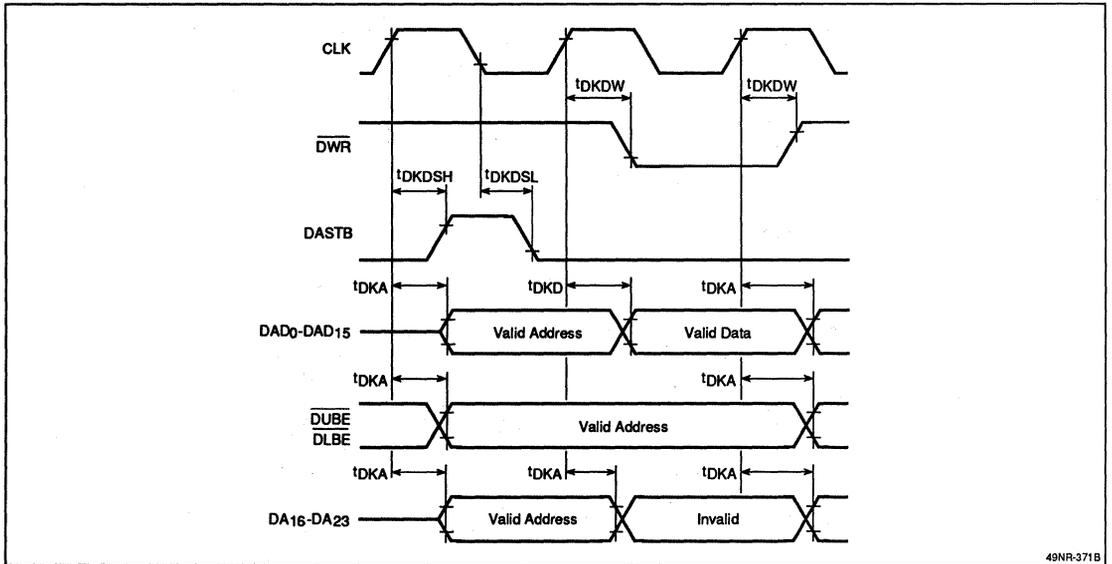
Figure 9. System Bus Read Cycle
