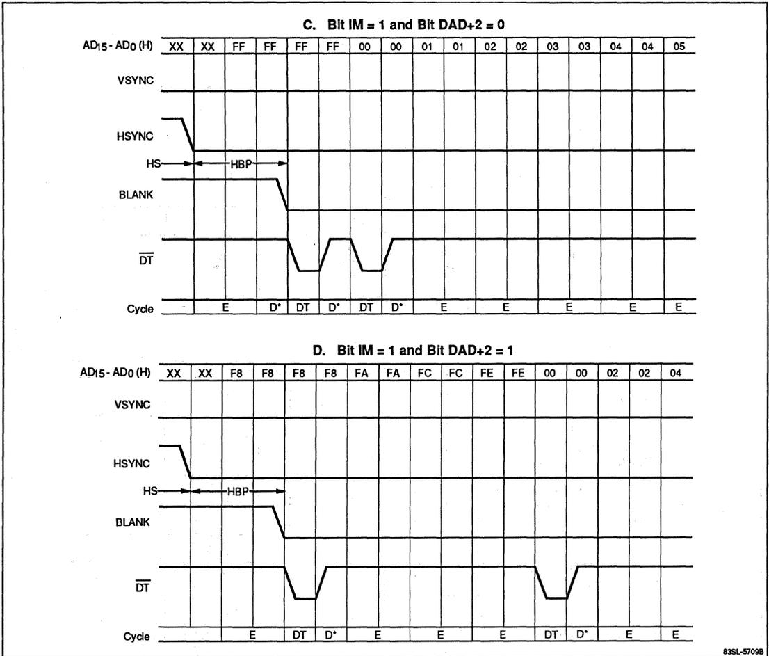
Figure 5.  $\overline{DT}$  Signal Output, Mode 1 and Mode 2
