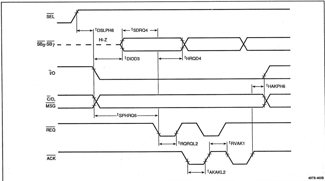
**Figure 18. SCSI Bus; Transfer as Initiator in Sync Mode**
