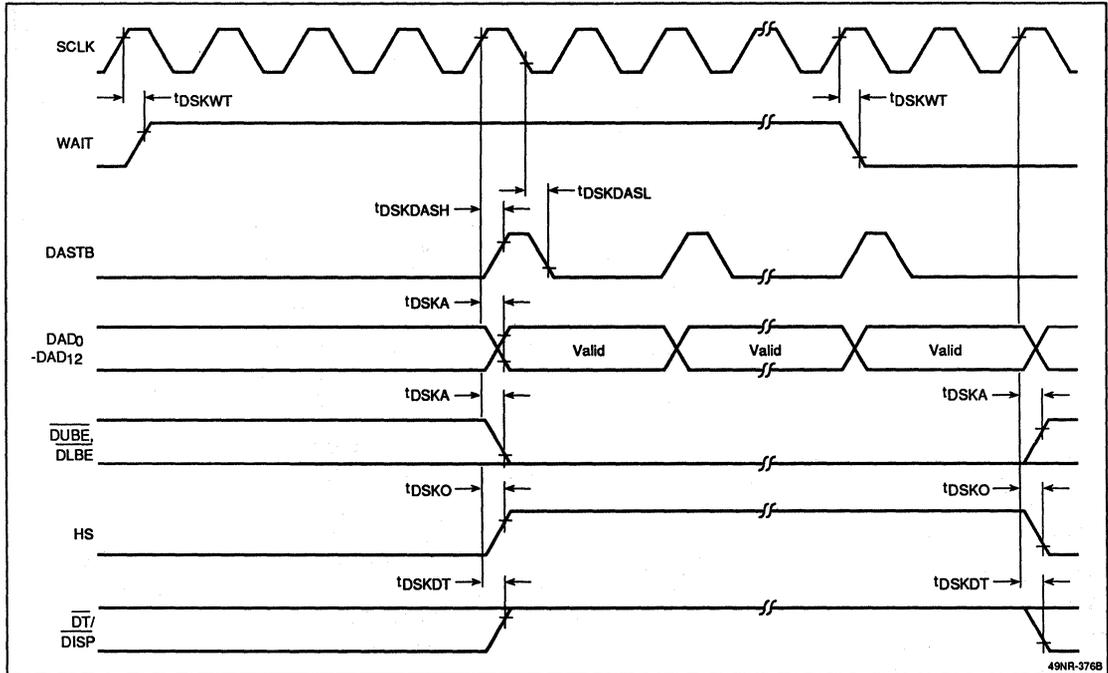
**Figure 13. Display Refresh Cycle (CS Mode)**
