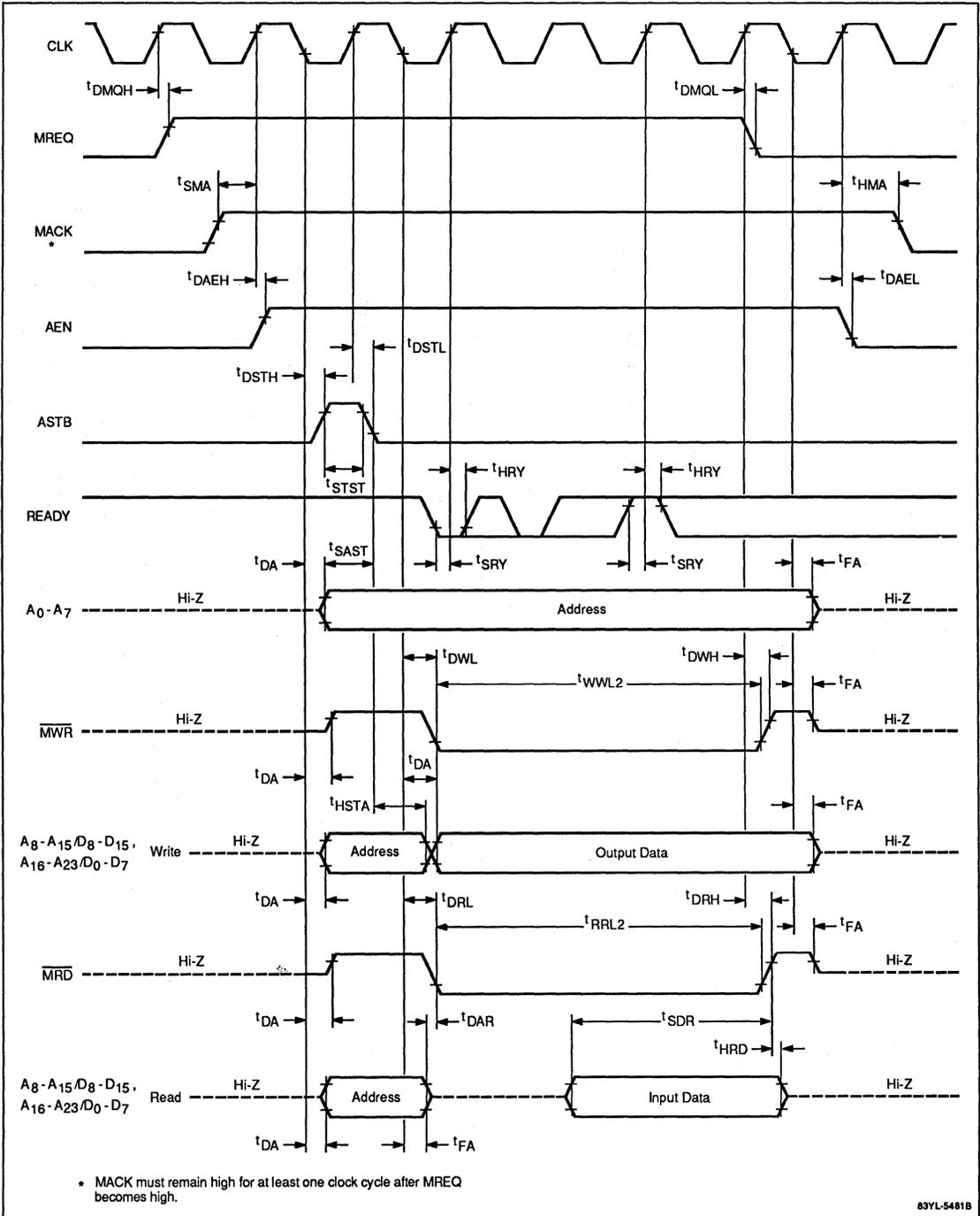
**Figure 4. Timing for Read from  $\mu$ PD72185 on Host Bus**
