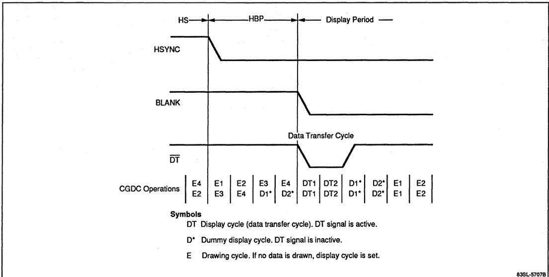
Figure 4.  $\overline{DT}$  Signal Output, Mode 0 (Sheet 1 of 2)
