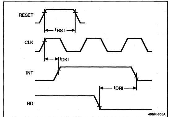
**Figure 2. Clock Waveforms**
