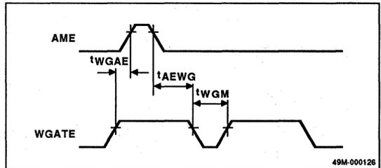
**Figure 17. Communications Timing**
