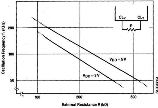
**Supply Voltage vs Oscillation Frequency**
