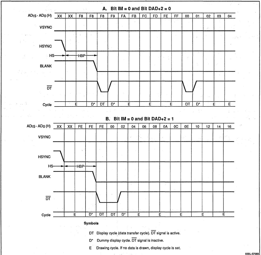
Figure 4.  $\overline{DT}$  Signal Output, Mode 0 (Sheet 2 of 2)
