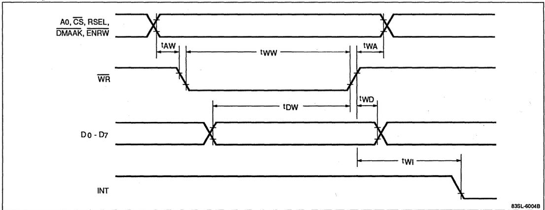
Figure 4. DMA Operation
