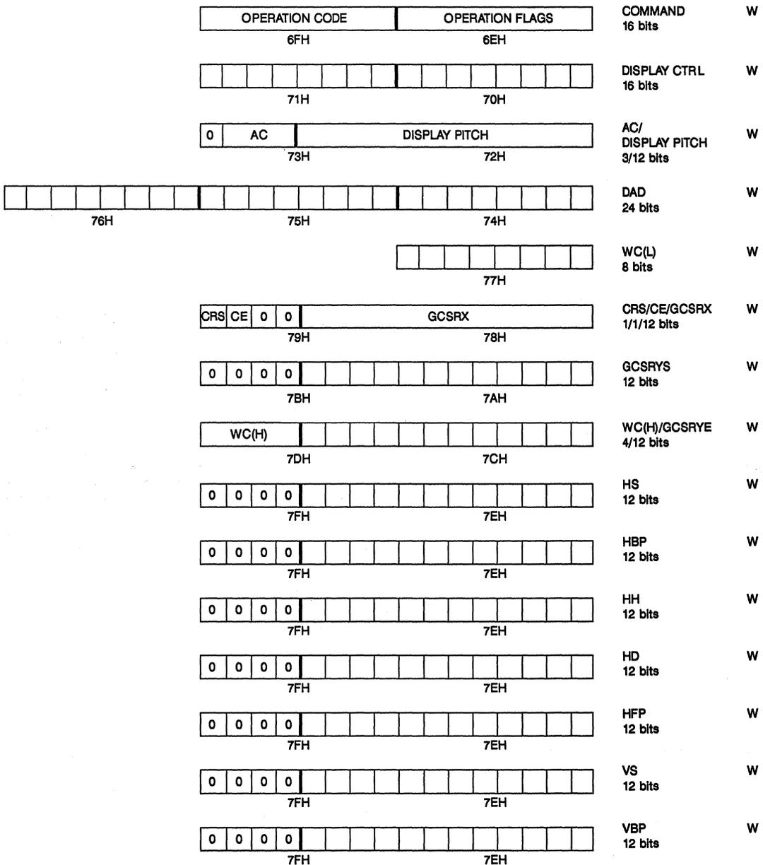
**Figure 14. Register Configurations (cont)**
