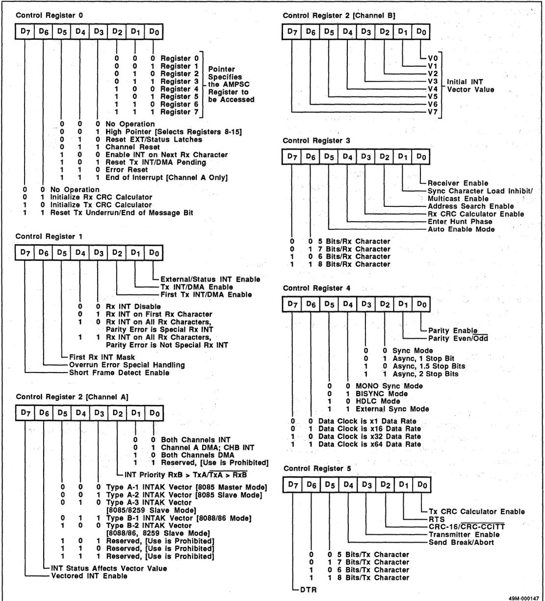
Figure 4. Control Register Bit Functions (cont)
