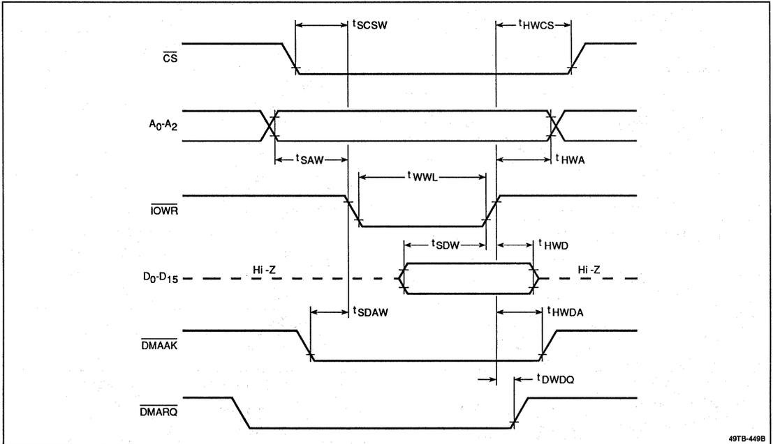
**Figure 6. Other CPU Bus Timing**
