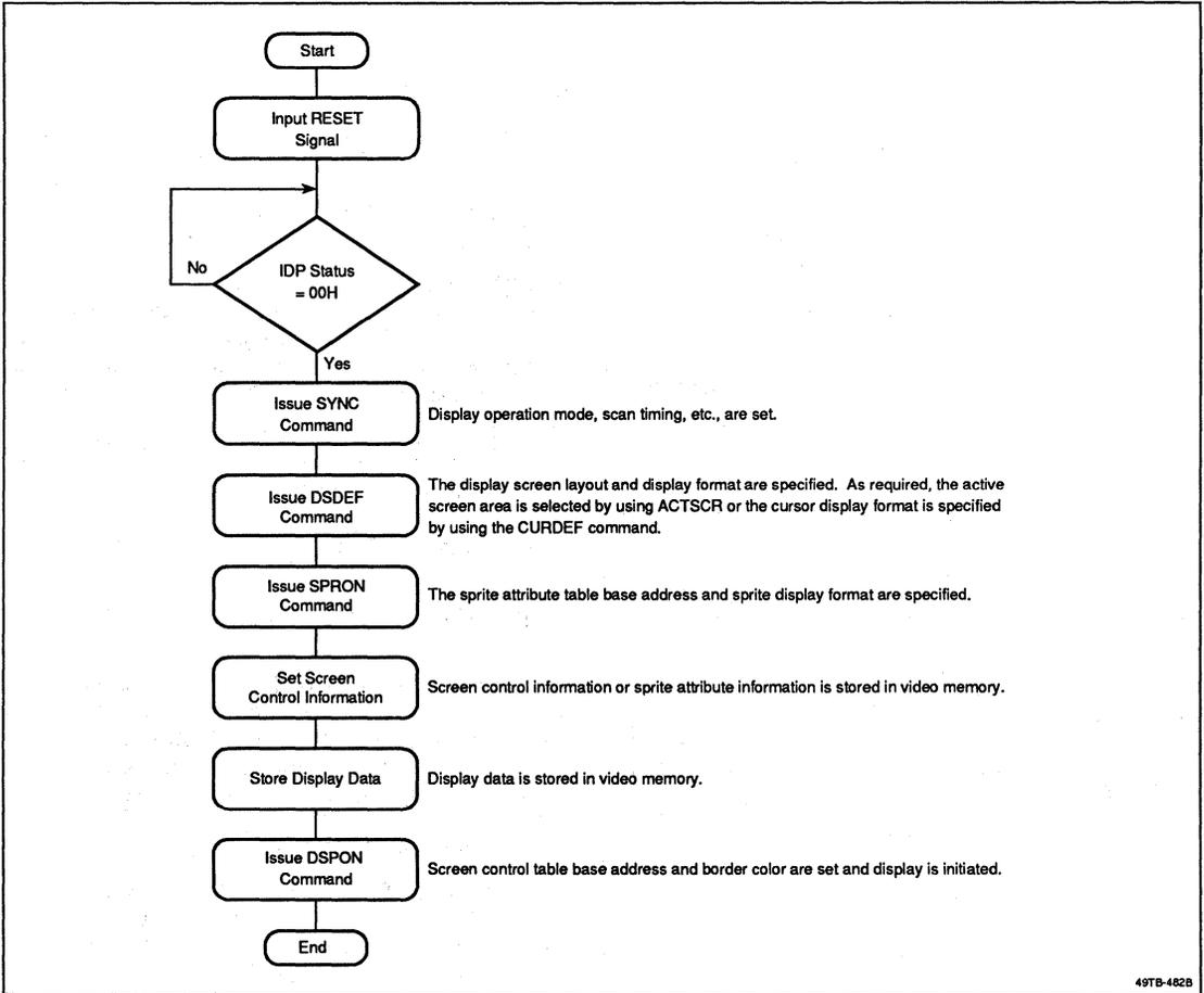
Figure 20 μPD72022 Basic Control Flow
