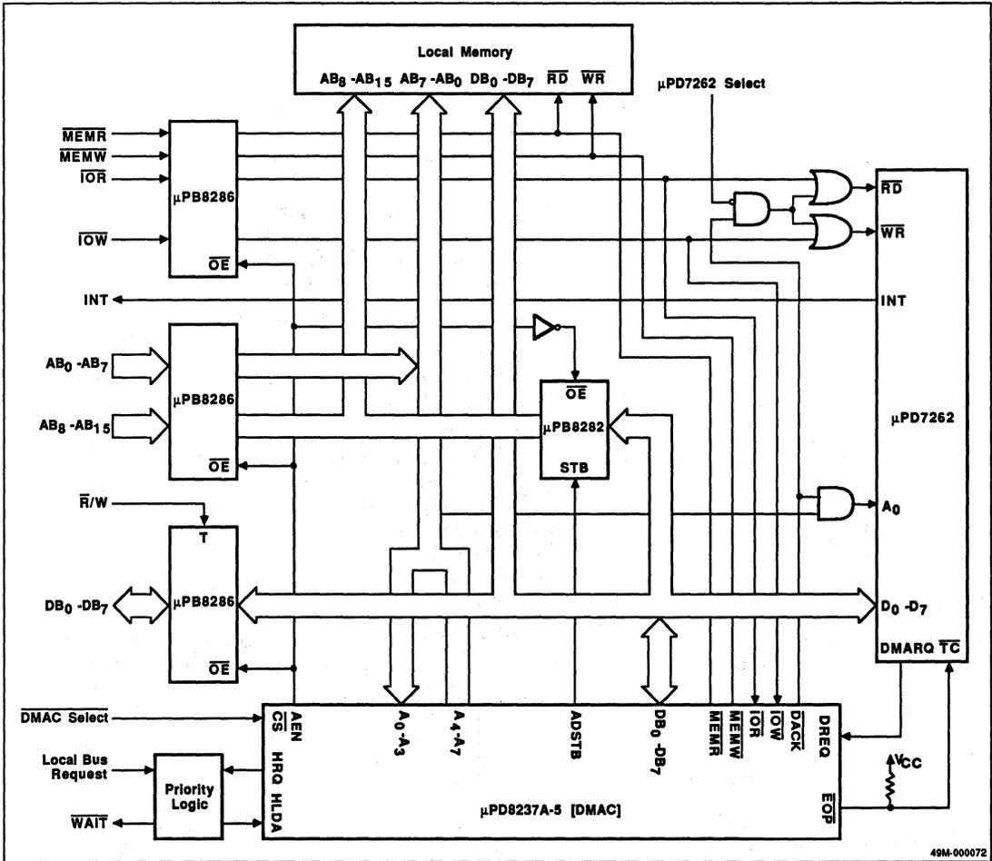
Figure 27. Example of the Interface Between the μPD7262 and a Hard-Disk Drive
