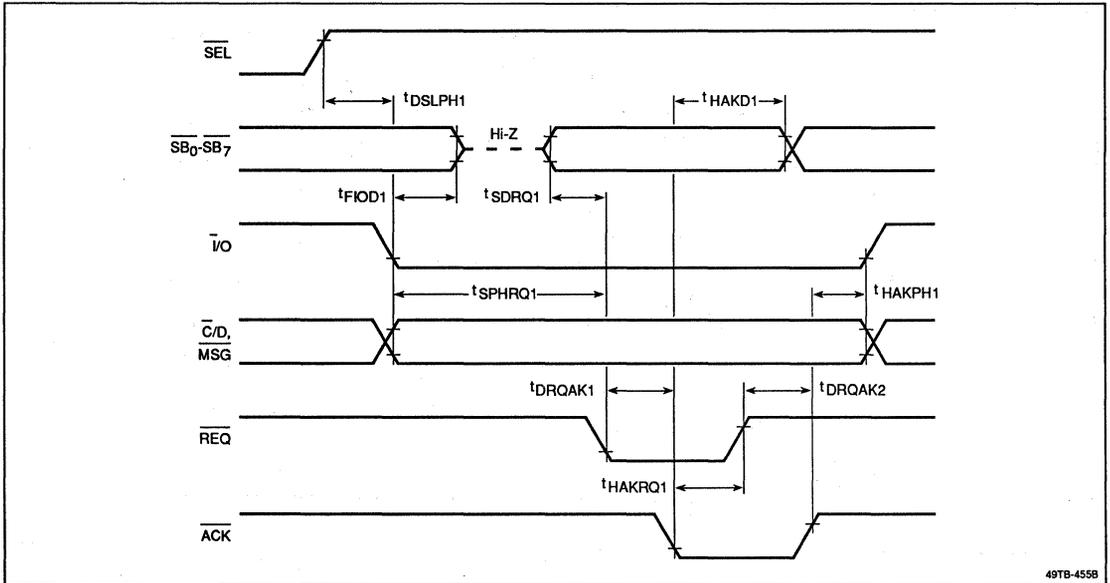
Figure 13. SCSI Bus; Transfer as Target
