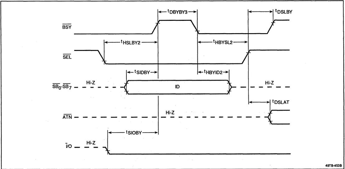
**Figure 11. SCSI Bus; Reselection as Target**
