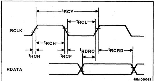
**Figure 10. Data Write Timing**
