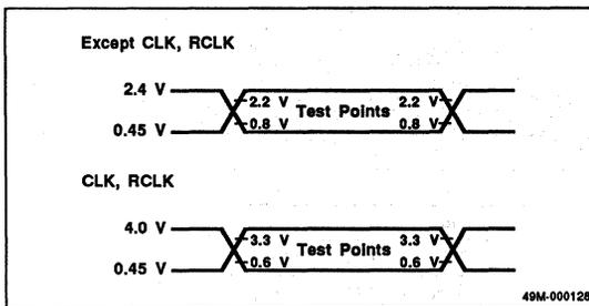
Figure 2. CLK Pulse Timing
