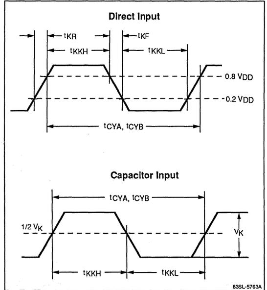
**Figure 3. Voltage Thresholds for Timing Measurements**
