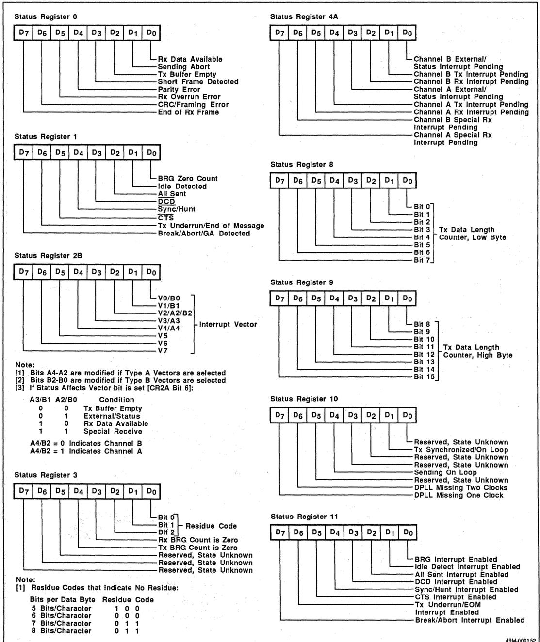
**Figure 5. Status Register Bit Functions (cont)**
