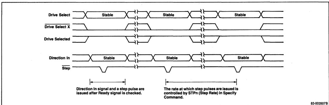
Figure 20. "Buffered Seek" Timing (Soft Sector)
