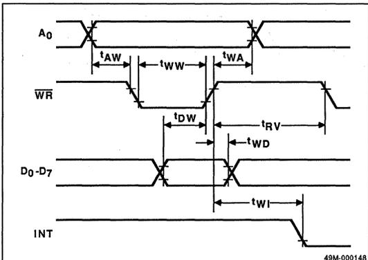
**Figure 7. DMA Read Timing**
