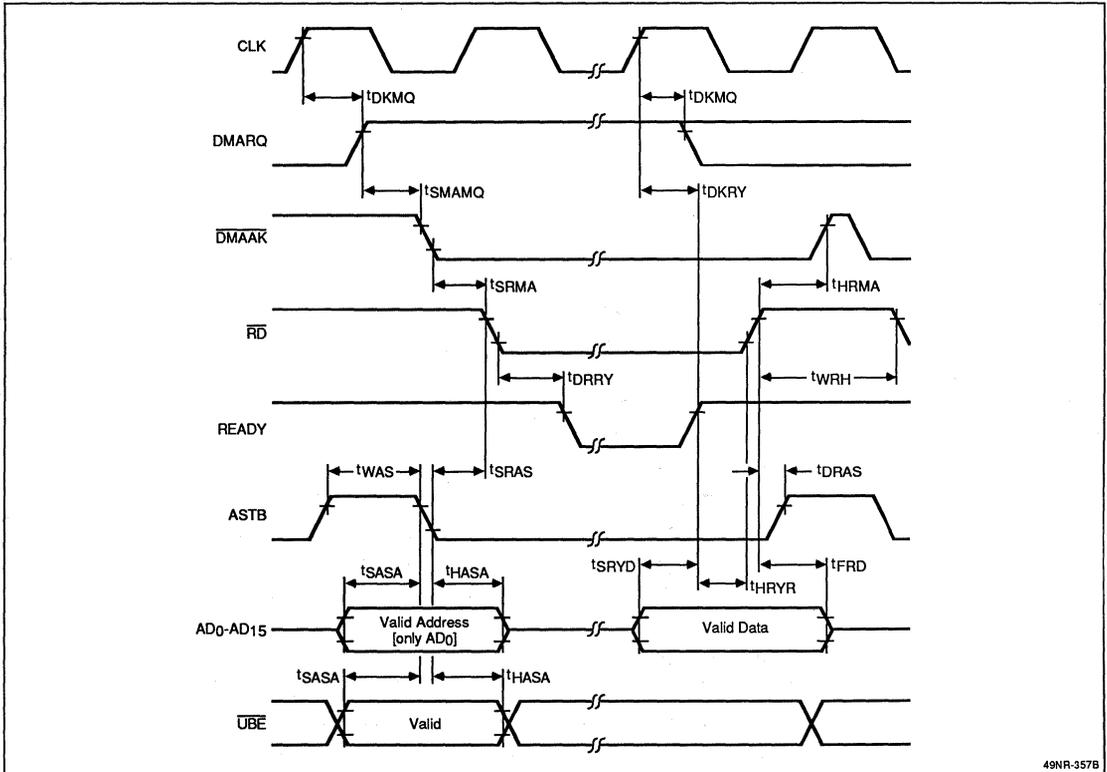
**Figure 6. DMA Write Cycle**
