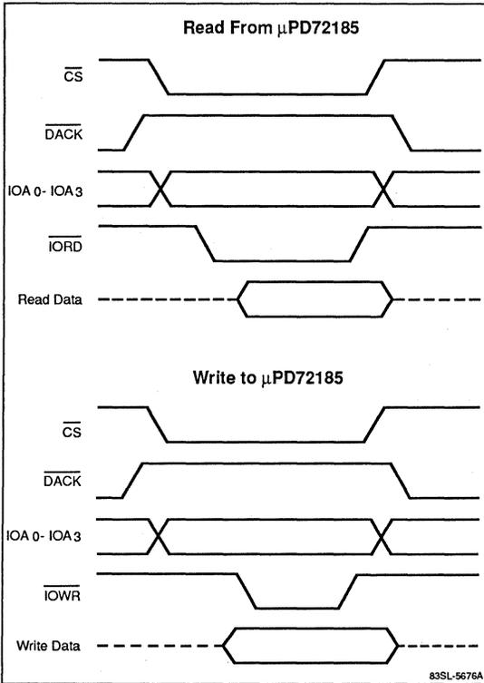
**Figure 14. Read/Write Timing With External DMA Controller**
