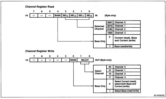
Figure 40. DMA Device Control Register
