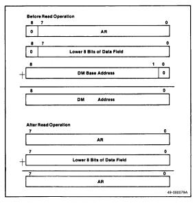
the lower eight bits of the data field of the token, and the DM Base address. After the read operation, the lower eight bits of the token's data field is added to the value of AR. Additionally, the data field of the token is replaced by the contents read from the Data Memory location.
