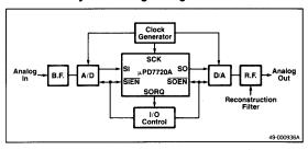
Figure 25. A Signal Processing System Using Cascaded SPIs & Serial Communication
