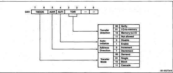
Figure 43. DMA Mask Register
