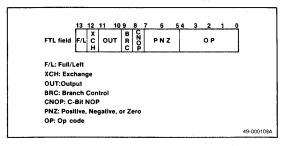
PU instructions (see table 20) are stored in the Function Table Left field of the Function Table memory. The bits 0 through 11 are used as control information for the Processing Unit. The bits 12 and 13 are deleted before the token arrives at the Processing Unit. Two operands from the A and B sides are operated on by the Processing Unit and the result is output to the X and Y sides (see figure 19).
