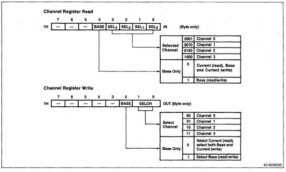
Figure 40. DMA Device Control Register
