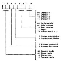
Request Register. This register allows the  $\mu$ PD8237A to respond to DMA requests from software as well as hardware. There is a bit pattern for each channel in the request register. These bits can be prioritized by the priority resolving circuitry and are not maskable. Each bit is set or reset under software control or cleared when TC or an external  $\overline{\text{EOP}}$  is generated. A reset clears the entire register. The correct data word is loaded by software to set or reset a bit.
