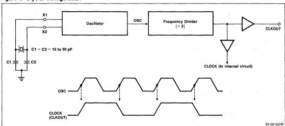
Figure 9. External Oscillator Configuration
