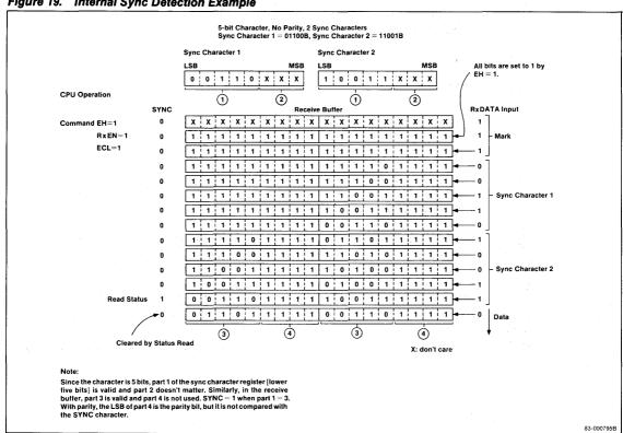
Figure 19. Internal Sync Detection Example
