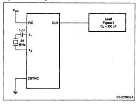
Figure 2. Clock High and Low Time
