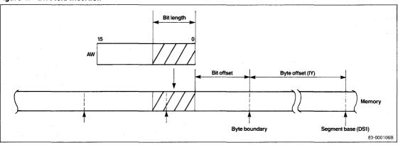
Figure 5. Bit Field Extraction
