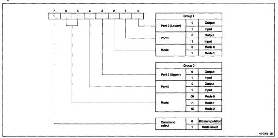
Figure 2. Bit Manipulation Command Word
