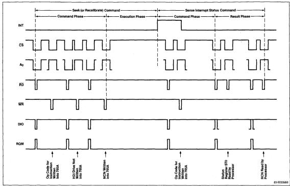
Figure 4. Seek, Recalibrate, and Sense Interrupt Status
