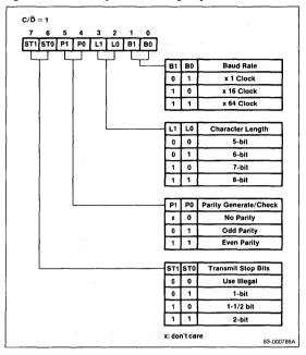
Figure 5. Mode byte for Setting Synchronous Mode
