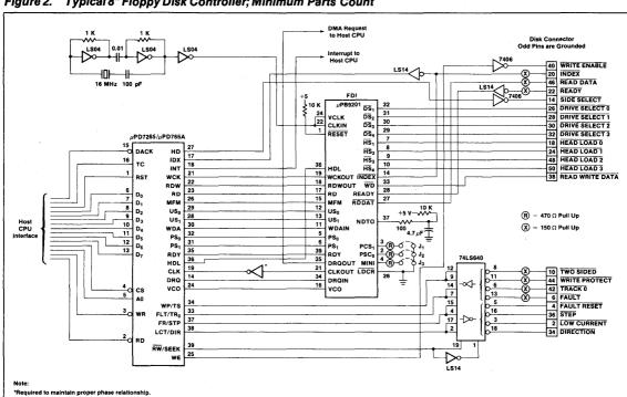
Figure 2. Typical 8" Floppy Disk Controller; Minimum Parts Count
