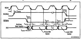
Figure 9. Serial Output Case #3: SOEN Active before SORQ is High
