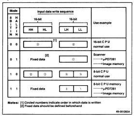
Figure 5. Setting Read Method for Output Data
