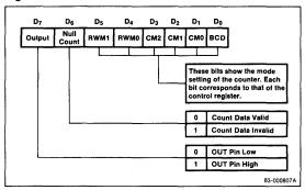
Initial OUT refers to the state of the OUT pin immediately after the mode is set.
