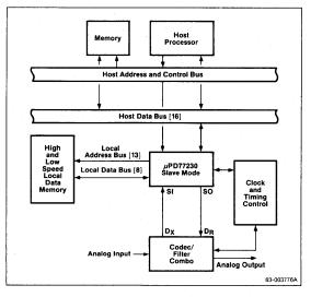
Figure 9. µPD77230s Cascaded Through Serial I/O Ports
