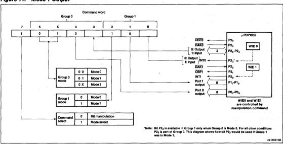
Figure 12. Mode 1 Output Timina
