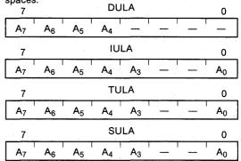
Figure 13. μPD70216 Peripheral Relocation
