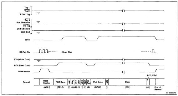
Figure 17. "Data Write" Timing (Hard Sector)
