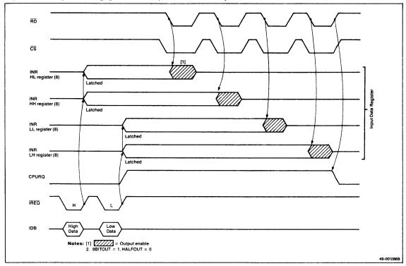
Figure 11. Output to  $\mu$ PD7281, Control Data Paths
