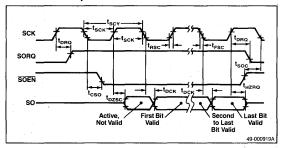
Figure 8. Serial Output Case #2: SOEN Asserted in Response to SORQ when SCK is High
