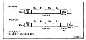
Figure 11. Asynchronous Transmitter Example
