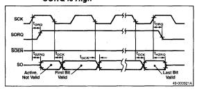
Figure 10. Serial Output Case #4A: If SOEN is Released in the Middle of a Transfer During SCK High
