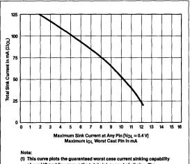
(f) This curve plots the guaranteed worst case current sinking capability of any I/O port line versus the total sink current of all pins. The  $\mu PD82C43$  is capable of sinking 5 mA (for  $V_{OL}=0.4$  V) through each of the 16 I/O lines simultaneously. The current sinking curve shows how the individual I/O line drive increases if all the I/O lines are not fully loaded.
