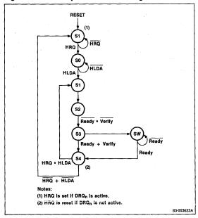
The DMA cycle consists of four internal states; S1, S2, S3, and S4. If the access time of the memory or I/O device is not fast enough to return a ready command to the  $\mu$ PD8257 after it reaches state S3, then a wait state is initiated (SW). One or more than one wait state occurs until a ready signal is received, and the  $\mu$ PD8257 is allowed to go into state S4. Either the extended write option or the DMA verify mode may eliminate any wait state.
