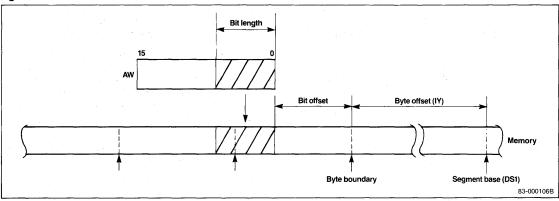
Figure 5. Bit Field Extraction.
