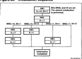
slave  $\mu$ PD71059 INT output is routed to one of the  $\mu$ PD70216 INTP inputs. During the second interrupt acknowledge bus cycle, the ICU places the slave address on address lines AD<sub>10</sub>-AD<sub>8</sub>. Each slave compares this address with the slave address programmed using interrupt initialization word 3 (IIW3). If the same, the slave will place the interrupt vector on pins AD<sub>7</sub>-AD<sub>0</sub> during the second interrupt acknowledge bus cycle.
