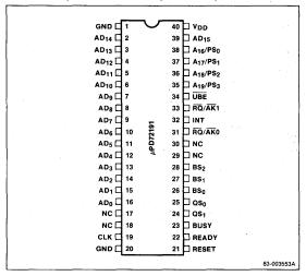
When used in the V40/V50 mode, the  $\mu$ PD72191 will directly generate the control signals for external bus transceivers, memory read/write, and address strobe outputs. In addition, the  $\mu$ PD72191 will select the HLDRQ/HLDAK protocol used by the V40/V50 microprocessors.
