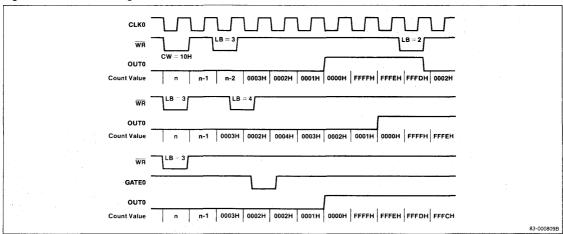
Figure 9. Mode 0 Program Example Timing Chart
