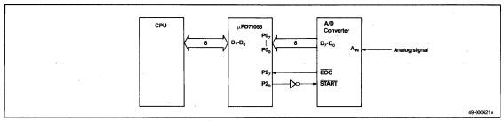
Figure 8. A/D Converter Example
