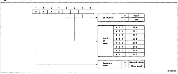
Figure 3. Bit Manipulation Command Example
