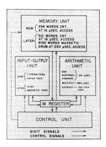
Figure 1. Simplified Block Diagram of the SWAC
