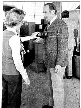
Airports pose a variety of potential threats. In addition to the x-ray devices and walk-through metal detectors, there are handheld metal detectors (here one is purposely being passed over magnetic stripe credit cards in the man's breast pocket) and even radar. The results of NBS tests, in everyday environments and in some nearly inconceivable situations, show that magnetic recording is almost accident proof.
